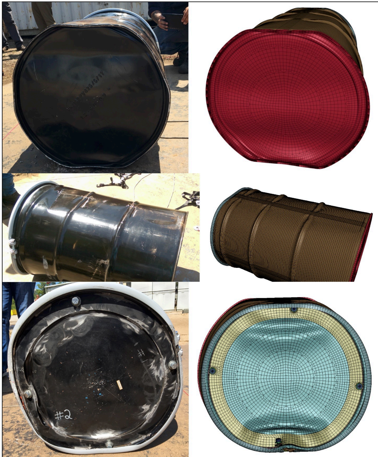
Figure 2-3.3. Side 30-ft Free-Drop/Crush
