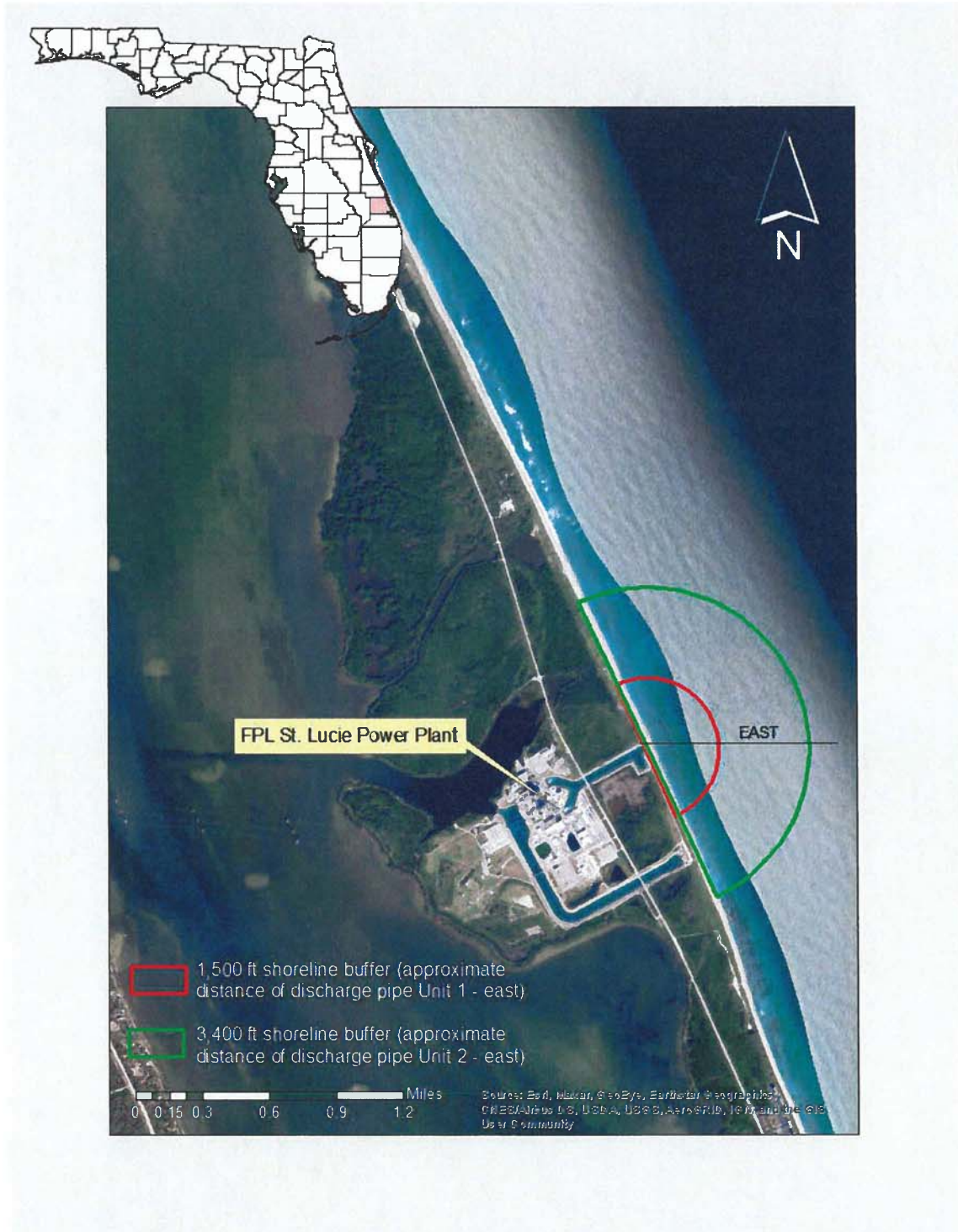
Figure 1. Florida Power & Light Company (FPL)—St. Lucie Nuclear Power Plant (PSL). (Source: https://www.nrc.gov/docs/ML2121/ML21215A319.pdf ) (Note: Red and Green Buffers do not show the area of potential wastewater discharge. Buffers are solely used to show distance from the shoreline. Wastewater discharge is approximately 1,500 to 3,400 feet (approximately 0.3 to 0.6 miles) offshore to the east.)
