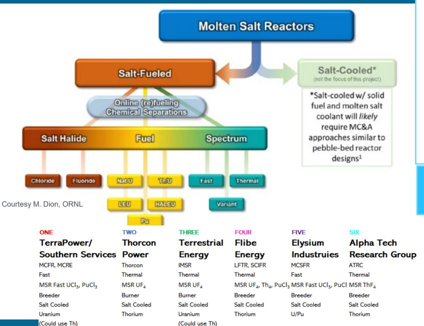
A molten salt reactor (MSR) is any nuclear reactor that employs liquid halide salt to perform a significant function in-core. MSRs include a broad spectrum of design options including:
