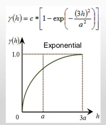
where  $C_0$  is the nugget constant,  $C+C_0$  is the sill, C is the structure variance, and a is the effective range. The slope rate at the point of origin is 3 C/2a, and the intersection between the sill value and x-axis is 2a/3.
