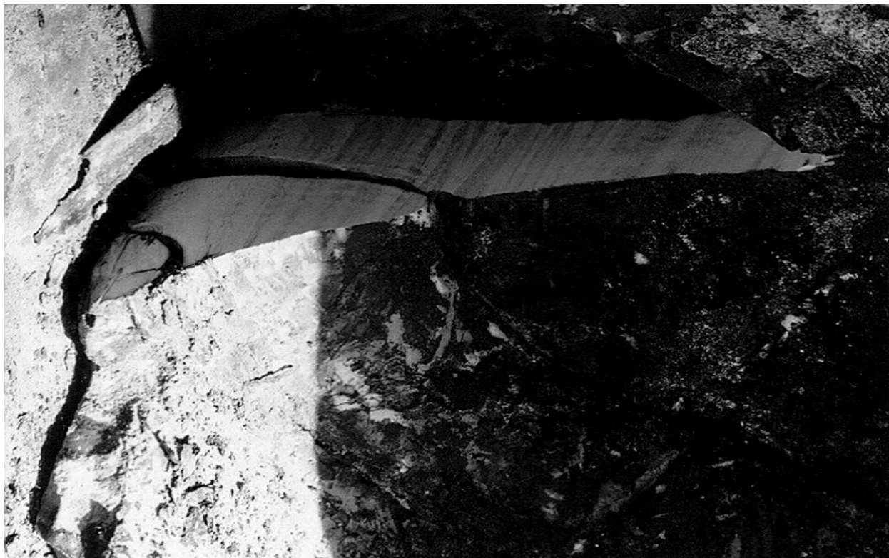
Figure 2.10.3-90 – CTU; Residual Foam in OCA Lid Side; Aligned with Test 1, 2, & 4 Damage
