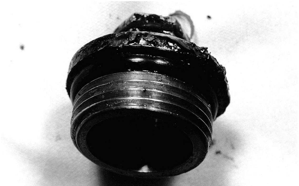
Figure 2.10.3-46 – ETU; View of OCV Vent Port Cover (As Removed; Not Cleaned)
