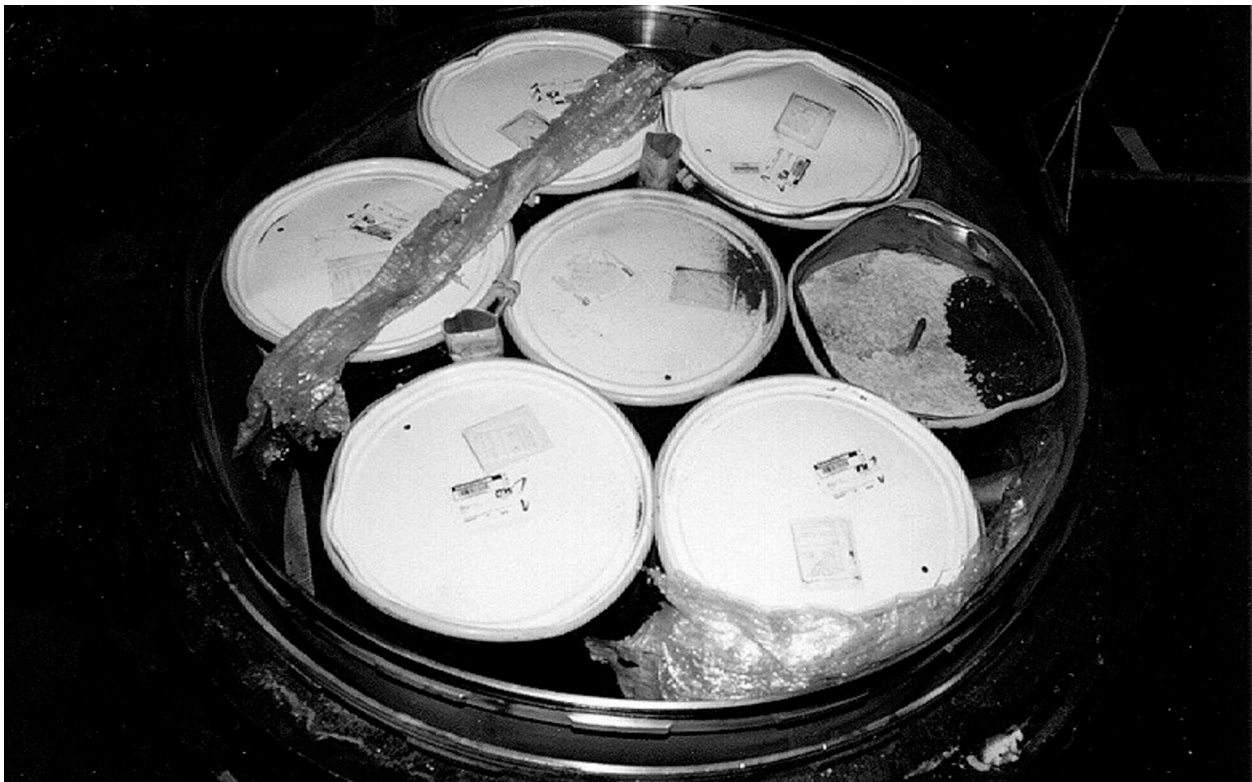
Figure 2.10.3-48 – ETU; View of 55-Gallon Payload Drums Following ICV Lid Removal
