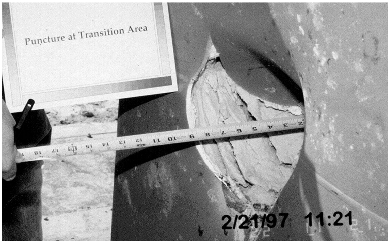
Figure 2.10.3-25 – ETU Puncture Drop Test 7; Radial Penetration ~8" Deep
