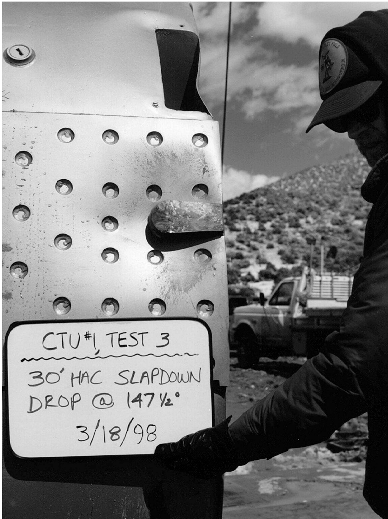
Figure 2.10.3-61 – CTU Free Drop Test 3; Bottom-End Damage
