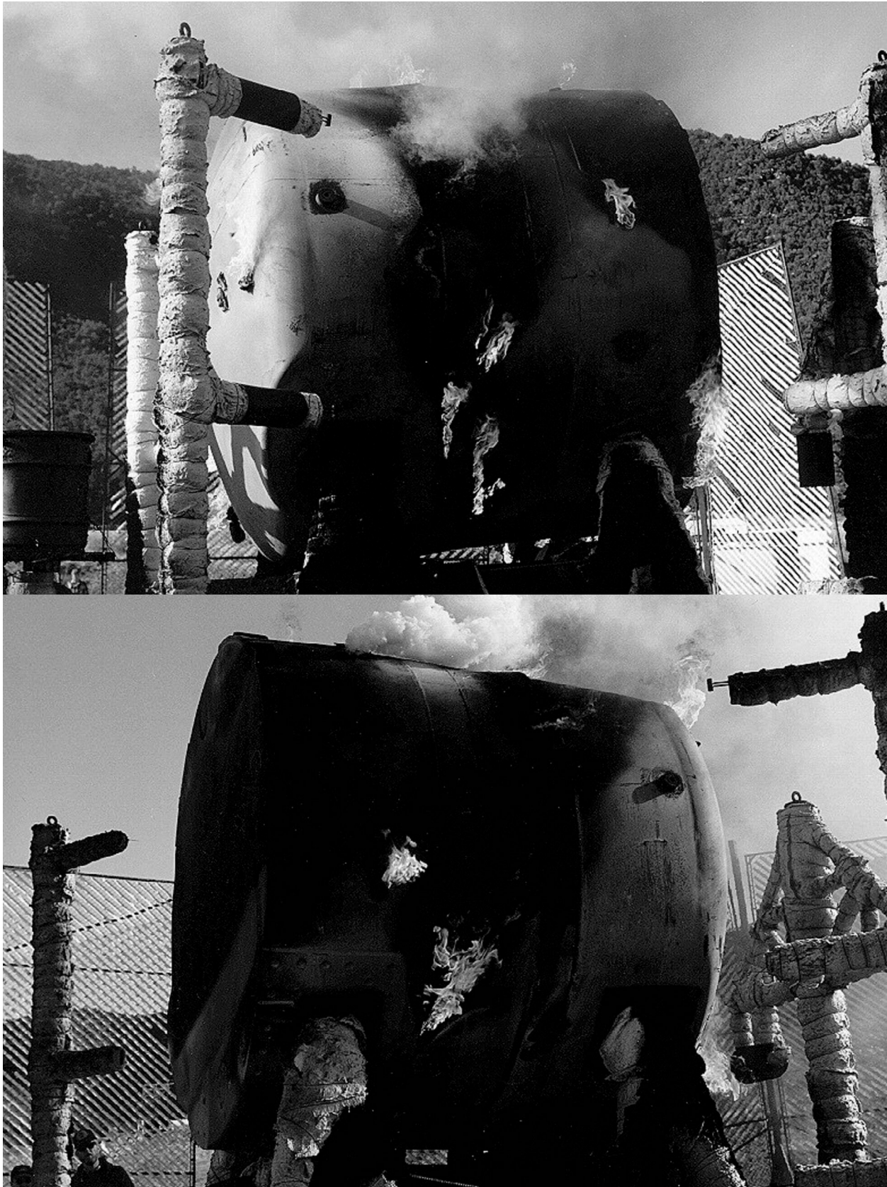
Figure 2.10.3-77 – CTU Fire Test 7; Side 1/2 Views ~10 Minutes after End of Fire
