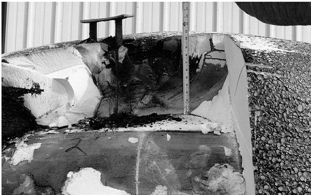
Figure 2.10.3-44 – ETU; Residual Foam in OCA Lid Top (~11")
