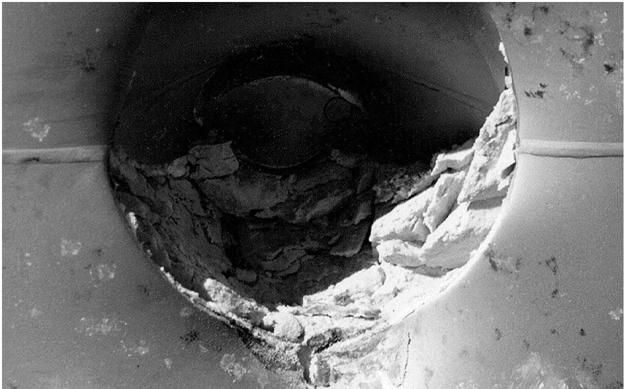
Figure 2.10.3-24 – ETU Puncture Drop Test 7; ~10½" High × ~11½" Wide Hole
