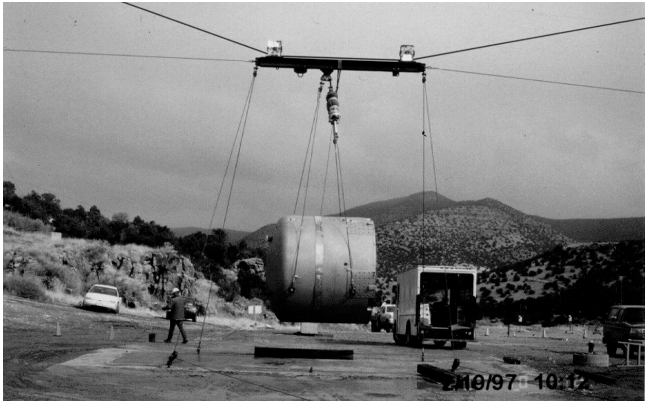
Figure 2.10.3-16 – ETU Free Drop Test 3; View Just Prior to NCT Free Drop Test
