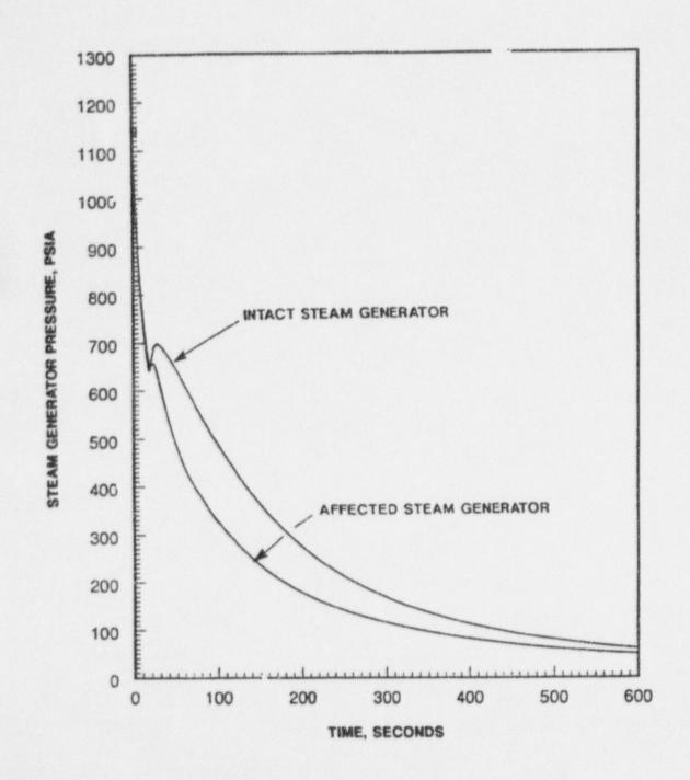
Zero Power Large Steam Line Break with Offsite Power Available; Steam Generator Pressures vs. Time Figure 15.1.5-4.8
