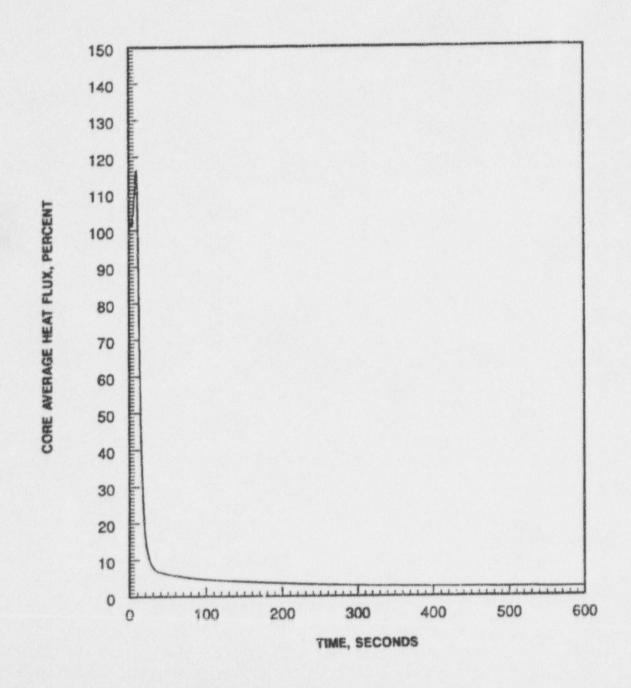
Full Power Large Steam Line Break with Offsite Power Available; Core Average Heat Flux vs. Time
