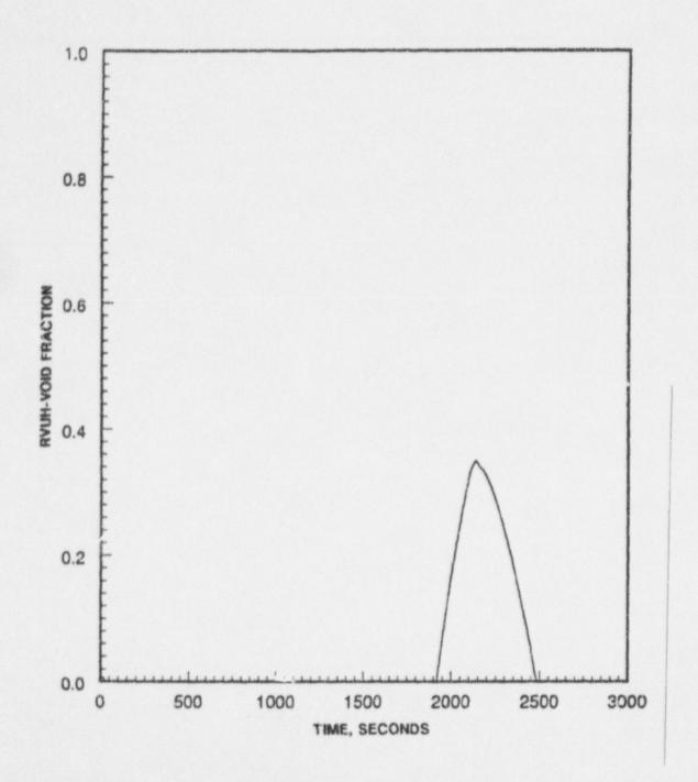
Inadvertent Opening of an Atmospheric Dump Valve (IOSGADV) with Loss of Offsite Power; Reactor Vessel Upper Head Steam Void Fraction
