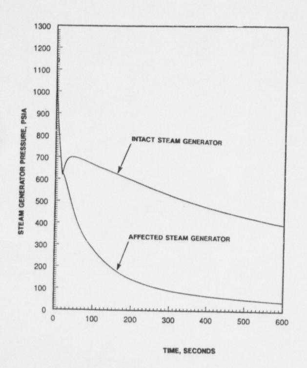
Zero Power Large Steam Line Break with Concurrent Loss of Offsite
