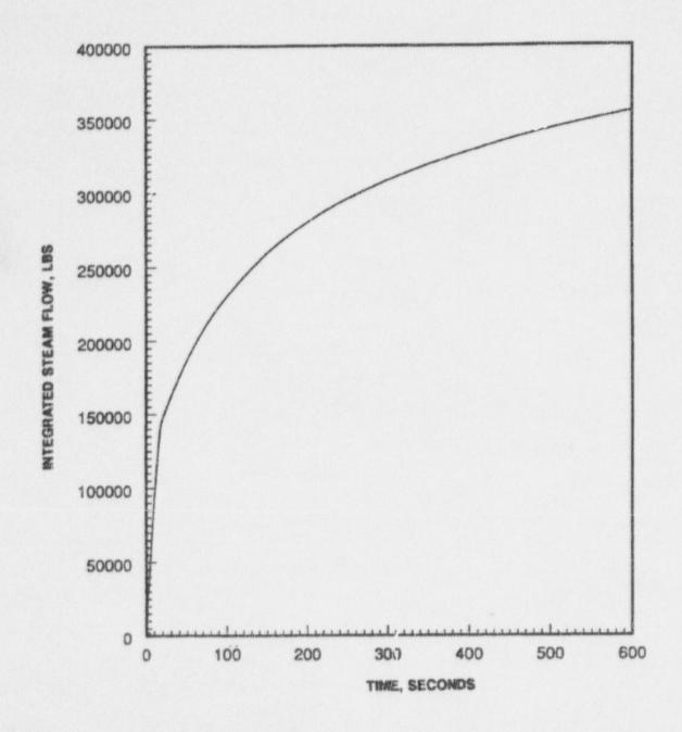
Zero Power Large Steam Line Break with Concurrent Loss of Offsite Power; Integrated Steam Flow Thru Break vs. Time Figure 15.1.5-3.11
