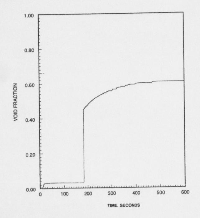
Full Power Large Steam Line Break with Concurrent Loss of Offsite Power; Reactor Vessel Upper Head Steam Void Fraction vs. Time
