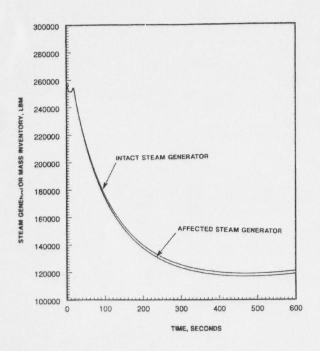
Full Power Large Steam Line Break with Offsite Power Available; Steam Generator Mass Inventories vs. Time Figure 15.1.5-2.10
