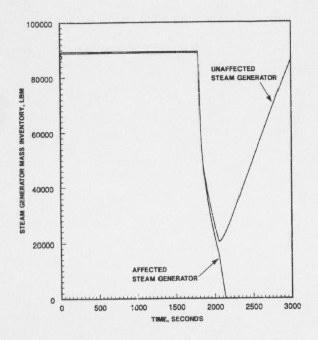
Inadvertent Opening of an Atmospheric Dump Valve (IOSGADV) with Loss of Offsite Power; Steam Generator Mass Inventories vs. Time
