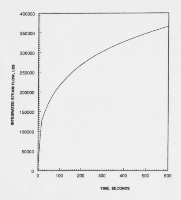
Full Power Large Steam Line Break with Concurrent Loss of Offsite Power; Integrated Steam Mass Release Through Break vs. Time Figure 15.1.5-1.11
