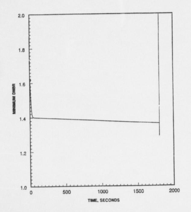
IOSGADV with Single Failure and LOOP; Minimum DNBR vs Time
