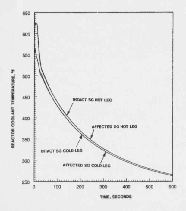
Full Power Large Steam Line Break with Offsite Power Available; Reactor Coolant Temperatures (B) vs. Time Figure 15.1.5-2.5B
