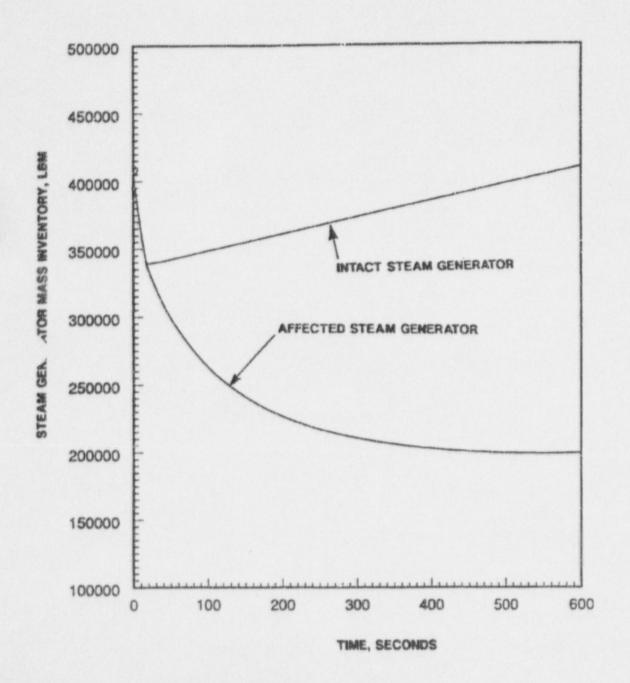
Zero Power Large Steam Line Break with Concurrent Loss of Offsite Power; Steam Generator Mass Inventories vs. Time Figure 15.1.5-3.10
