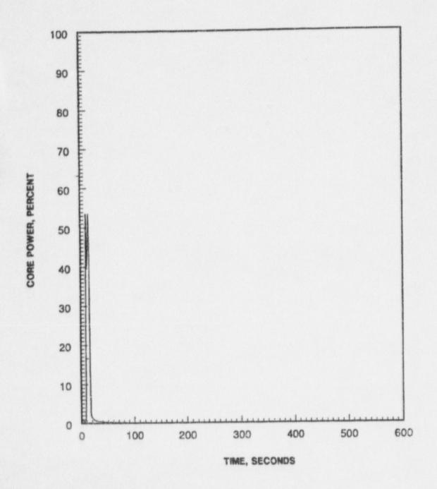
Zero Power Large Steam Line Break with Offsite Power Available; Core Power vs. Time
