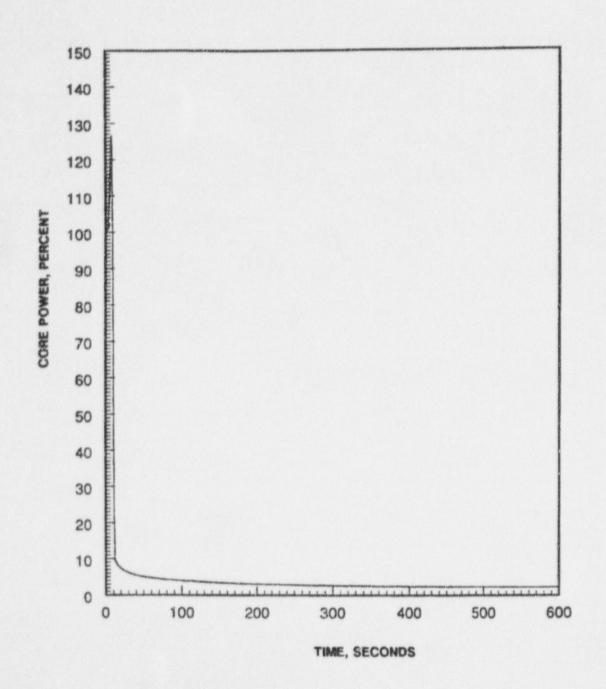
Full Power Steam Line Break with Loss of Offsite Power; Core Power vs. Time
