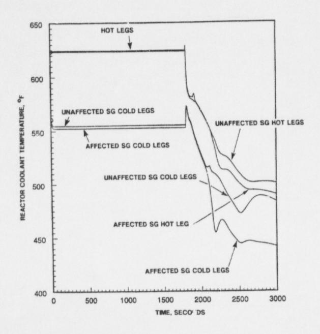
Inadvertent Opening of an Atmospheric Dump Valve (IOSGADV) with Loss of Offsite Power; Reactor Coolant Temperatures (B) vs. Time
