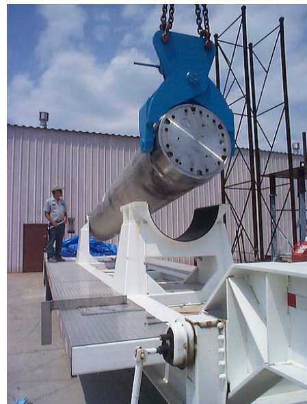
Figure 5. TN-FSV Legal Weight Truck Transport Cask (Greene et al. 2013).
