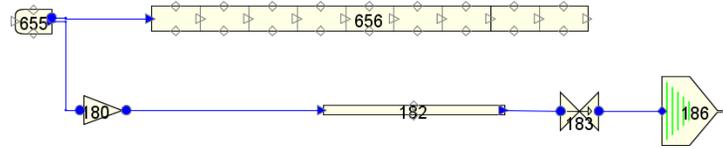
**Figure 3-2 RELAP5 Nodalization of Break Flow in Cold Leg 1**
