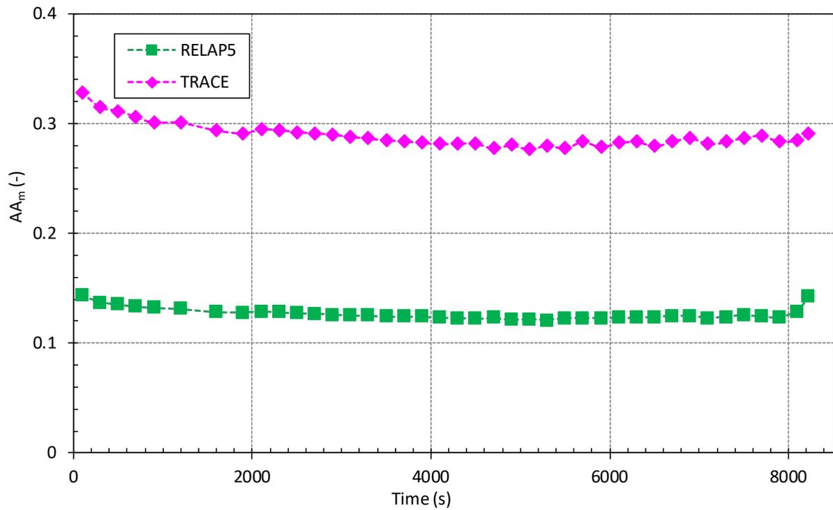
Figure 5-16 Core (Electrical) Power (W+02): a) Visual Observation (Top), b) Accuracy Measure  $AA_m$  (Bottom)
