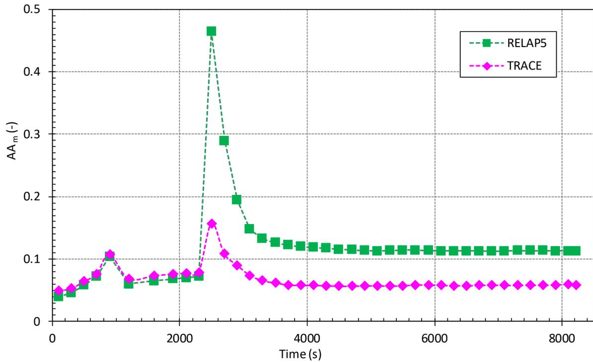
Figure 5-2 SG1 Steam Dome Pressure (P+47): a) Visual Observation (Top), b) Accuracy Measure  $AA_m$  (Bottom)
