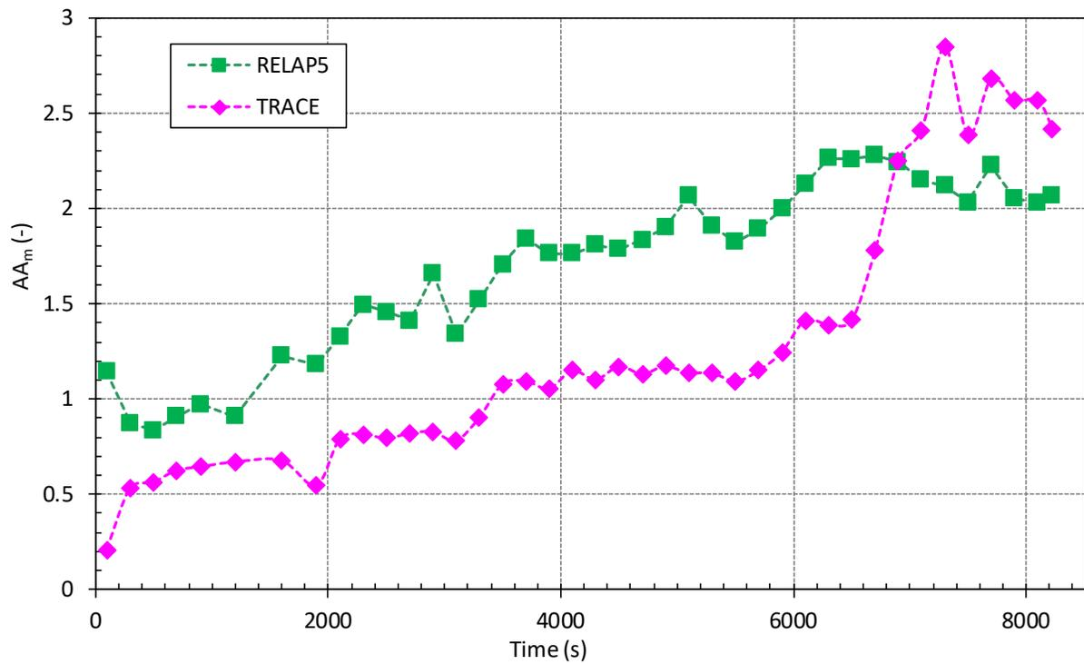
**Figure 5-18 Loop Seal 1 Upflow Side Differential Pressure (DP12VP): a) Visual Observation (Top), b) Accuracy Measure  $AA_m$  (Bottom)**
