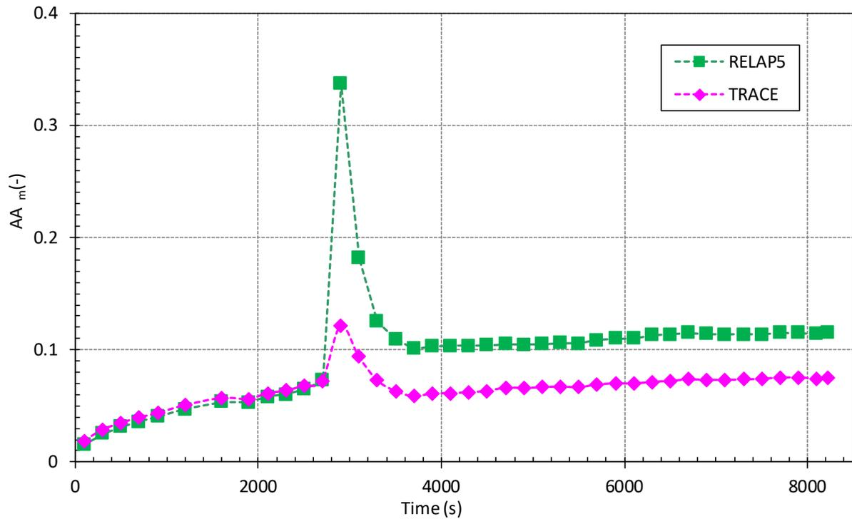
Figure 5-3 Accumulator 2 Gas Phase Pressure (P+SM2): a) Visual Observation (Top), b) Accuracy Measure AA<sub>m</sub> (Bottom)
