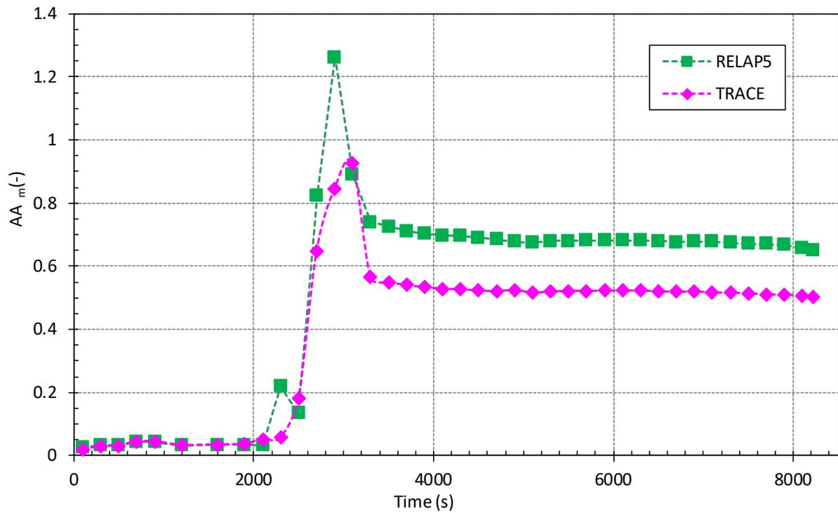
Figure 5-12 Rod Temperature (Top) (TS0228L): a) Visual Observation (Top), b) Accuracy Measure AA<sub>m</sub> (Bottom)
