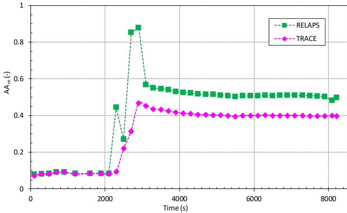
Figure 5-11 Rod Temperature (Middle) (TS0215L): a) Visual Observation (Top), b) Accuracy Measure AA<sub>m</sub> (Bottom)
