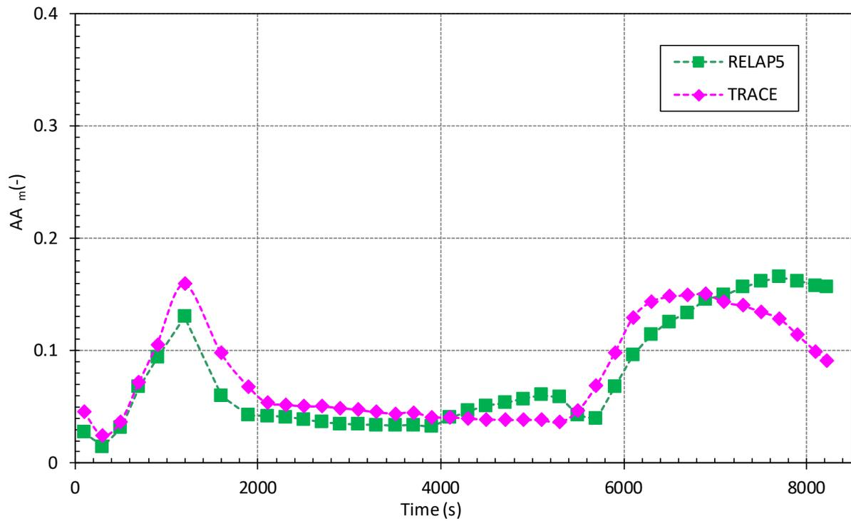
**Figure 5-9 Time Integrated Break Mass Flow (INTQMB): a) Visual Observation (Top), b) Accuracy Measure AA<sub>m</sub> (Bottom)**
