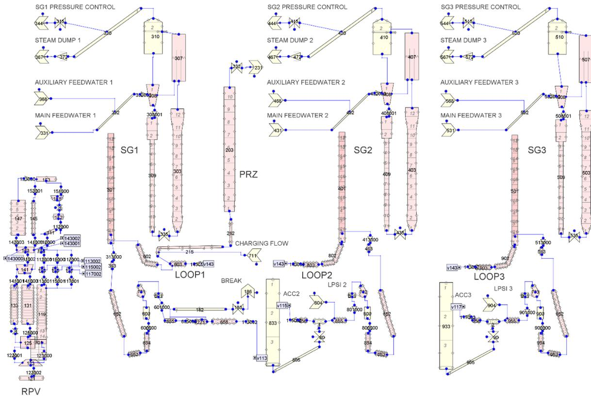
**Figure 3-3 TRACE Hydraulic Components View of BETHSY Facility**
