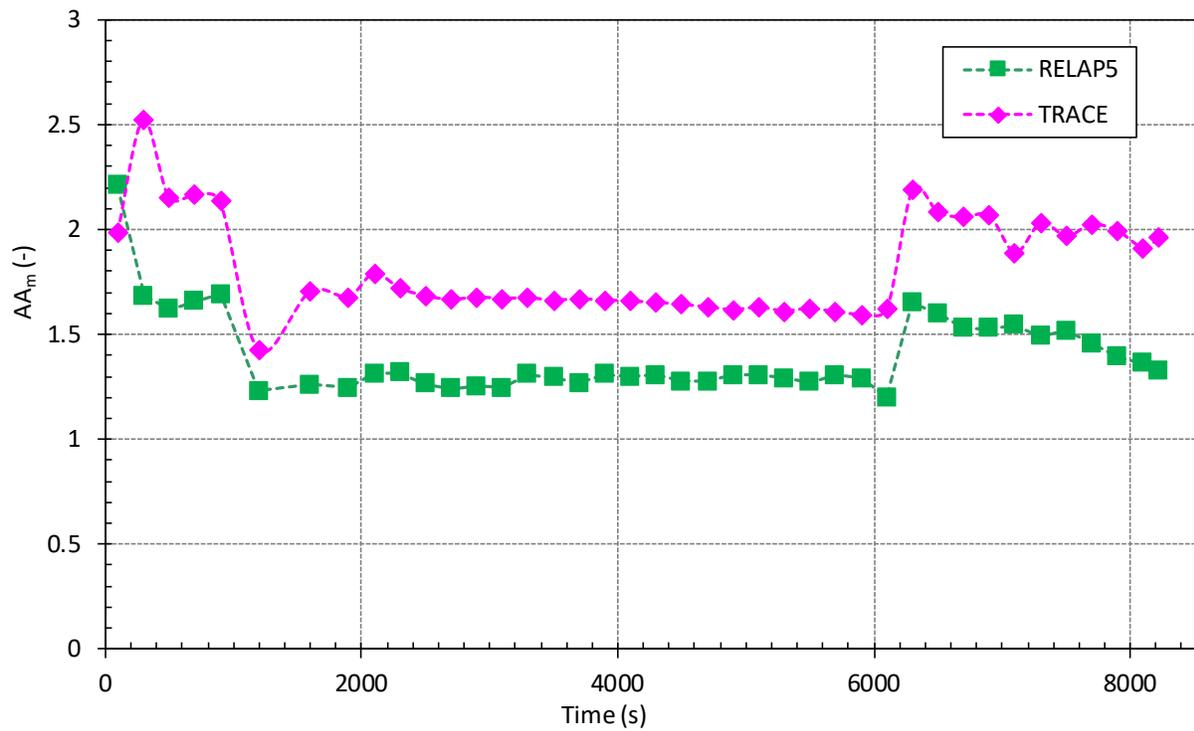
Figure 5-21 Downcommer to Upper Head Differential Pressure (DP050): a) Visual Observation (Top), b) Accuracy Measure AA<sub>m</sub> (Bottom)
