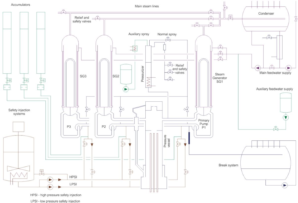
**Figure 2-1 BETHSY Schematic Diagram**
