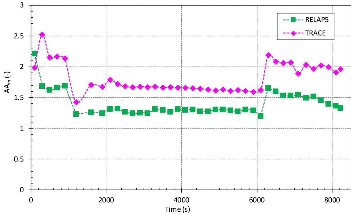
Figure 5-20 SG1 Inlet Plenum Differential Pressure (DP41): a) Visual Observation (Top), b) Accuracy Measure  $AA_m$  (Bottom)
