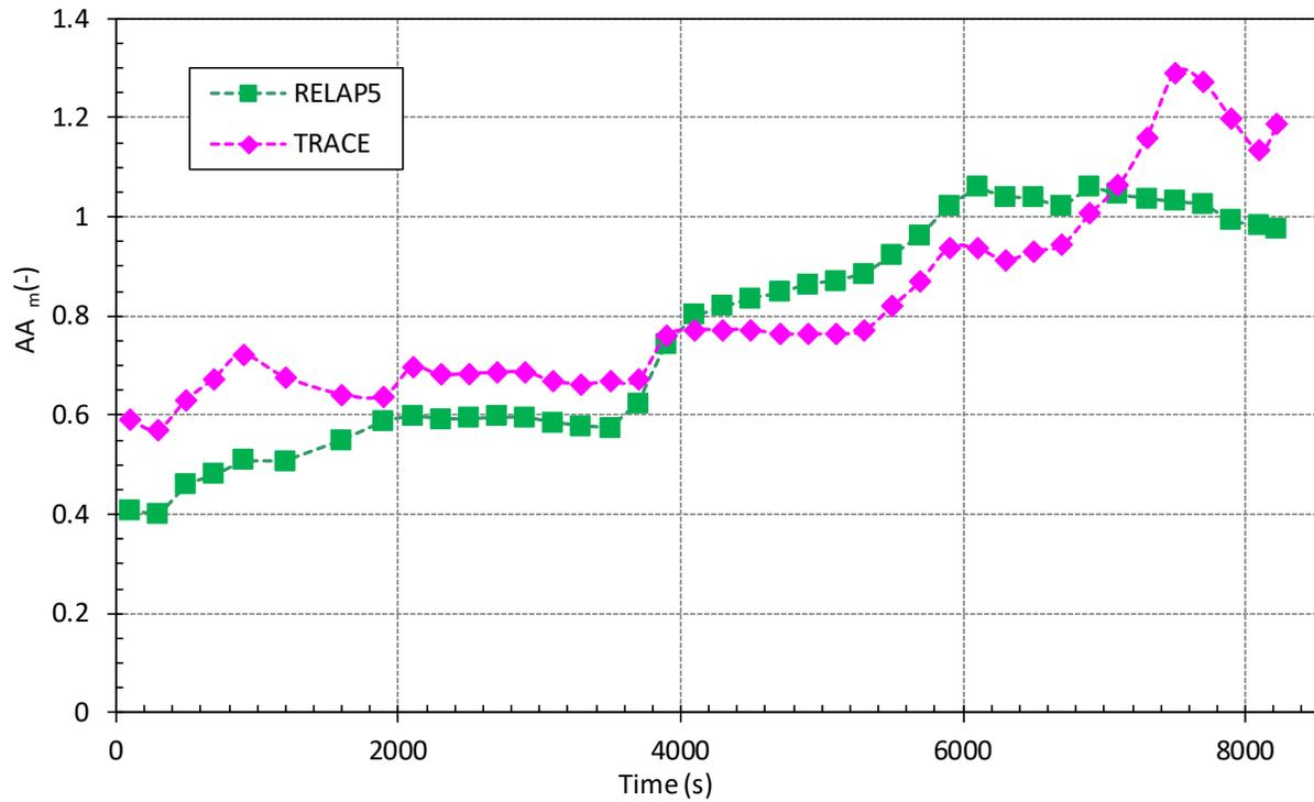
Figure 5-8 Break Mass Flow Rate (QMB): a) Visual Observation (Top), b) Accuracy Measure  $AA_m$  (Bottom)
