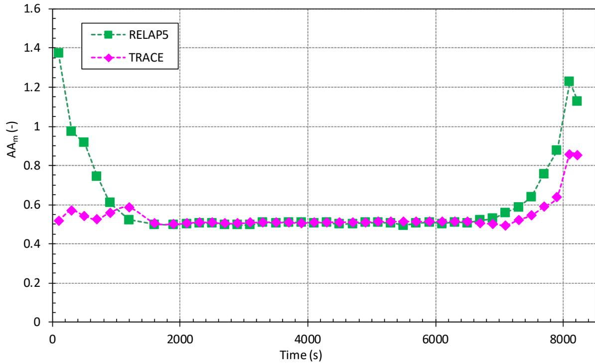
**Figure 5-14 SG1 U-Tube Upflow Side Differential Pressure (DP426): a) Visual Observation (Top), b) Accuracy Measure  $AA_m$  (Bottom)**
