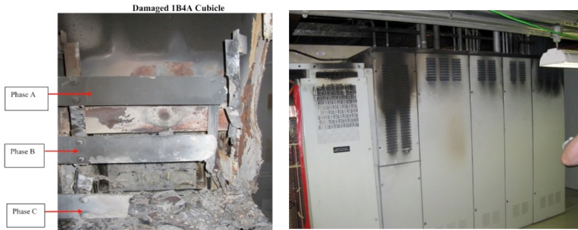
Figure 4-9 Backside of initiating breaker (left) showing damaged bus bars and backside of low-voltage switchgear (right) showing smoke stains and discolored paint behind arc location (brown stain at the mid-height of the middle section) [34]
