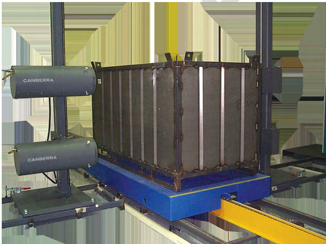
Figure J-7 WM2500—Modular Gamma Box and Container Counter
