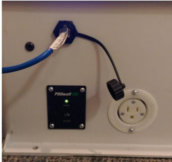
Figure 2 Interface box power button, Ethernet port and AC power outlet
