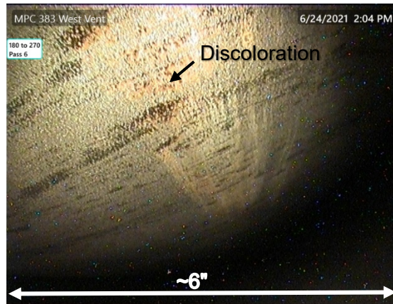
116. Rust colored discoloration on MPC
