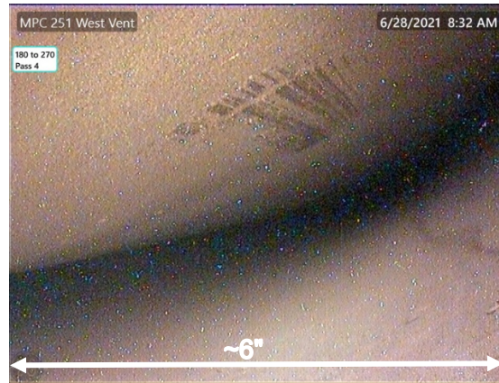
72. Superficial scrape mark on MPC
