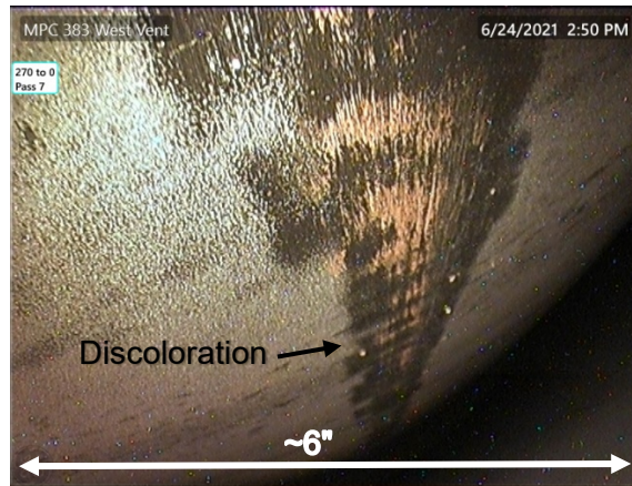
123a. Closeup of rust spots / discoloration on MPC (photo 123)
