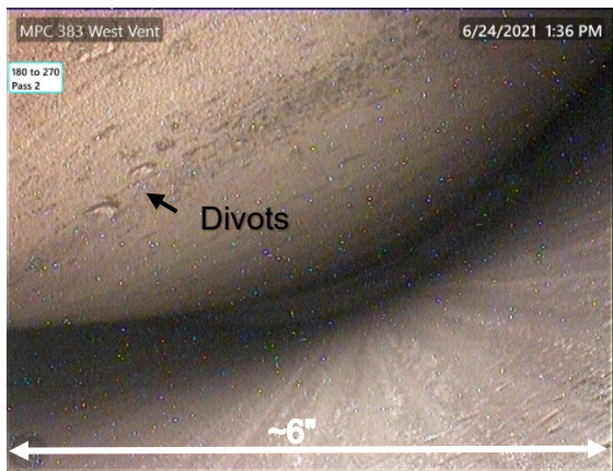
111. Divots on MPC, shallow, no observable depth
