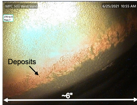
168. Rust colored deposits near lower weld of MPC
