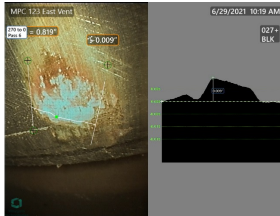
4a. Rust spot (photo 4) measurement, buildup of 0.009" 5
