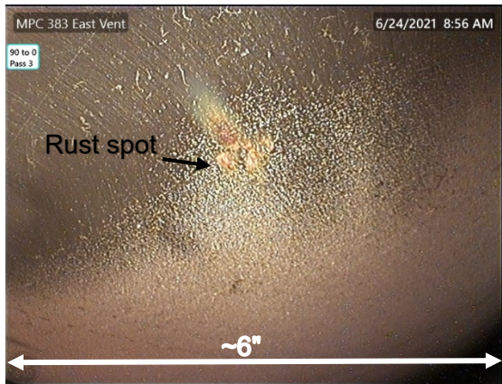
82. Rust spot on MPC, not 3-D
