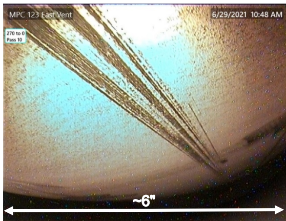
9. Superficial scratches on MPC
