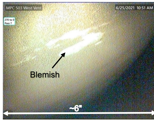
166. Blemish on MPC, no observable depth
