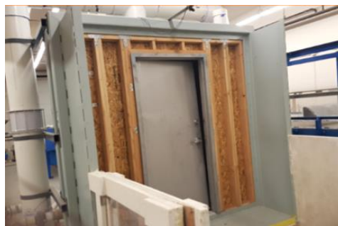
Figure 5-10 ISU Flood Testing Facility PET tank - Front side, with Modular Wall and Inserted Door Barrier [34]
