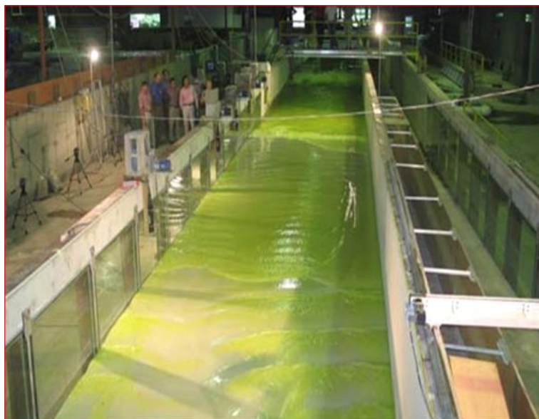
Figure 5-23 USACE ERDC CHL 10-ft Wave Flume [54]
