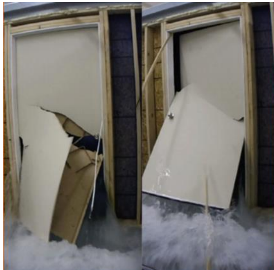
Figure 5-16 Flood Testing of a Hollow Door Barrier at ISU flood Testing Facility [34]
