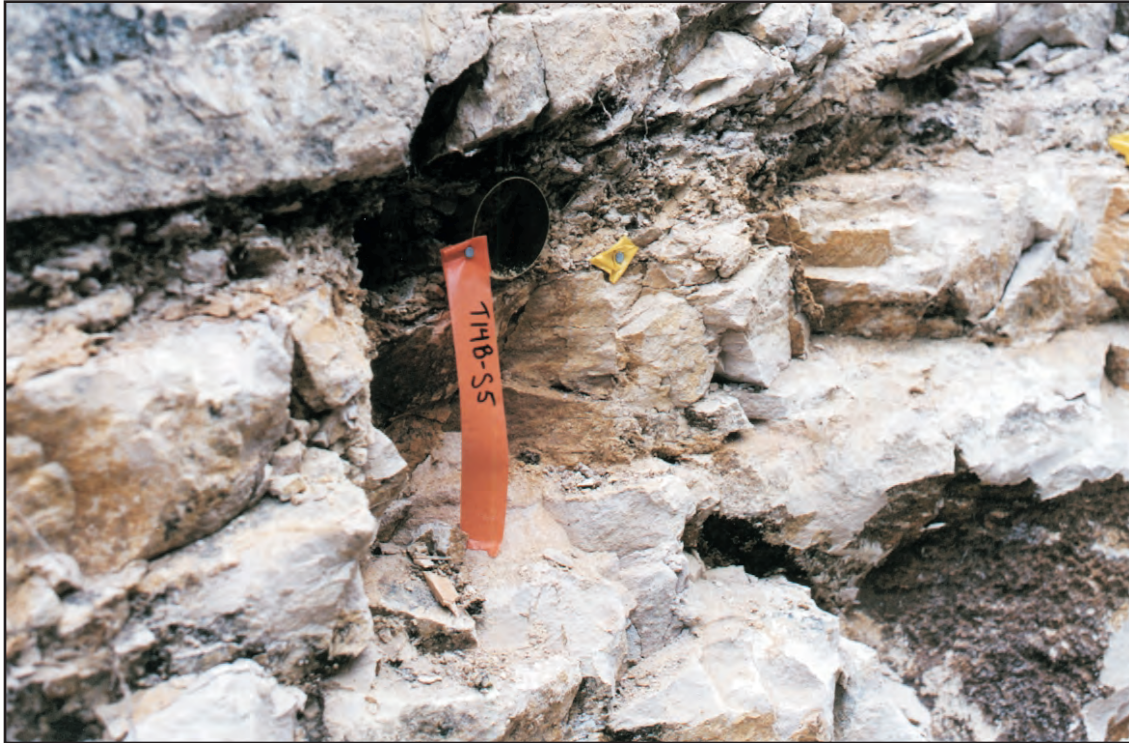
Clay bed within dolomite (Tof b-1 ) with sample tube in trench T-14B. Photo roll JLB-8.
