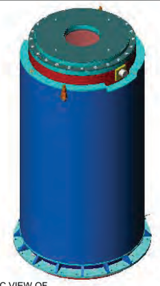
ISOMETRIC VIEW OF HI-TRAC 125D TRANSFER CASK
