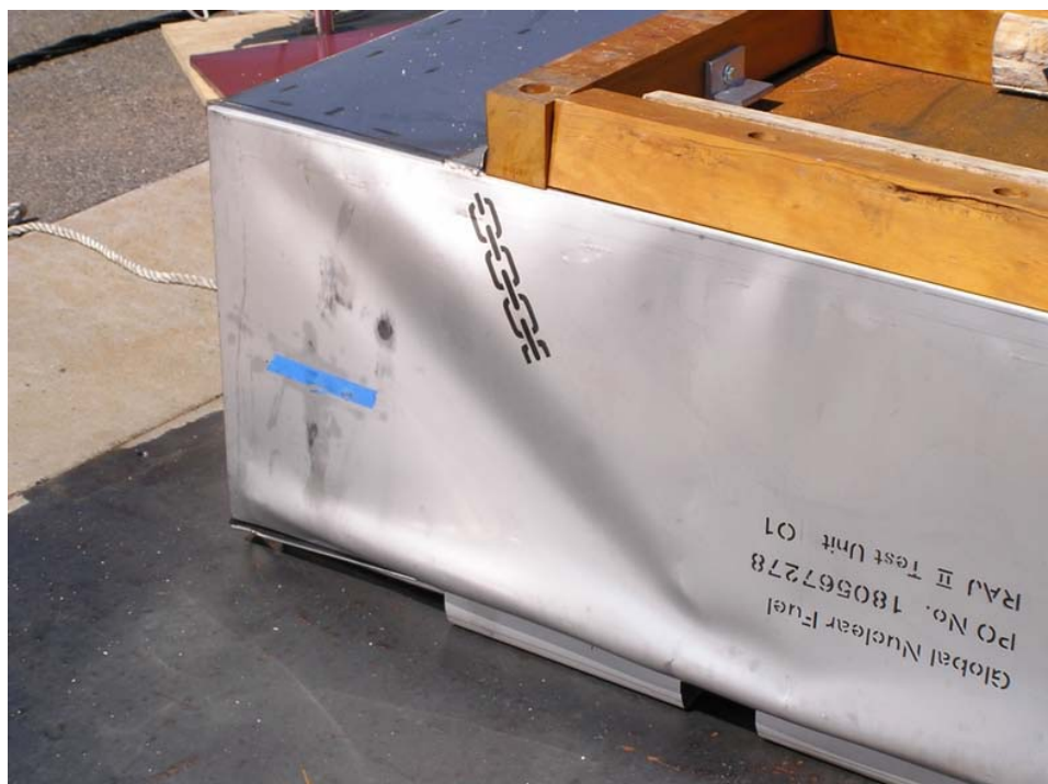
Figure 2-30 Secondary Impact End Damage
