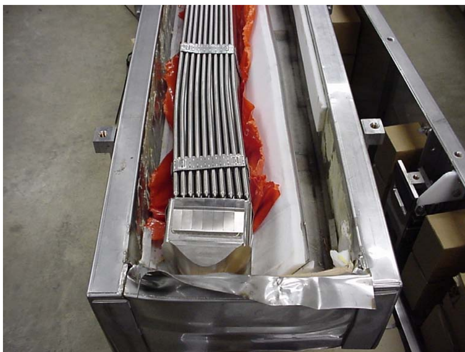
Figure 2-40 Internal Damage to CTU 2
