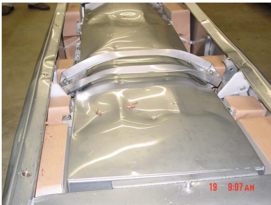
Figure 2-36 Damage Inside Outer Container to CTU 1
