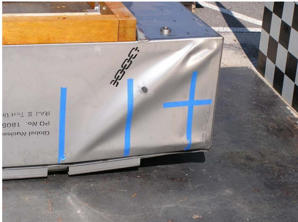
Figure 2-29 Primary Impact End Slap-down Damage
