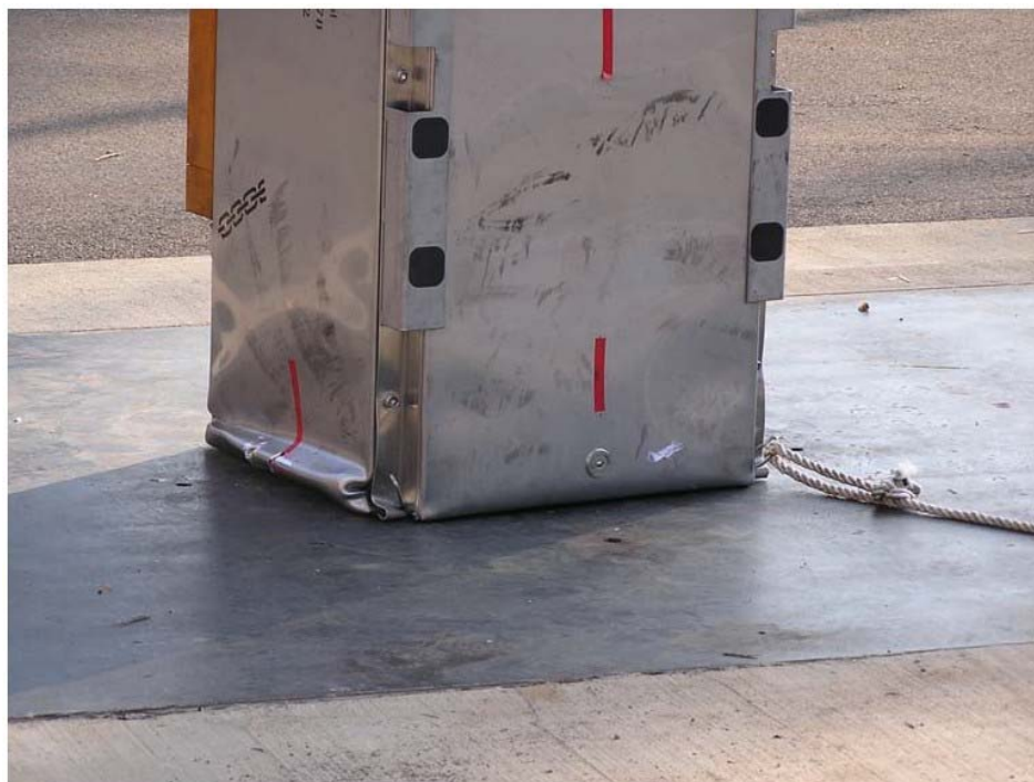
Figure 2-35 End Impact Damage (Top and Side)
