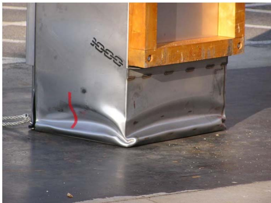
Figure 2-34 Damage from End Impact (Bottom and Side)
