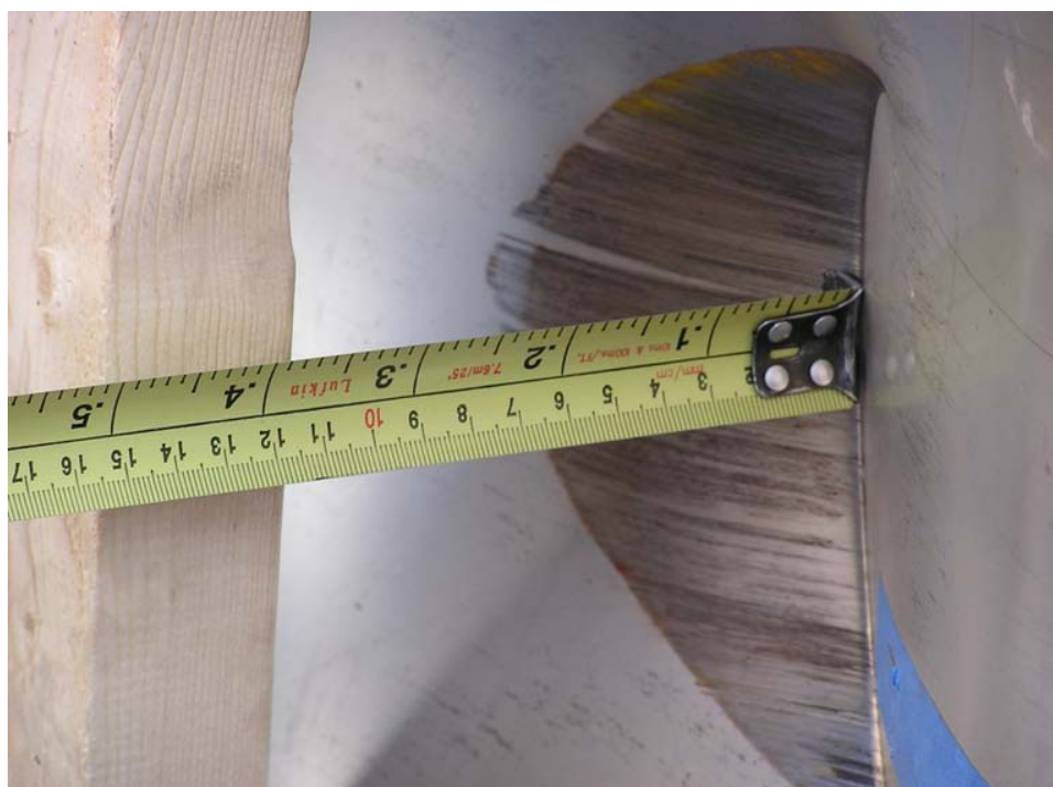
Figure 2-32 Close Up of Puncture Damage
