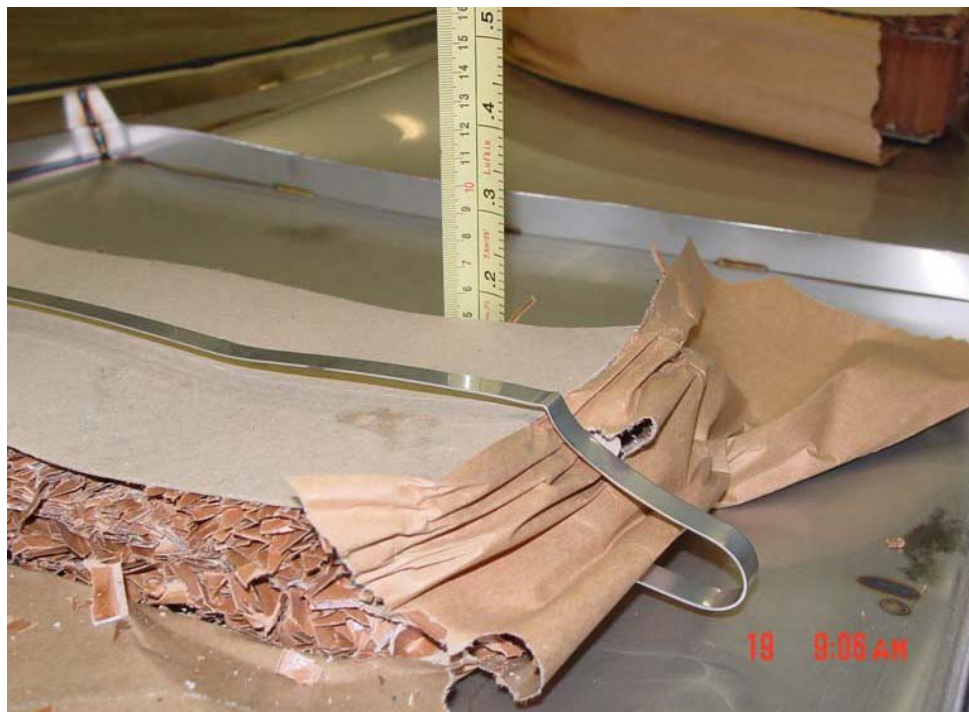
Figure 2-38 Lid Crush on CTU 1
