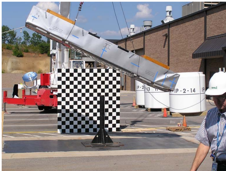
Figure 2-27 Position for Puncture Test
