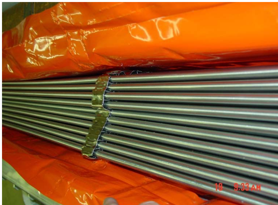
Figure 2-39 Damage to Fuel in CTU 1
