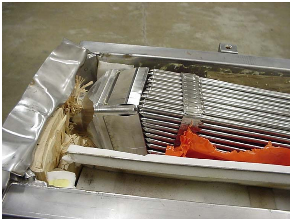
Figure 2-41 Fuel Damage CTU 2
