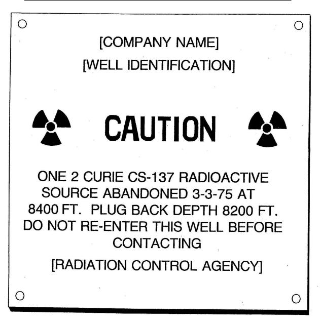
The size of the plaque should be convenient for use on active or inactive wells, e.g., a 7-inch square, <sup>1</sup>/<sub>8</sub><sup>th</sup> inch thick. Letter size of the word "CAUTION" should be approximately twice the letter size of the rest of the information, e.g., 1/2-inch and 1/4-inch letter size, respectively.
