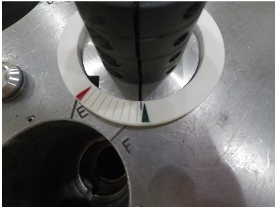
Figure 2. Fuel element latched in position H-7 (note: in this prototype the fully latched green triangle is about 2^\circ off of the actual fully latched position. This will be corrected in future prototype and design development.)
