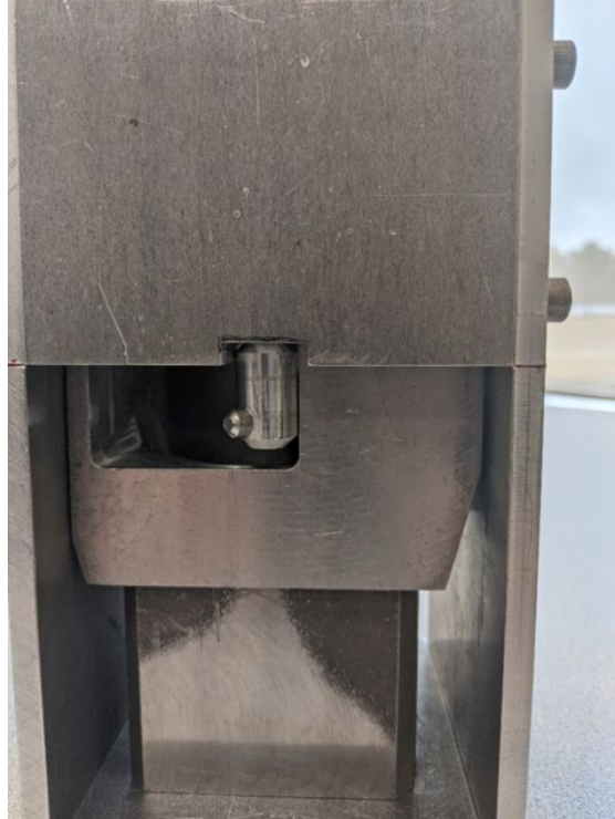
Figure 1. Fuel element head latched into a mockup of the upper grid plate.
