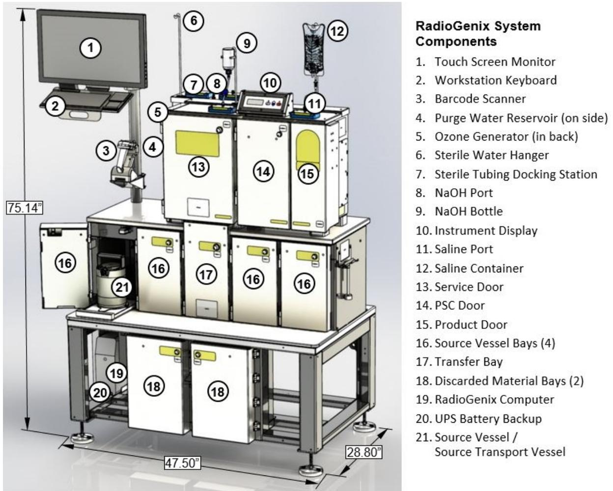
Figure 1. The NorthStar RadioGenix® Mo-99/Tc-99m Generator System Model 1.2<sup>1</sup> with enhanced shielding and with the major components labeled. Component 20, the source vessel (on the left and inside the first of the four components numbered 15), is approximately the same size as a conventional generator containing fission-produced Mo-99. The generator system with enhanced shielding weighs 4,100 pounds and is approximately 48 inches wide, 29 inches deep, and 75 inches tall.
