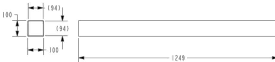
Fig. 0 Dimensions of rectangular pipe Tolerances on all dimensions shall
