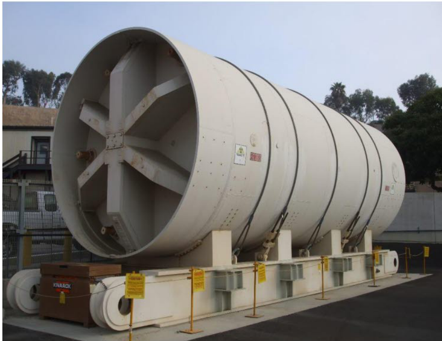
Unit 1 RPV and associated skid prior to modification
