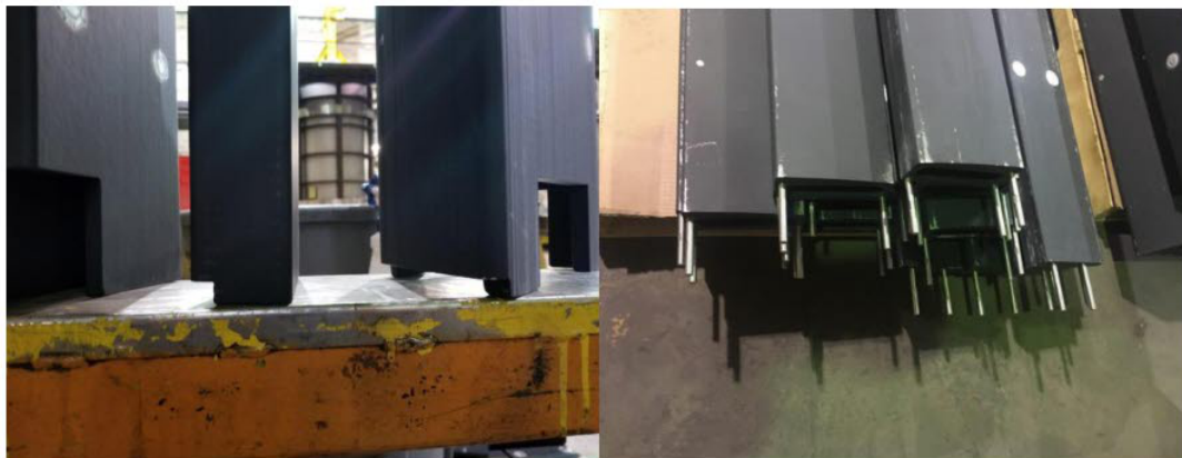
Original design: machined slots (left) and new design: stand off pins (right)
