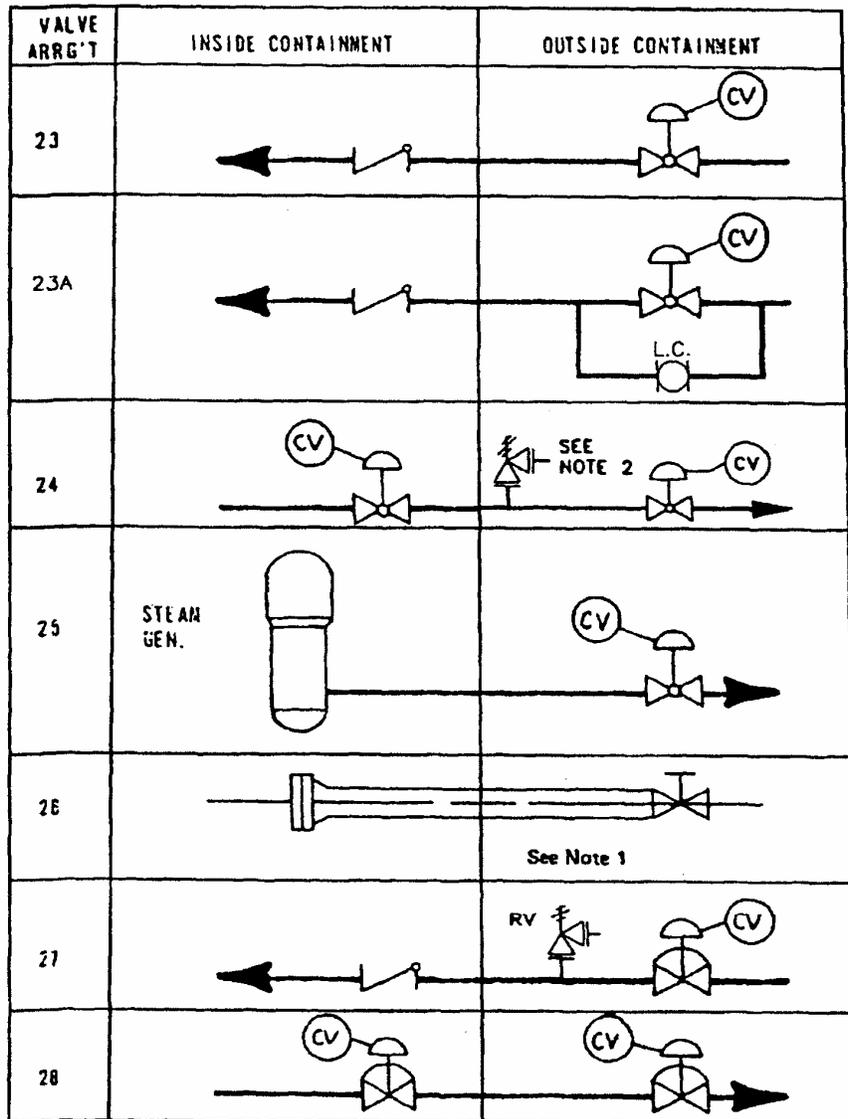
Note 1: Containment isolation is provided by the blind flange inside containment. Valve outside containment for arrangement 26 is shown for completeness only and is not a containment isolation valve.
