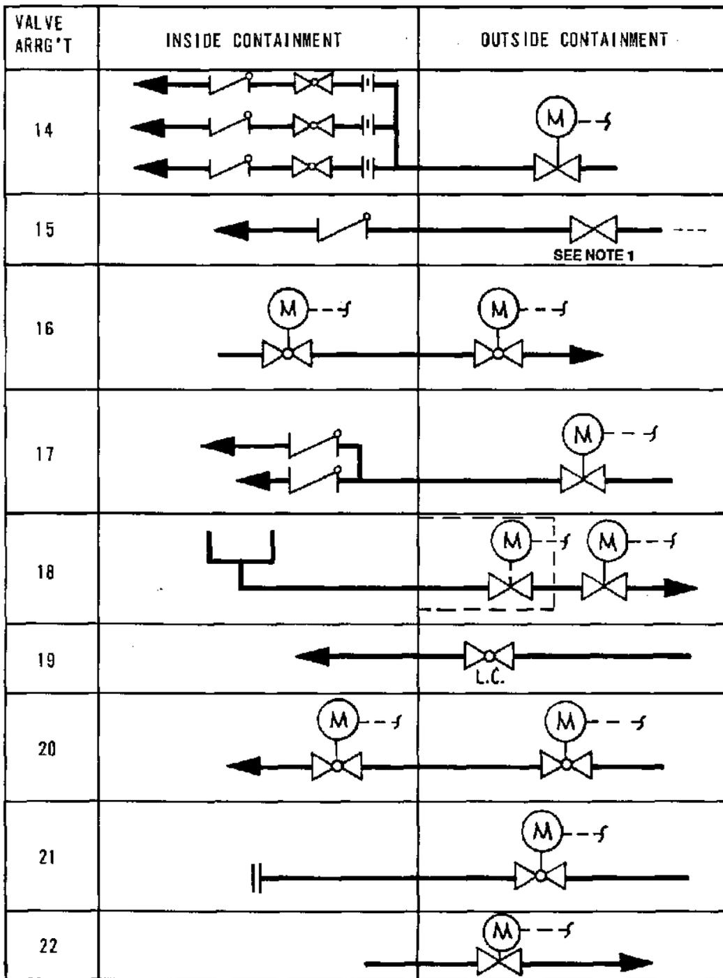
Note 1: Containment Isolation Protection Is Provided By The High Pressure Seal Water In-Flow And The Check Valve Inside Containment. The Valve Outside Containment For Arrangement 15 Is Shown For Completeness Only And Is Not A Containment Isolation Valve.
