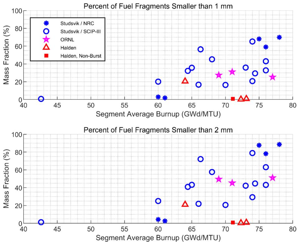
Figure A-2. Mass fraction of fuel fragments smaller than 1 mm<sup>10</sup> and 2 mm (Wiesenack, 2013; Wiesenack, 2015; NRC, 2013; Capps, et al., 2020; Magnusson, 2017; Magnusson and Sheng, 2017; Magnusson, 2018; Magnusson, et al., 2020; Mileshina and Magnusson, 2019a, b, c, d, e; Mileshina et al., 2019; König, 2021a, b, c).
