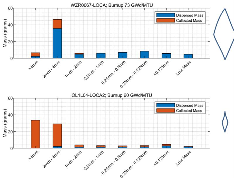
Figure A-4. Fragment size distribution for SCIP III test at 60 and 73 GWd/MTU, with relative burst opening size (Mileshina and Magnusson, 2019b, c).
