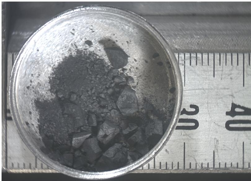
Figure 5. Fuel fragments collected from the top end of rod 192 after gentle shaking and just before gamma scan (NRC, 2013).
