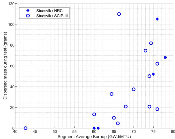
Figure A-1. Mass of fuel dispersed during the LOCA experiment as a function of burnup (NRC, 2013; Magnusson, 2017; Magnusson and Sheng, 2017; Magnusson, 2018; Magnusson, et al., 2020; Mileshina and Magnusson, 2019a, b, c, d, e; Mileshina et al., 2019; König, 2021a, b, c).
