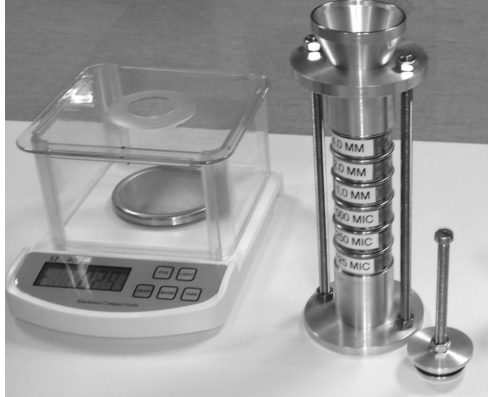
Figure 1 A sieve stack apparatus is used to examine fuel fragment size distribution in the programs referenced in this RIL. The image is of Halden's sieving apparatus used in the IFA-650 experiments (Wiesenack, 2015).
