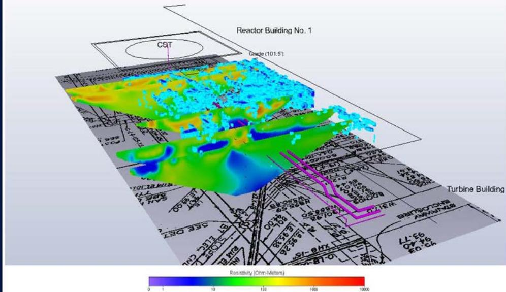
Modeled Earth Resistivity and Ground Penetrating Radar Survey to Support Buried Pipe Encasement Evaluation - DRAFT
