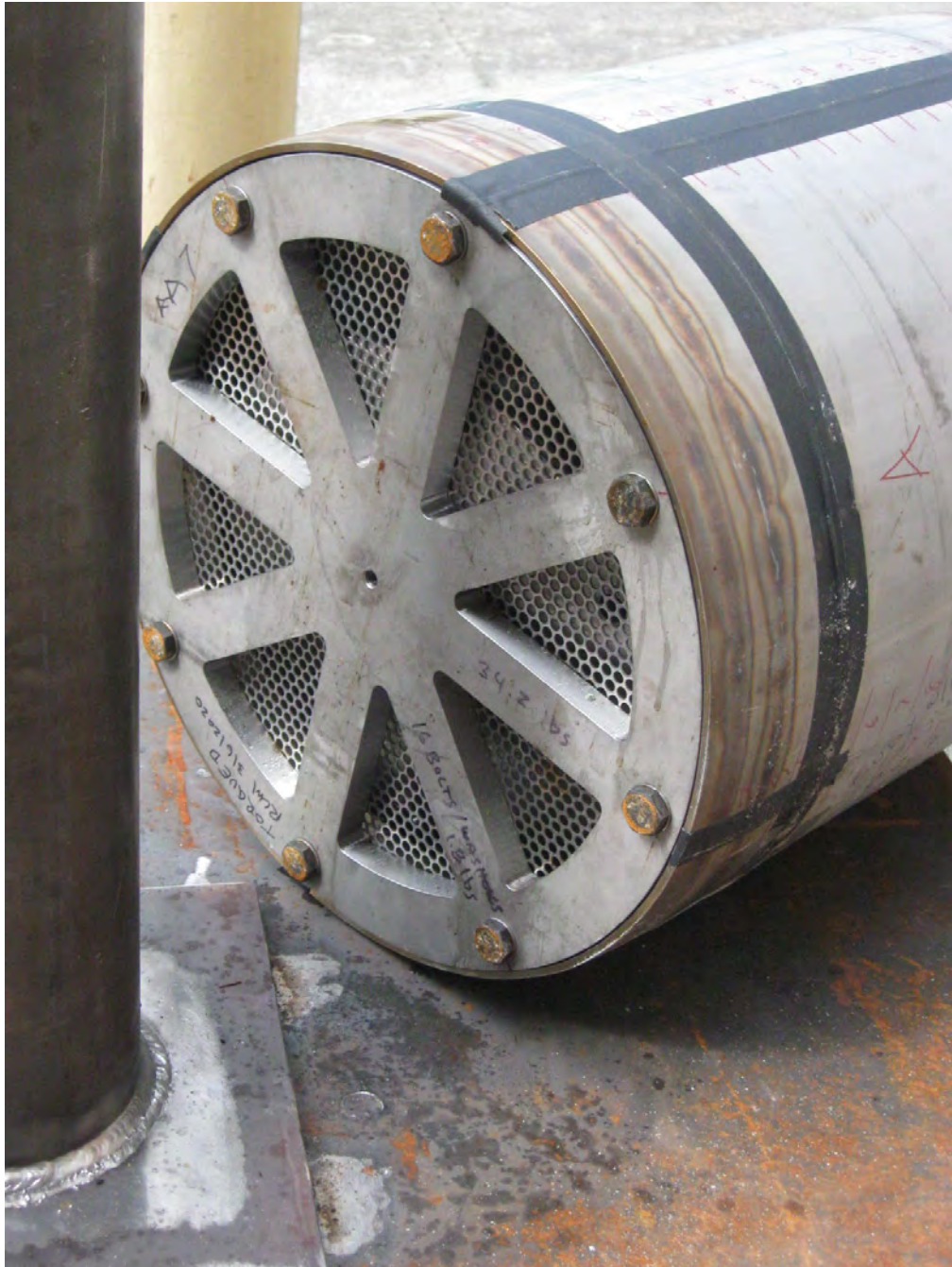
FIGURE B.1.5-2 – Close-up View of Closure Lid After Puncture Drop
