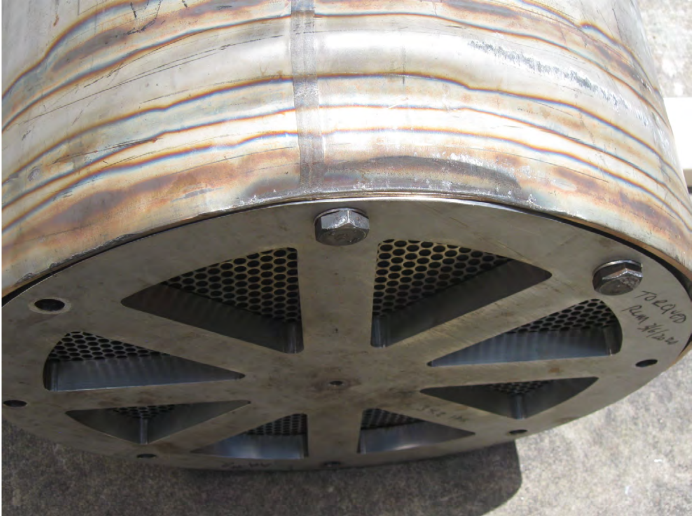
FIGURE B.1.7-2 – Close-up View of Top Corner After Puncture Drop
