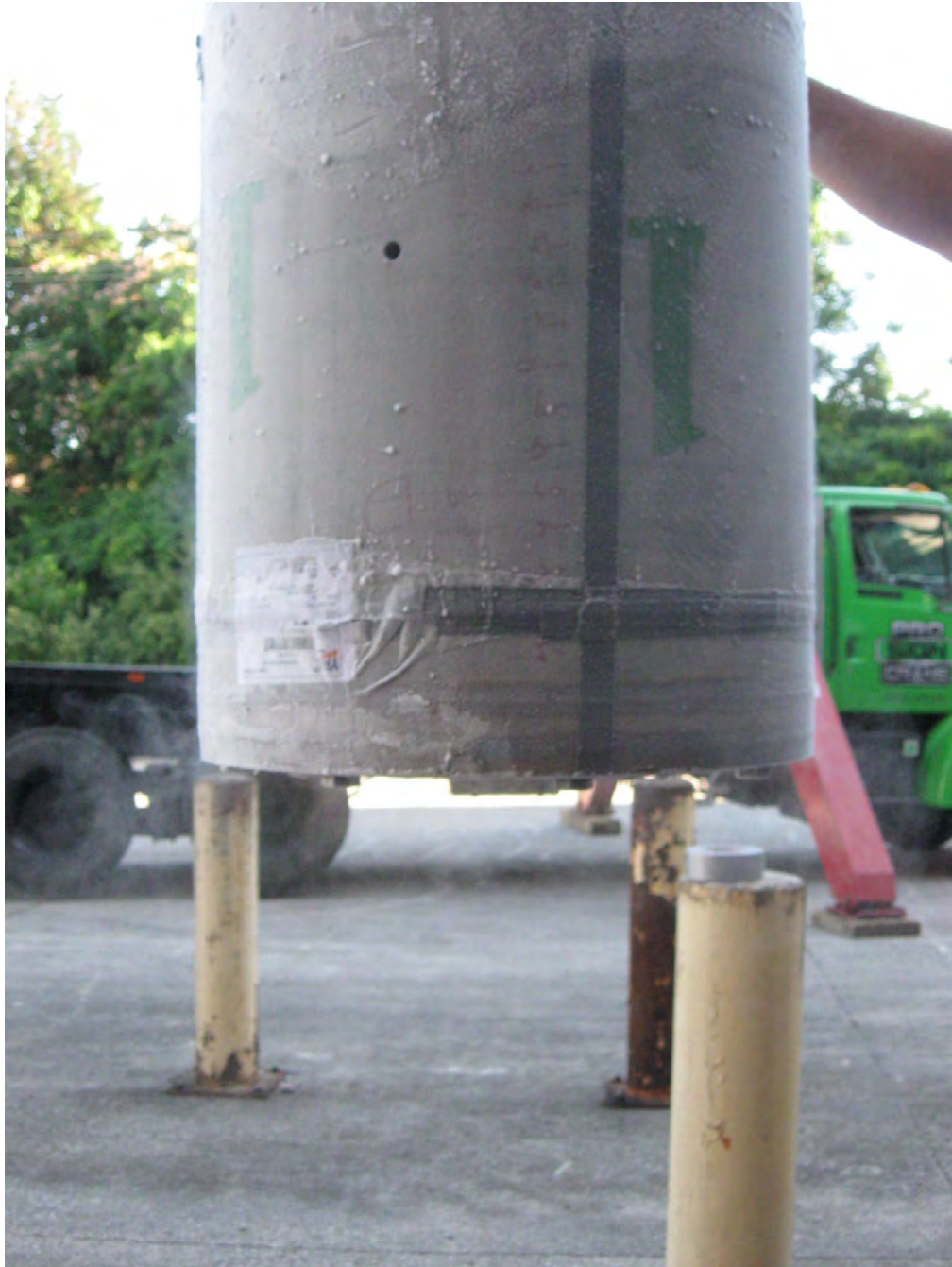
FIGURE B.1.1-3 – Close-up View of Top/Side Following NCT 4-Foot Top Down Drop
