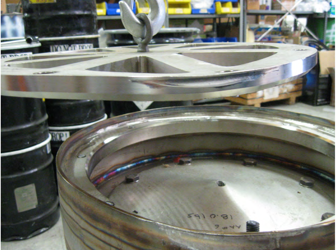
FIGURE B.2-6 – CTU-2 Post-Test Disassembly: View of OP-RMSC Closure Lid w/ CG-Over-Top Corner Impact Damage
