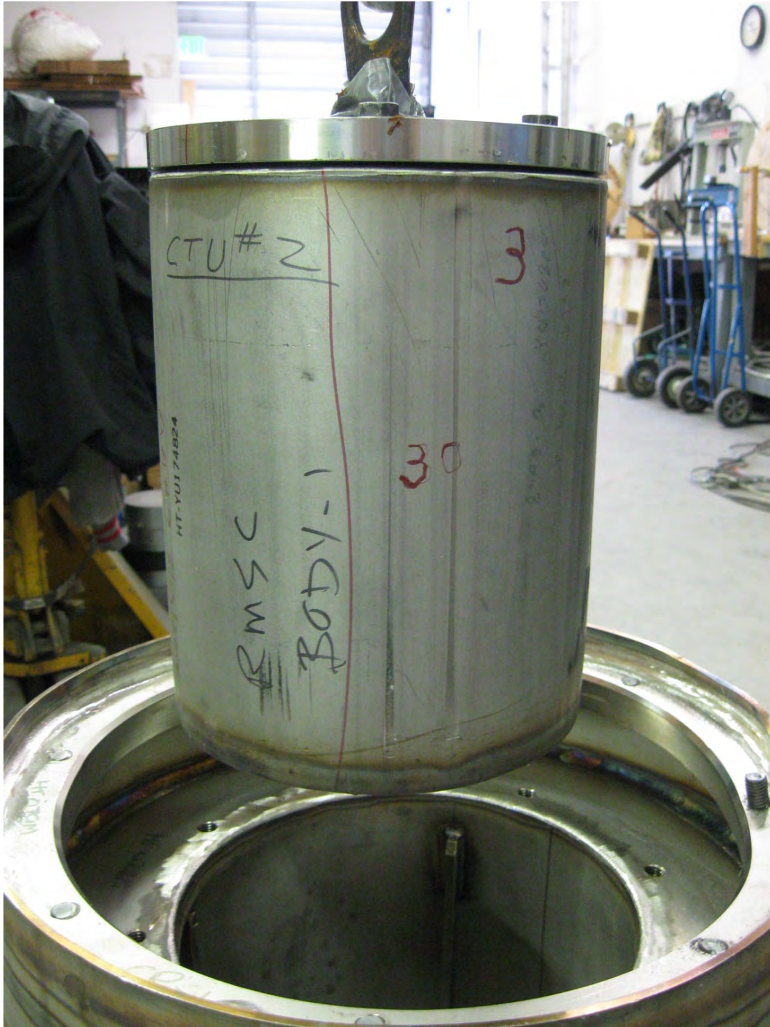
FIGURE B.2-8 – CTU-2 Post-Test Disassembly: Overall View of RMSC Payload
