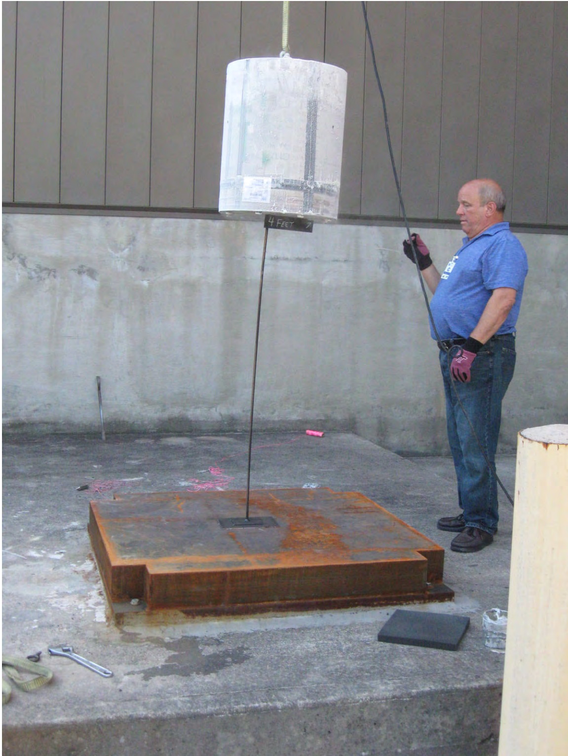
FIGURE B.1.1-1 – Test Unit Immediately Prior to NCT 4-Foot Top Down Drop
