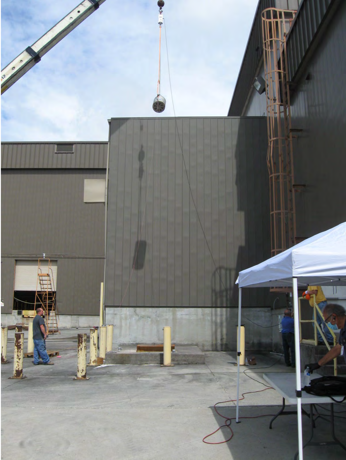
FIGURE B.1.4-1 – Test Unit Immediately Prior to HAC 30-Foot CG-Over-Top Corner Drop
