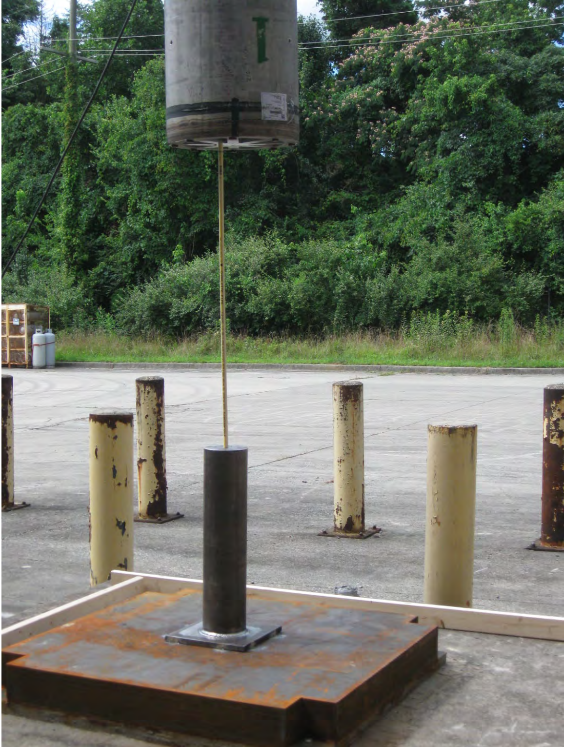
FIGURE B.1.5-1 – Test Unit Prior to HAC Puncture Drop on Top
