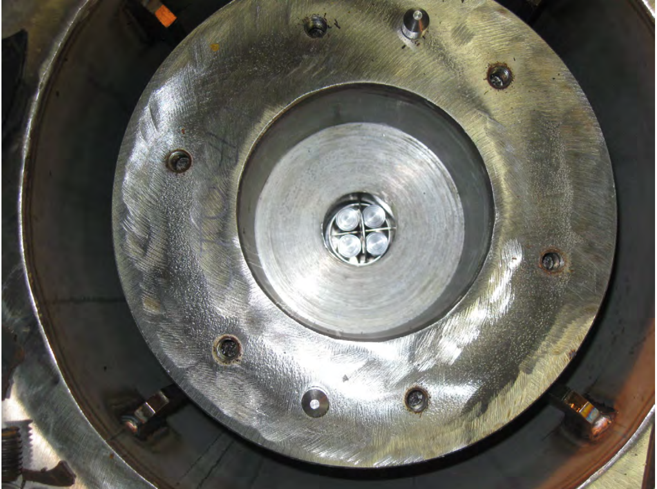
FIGURE B.2-5 – CTU-1 Post-Test Disassembly: View of Dummy Sources in RMSC Payload
