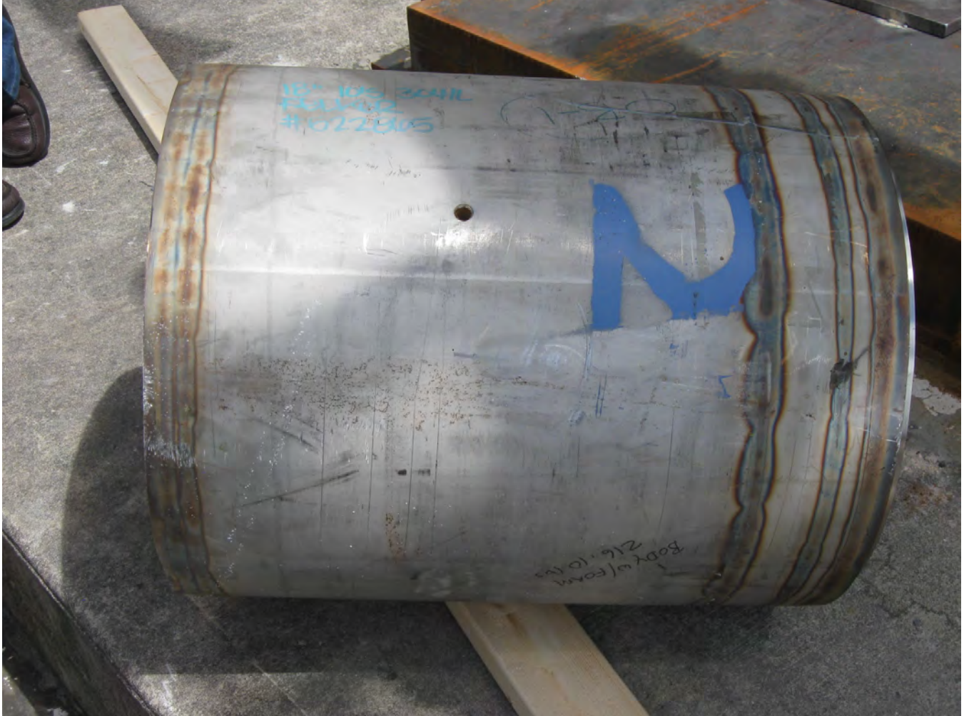
FIGURE B.1.6-2 – Close-up View of Side After Puncture Drop
