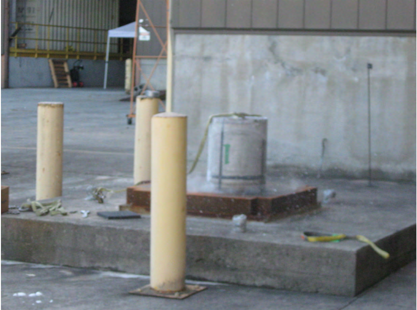
FIGURE B.1.2-2 – Test Unit at Impact, HAC 30-Foot Top Down Drop
