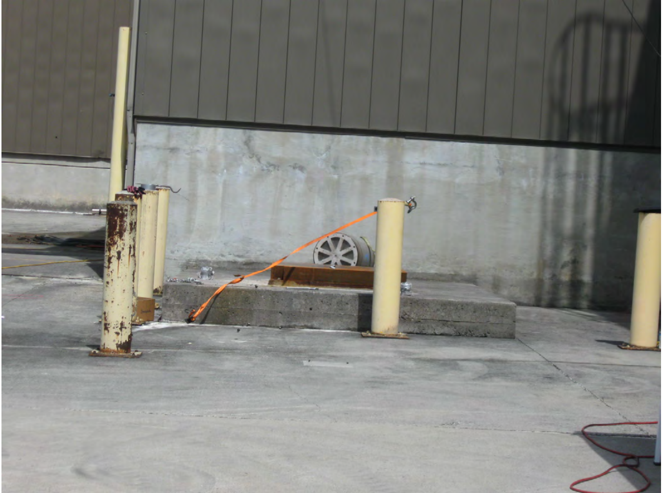
FIGURE B.1.4-2 – Test Unit After HAC 30-Foot CG-Over-Top Corner Drop
