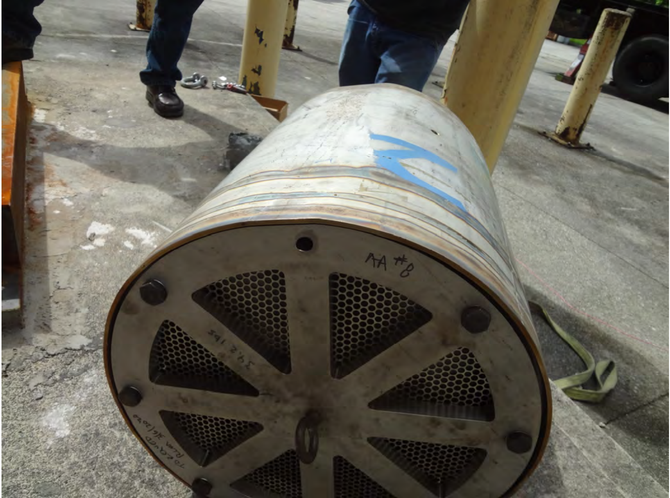
FIGURE B.1.3-3 – Close-up View of Deformed Side Flat (~4 inch Width), Failed Closure Lid Bolt, HAC 30-Foot Side Drop
