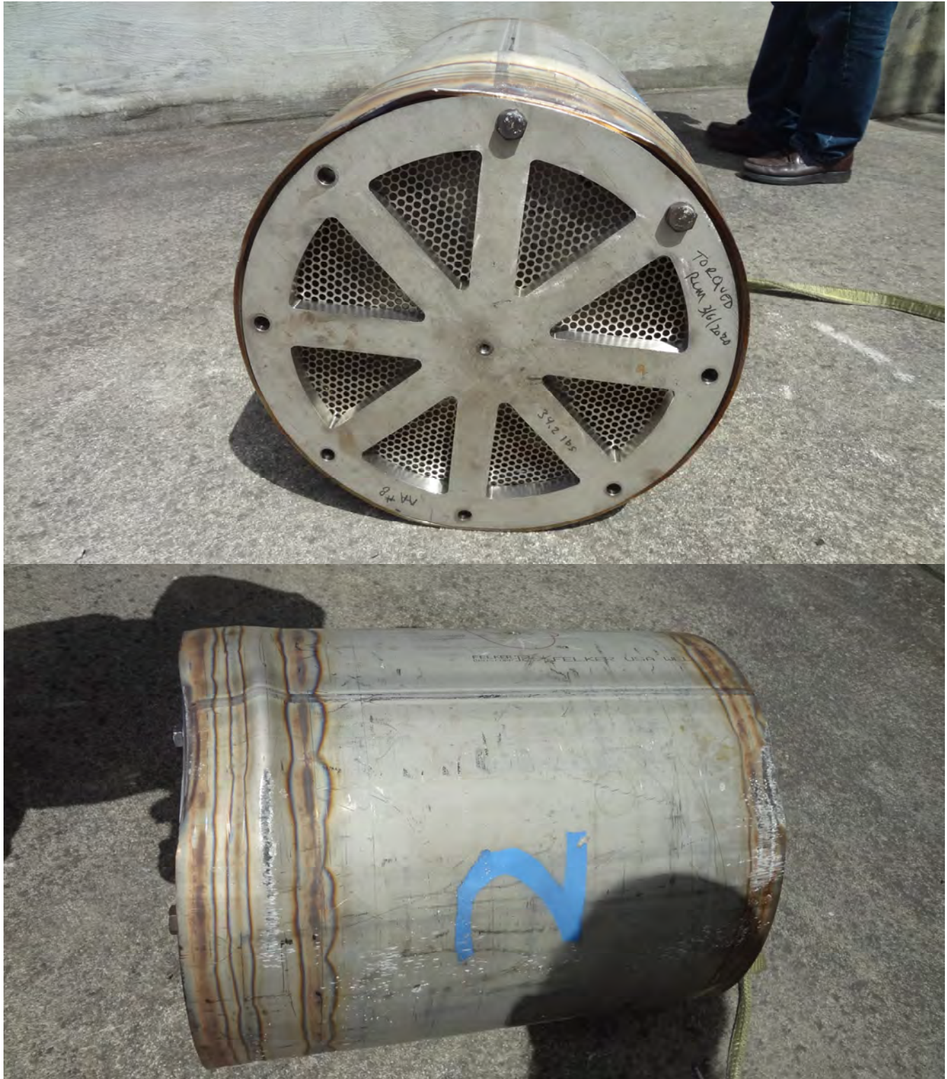
FIGURE B.1.4-3 –View of Failed Closure Lid Bolts, Deformed Shell/Lid Interface, HAC 30-Foot CG-Over-Top Corner Drop
