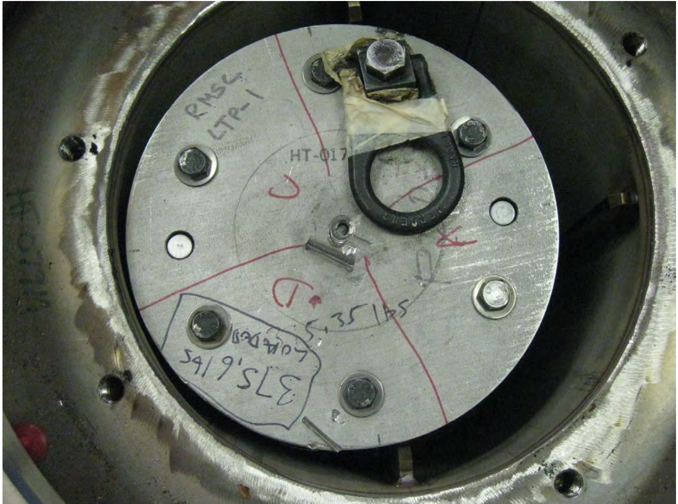
FIGURE B.2-7 – CTU-2 Post-Test Disassembly: View of RMSC Payload w/ Sheared Hoist Ring Hex Bolt and CG-Over-Top Corner Impact Damage to Lid
