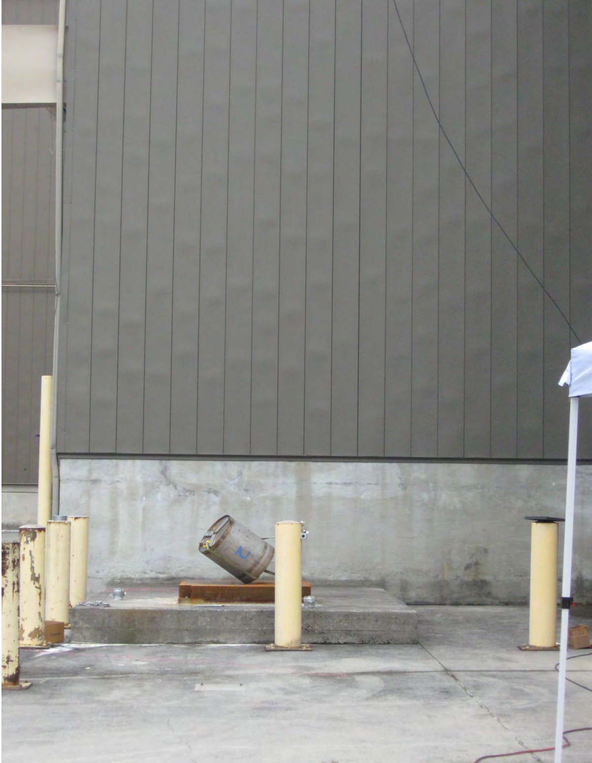
FIGURE B.1.3-2 – Test Unit Immediately After HAC 30-Foot Side Drop
