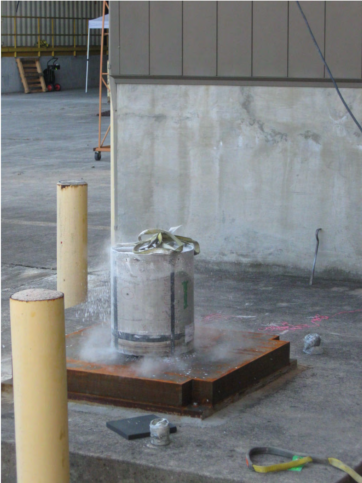
FIGURE B.1.1-2 – Test Unit at Impact, NCT 4-Foot Top Down Drop
