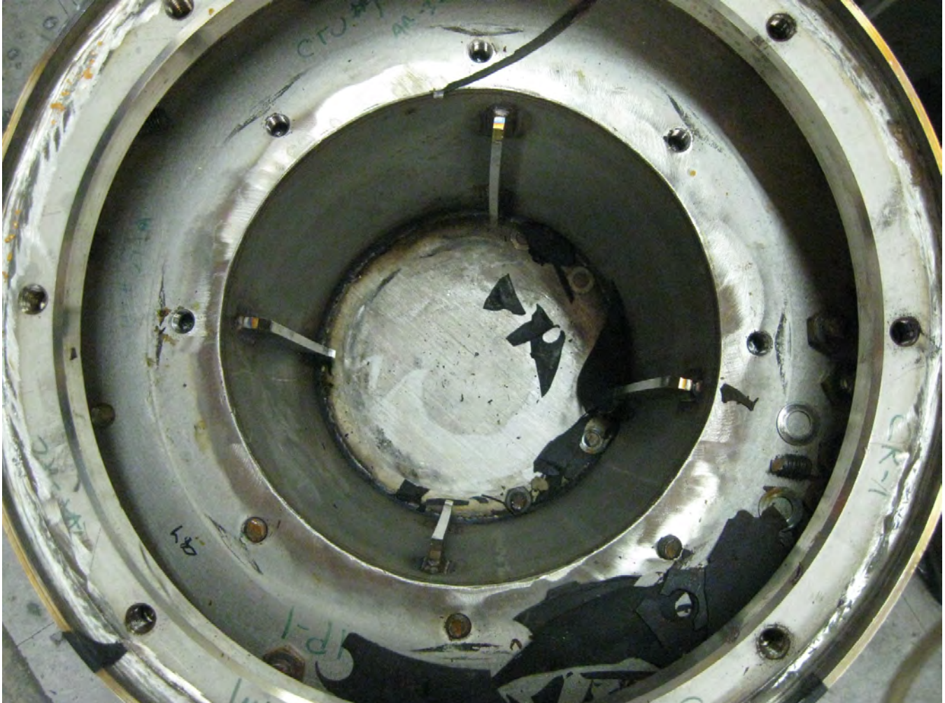
FIGURE B.2-3 – CTU-1 Post-Test Disassembly: View of OP-RMSC Payload Cavity
