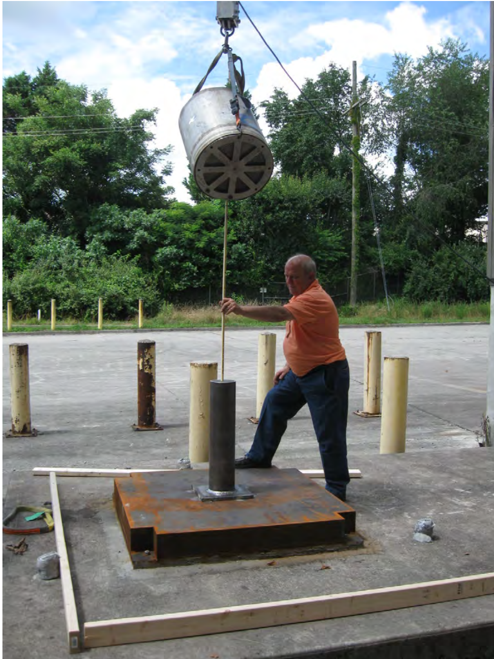
FIGURE B.1.7-1 – Test Unit Prior to HAC Puncture Drop on CG-Over-Top Corner
