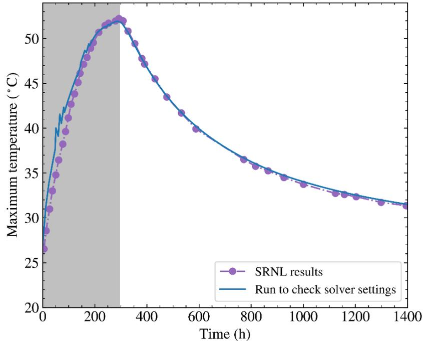
Figure 1. Results from run for checking solver settings, compared with results from SRNL [1]. The gray band indicates the timing of the first grout pour.
