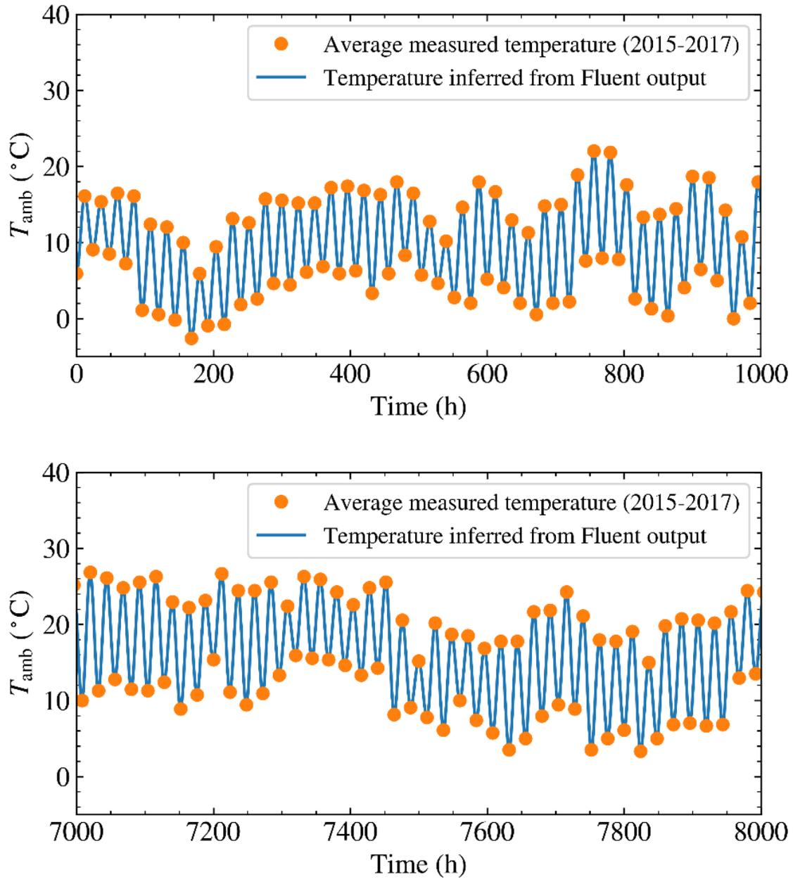
Figure 2. Ambient temperature inferred from Fluent output (blue curve), compared with the average measured temperatures used as inputs (orange circles), for two representative 1000-hour periods.
