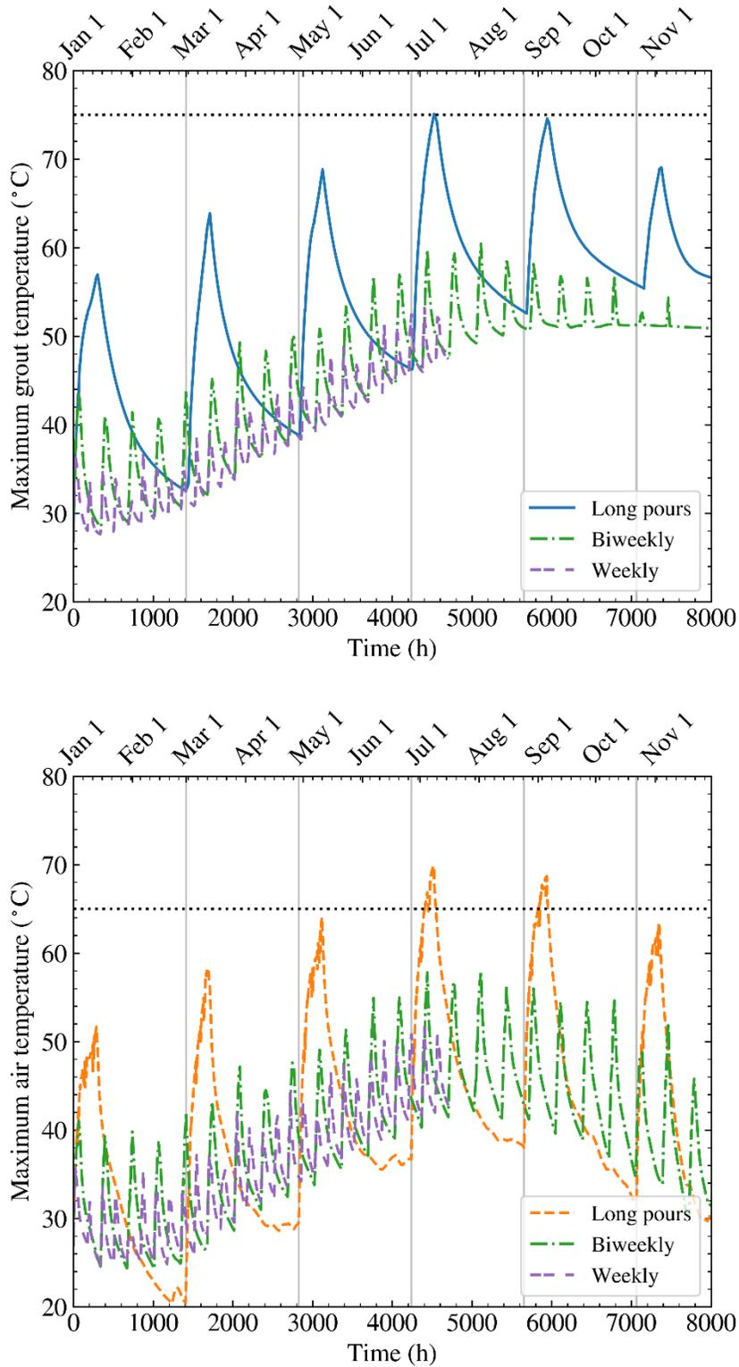
Figure 6. Comparison of maximum grout (upper) and air (lower) temperatures predicted for different pour schedules [long pours: 12.3 days pouring + 46.6 days idling; biweekly: 70.35 h + 265.65 h [nominal]; weekly: 35.17 h + 132.83 h [nominal]]. The vertical gray lines indicate the starts of the pours in the long-pour schedule. The horizontal dotted lines indicate the relevant DSA limits.
