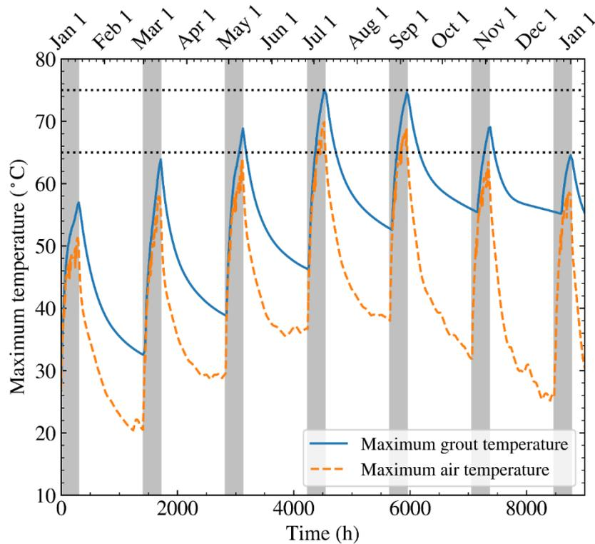
Figure 3. Maximum grout temperature (blue solid curve) and maximum air temperature (orange dashed curve) in SDU 6 during one year of pouring cement-free grout. The pouring is assumed to start on January 1<sup>st</sup>. The gray bands indicate the timings of the pours. The horizontal dashed lines indicate the maximum allowed grout and air temperatures (75 °C and 65 °C, respectively [3]).
