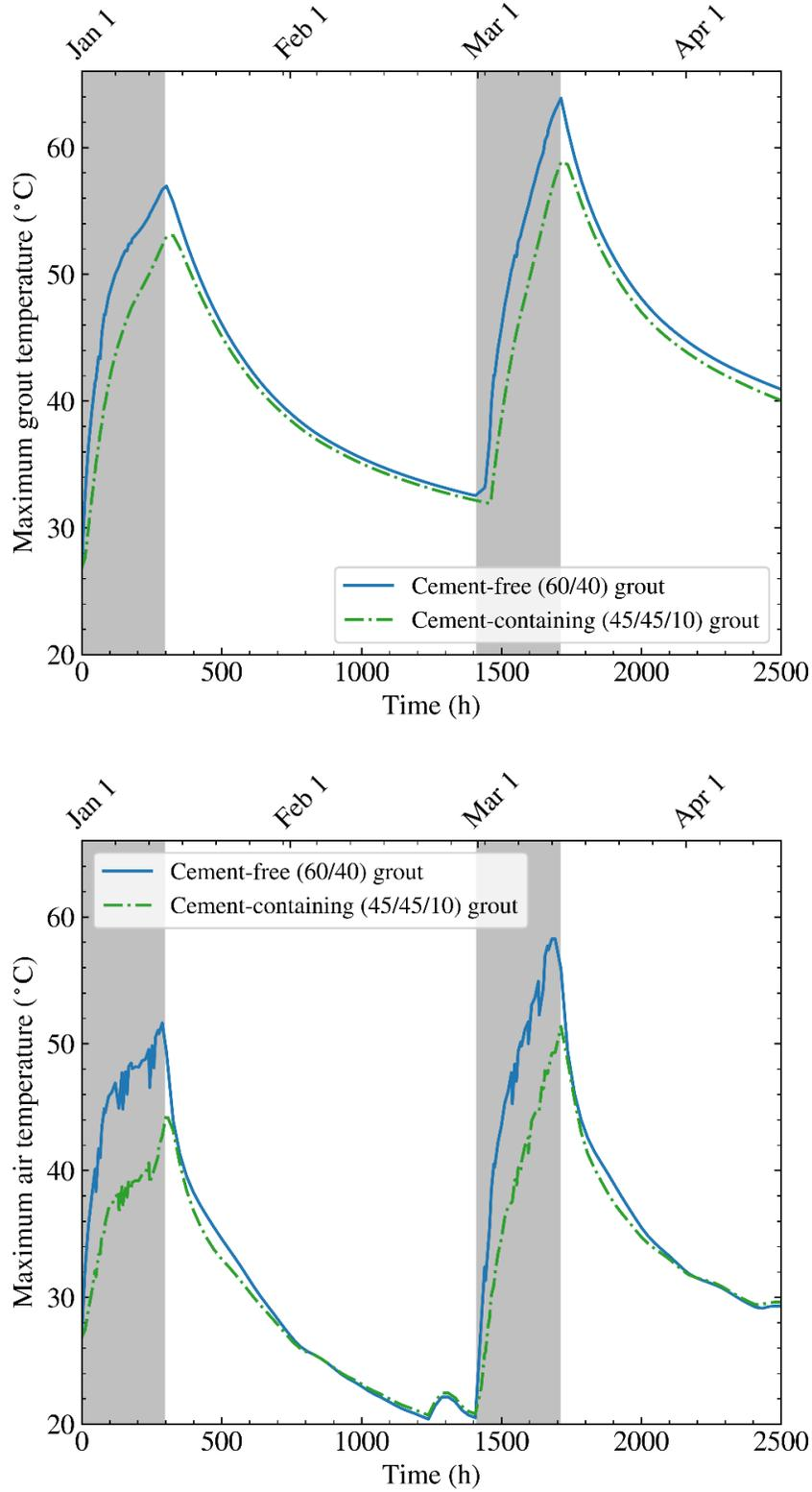
Figure 5. Comparison of the maximum grout (upper) and air (lower) temperatures in SDU 6 predicted for cement-free (60/40) grout and for the current cement-containing (45/45/10) grout.
