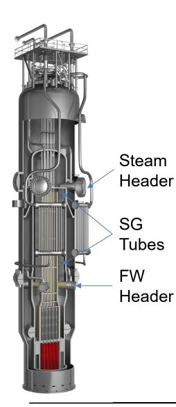
Concern that TF-2 is not a prototypical test for NuScale SG design; pump flow is not constant, vertical height difference
