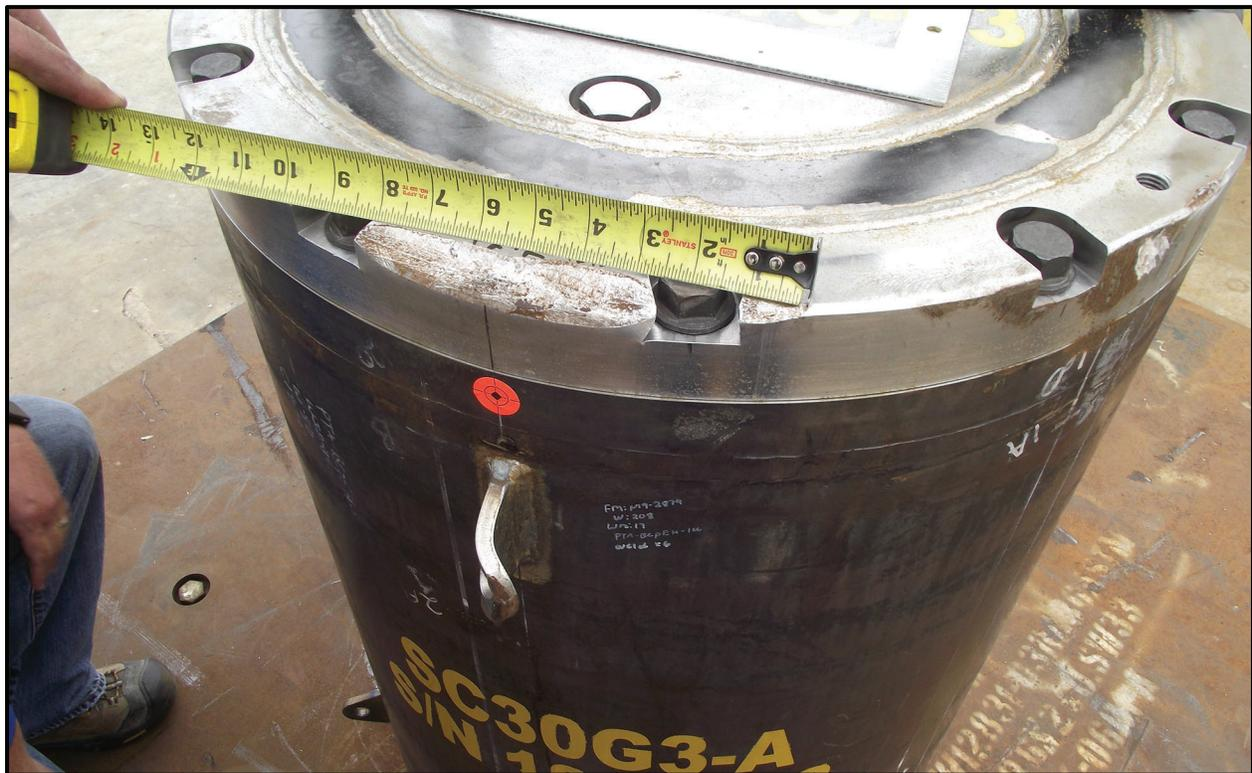
Figure 6-55 – SC-30G3 18TU-03 Center-of-Gravity Over Top Corner Drop Damage 1
