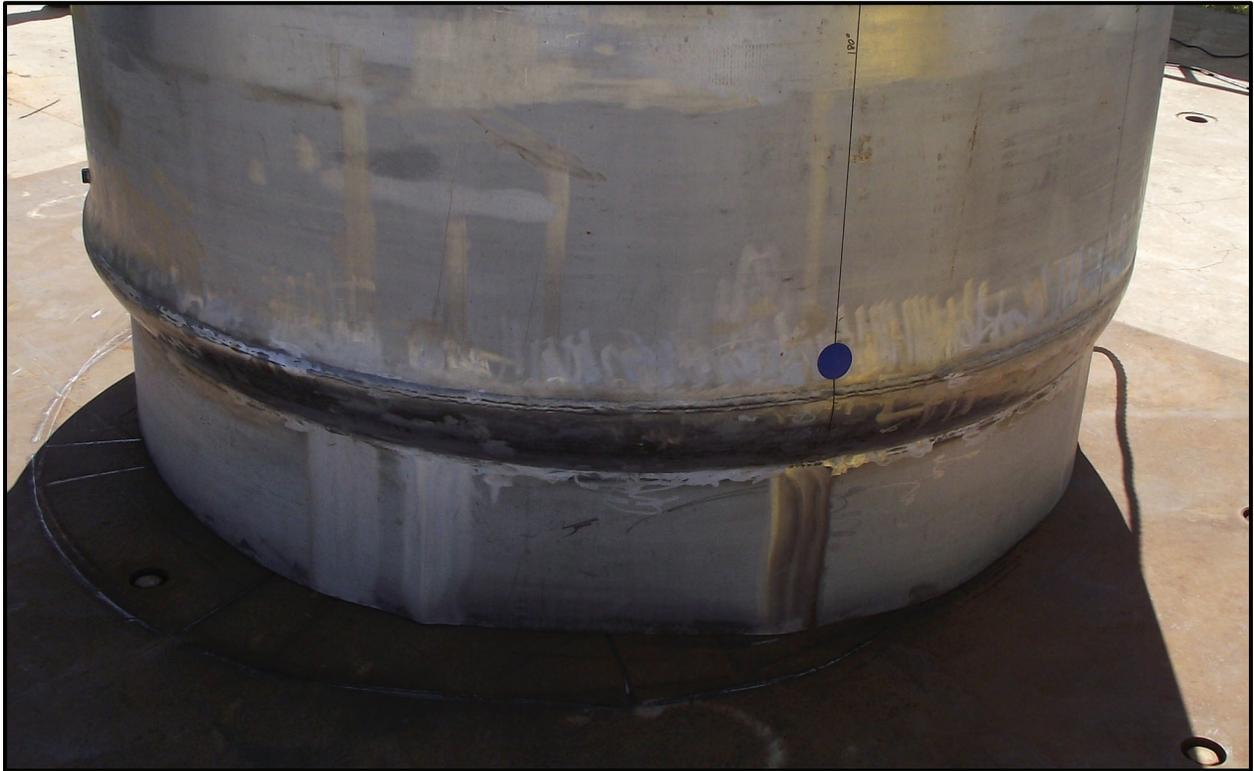
**Figure 6-31** – SC-30G3 End Drop Hoop Damage to the ICV Shell
