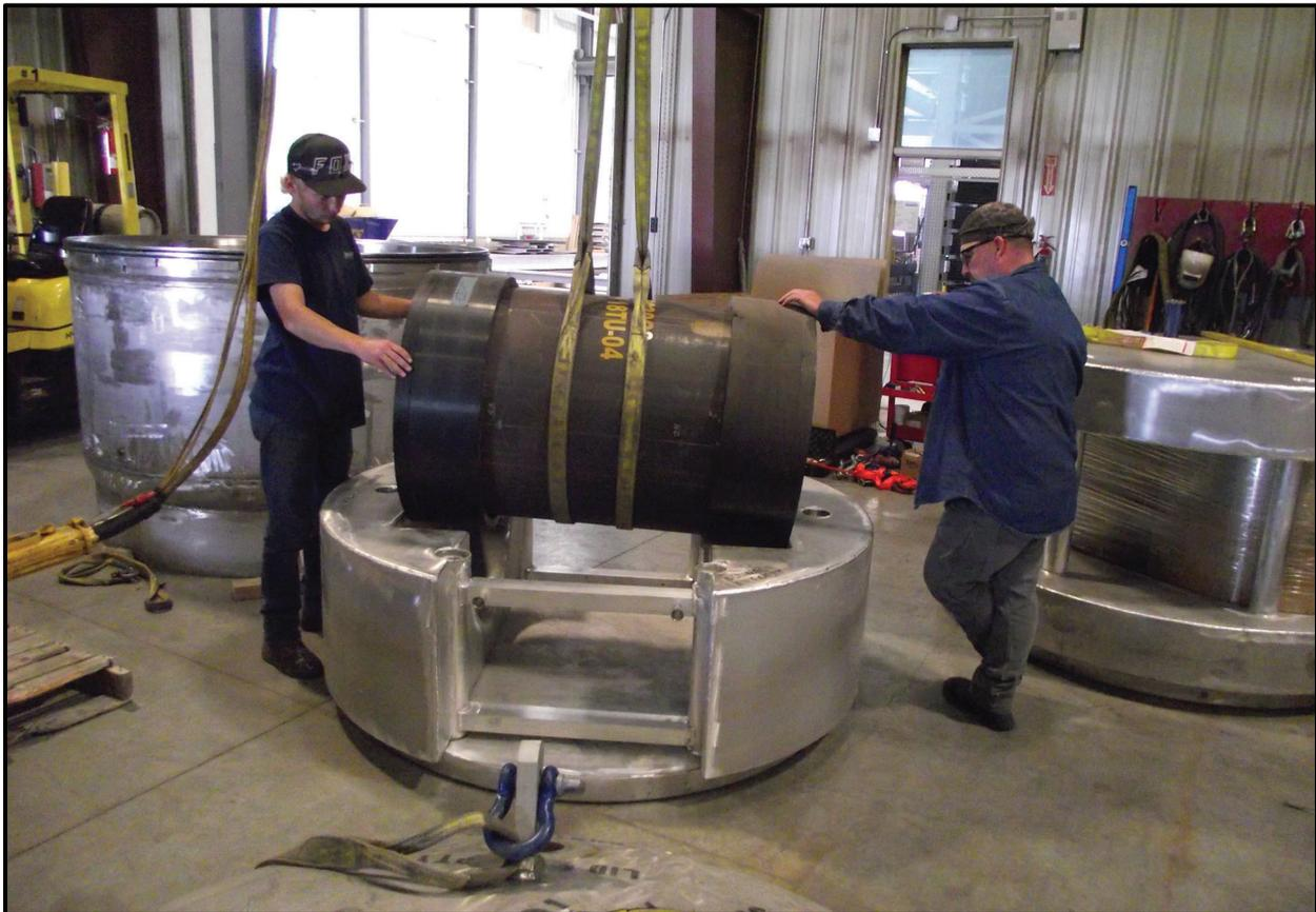
**Figure 6-28** – SC-30G3 with End Caps Loaded into Lateral Dunnage
