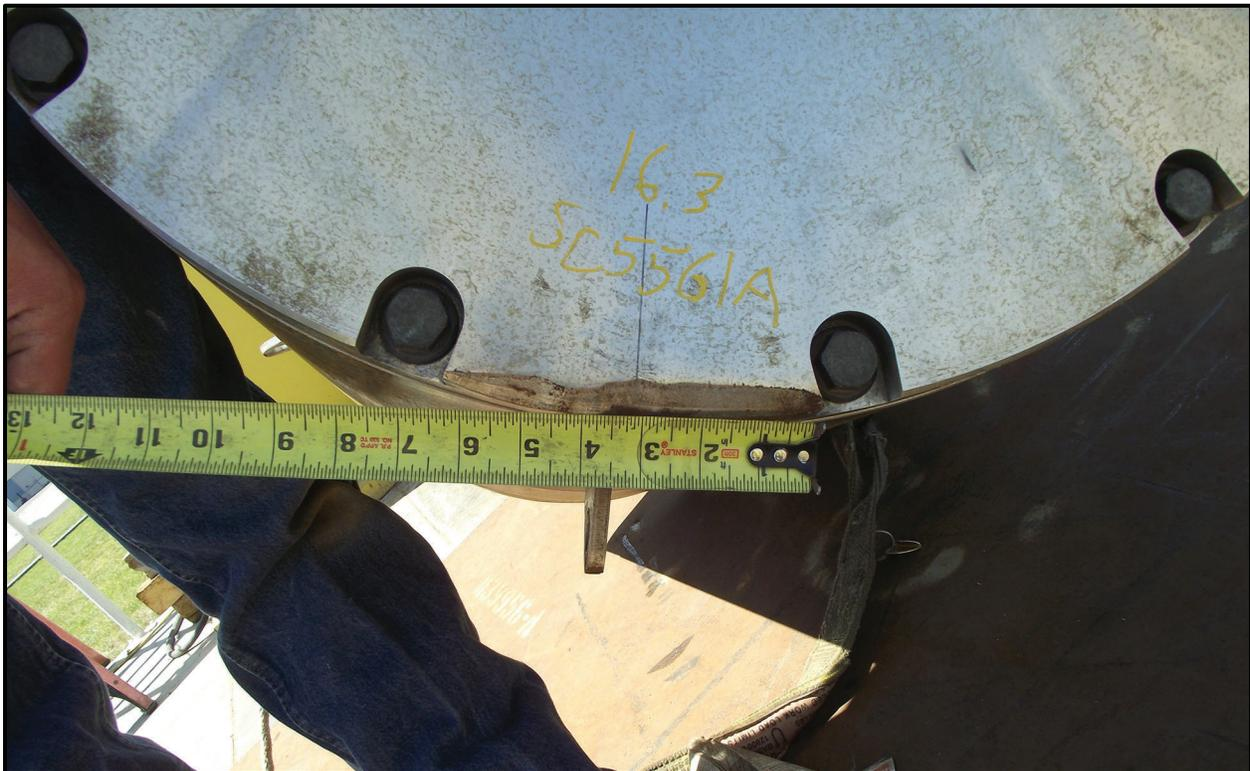
Figure 6-23 – SC-55G1 18TU-06 Center-of-Gravity Over Top Corner Drop Damage 1
