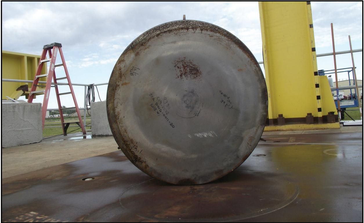
**Figure 6-58** – SC-30G3 18TU-03 Vertical Bottom End Drop Damage 2
