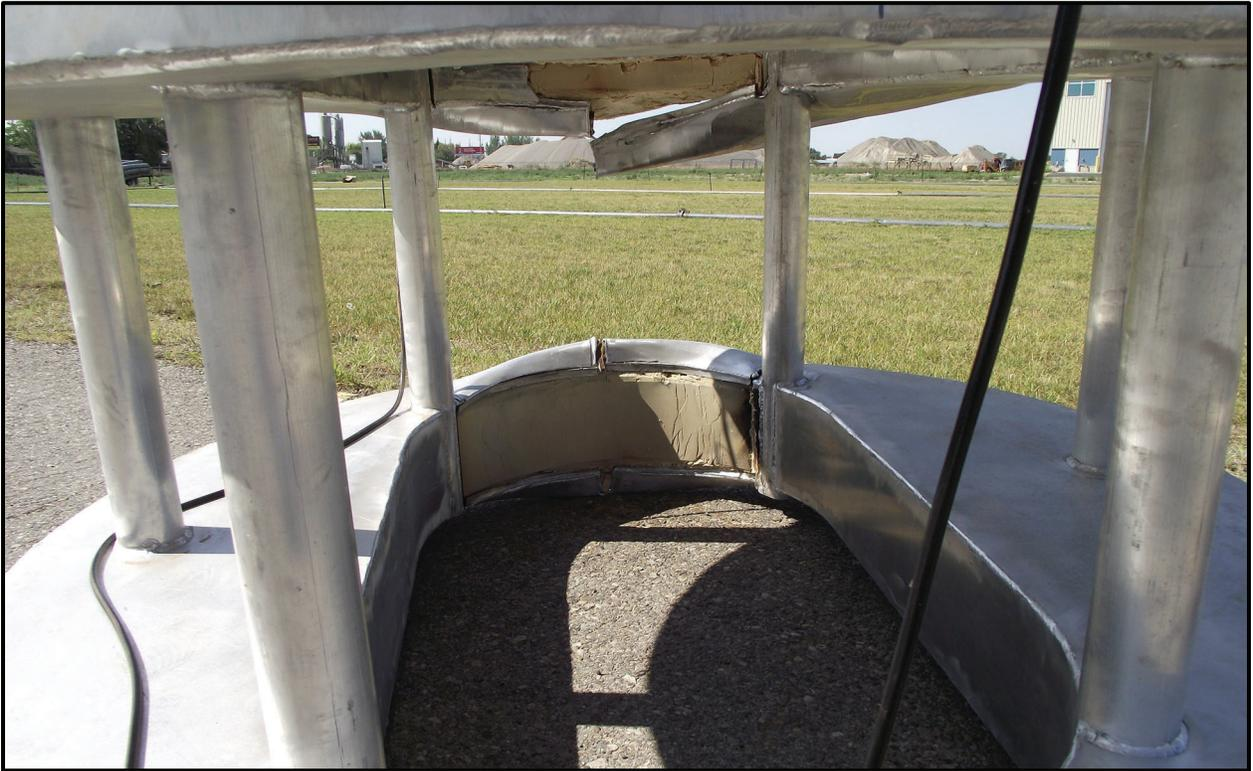
Figure 6-13 – SC-55G1 Radial Dunnage Side Drop Damage
