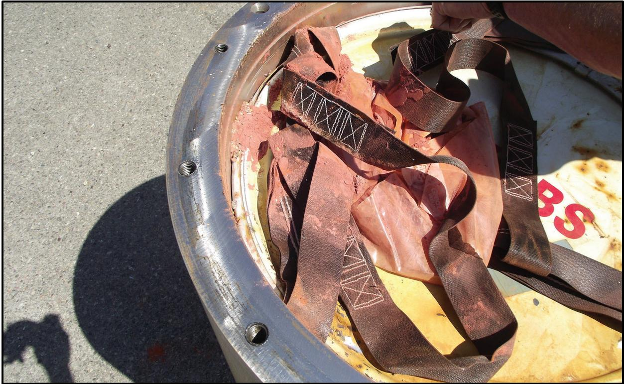
**Figure 6-21** – Fluorescein Dye inside the SC-55G1 Body
