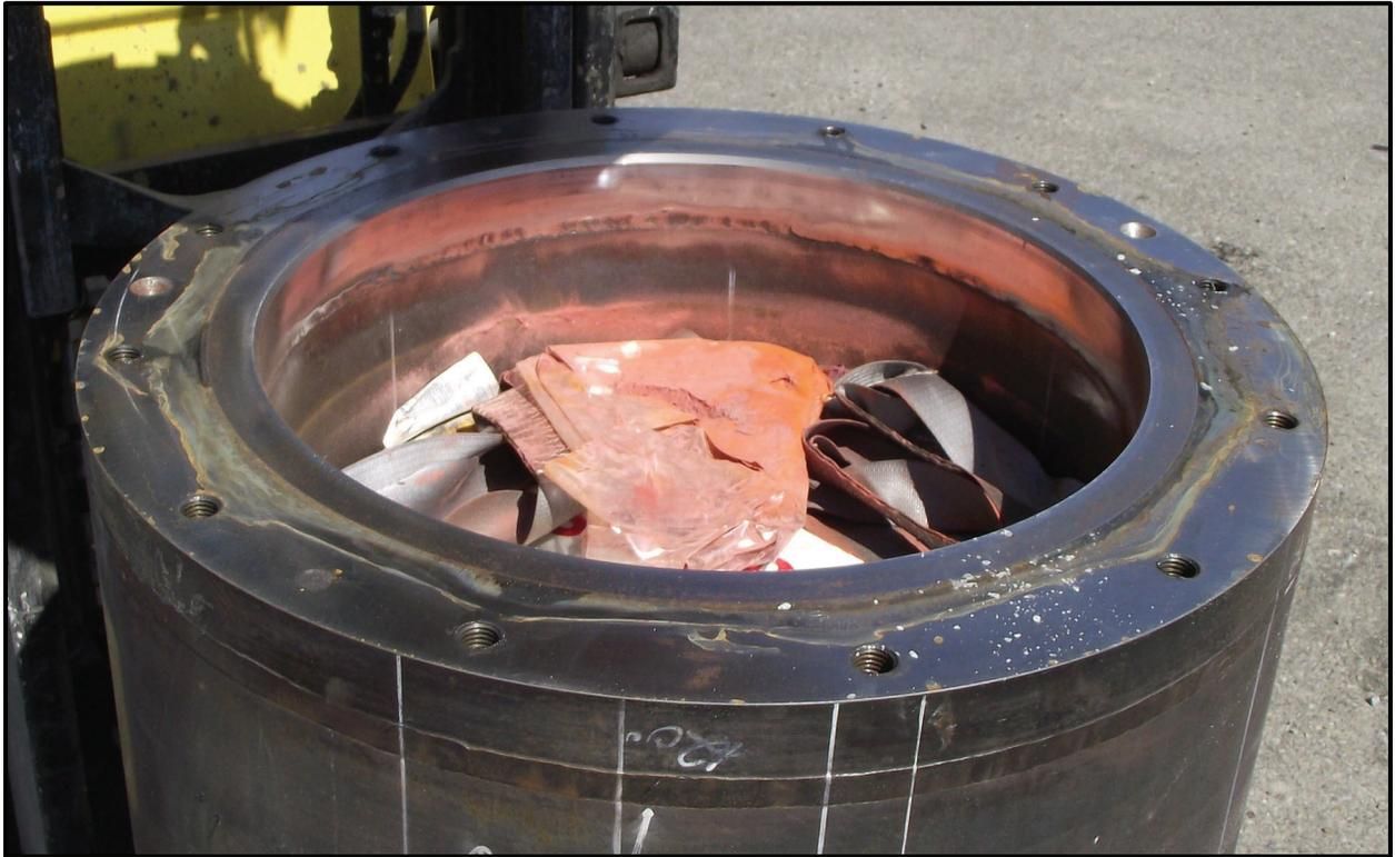
**Figure 6-43** – Fluorescein Dye inside the SC-30G3 Body
