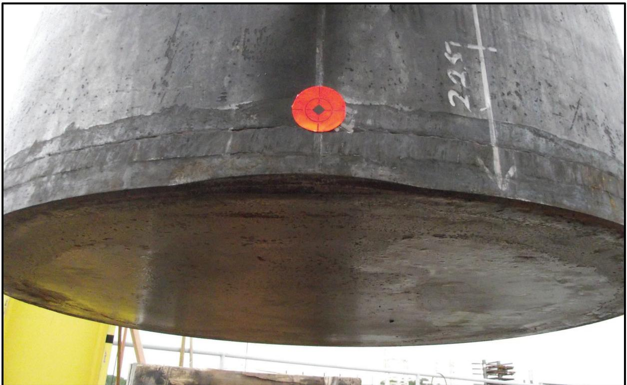
Figure 7-6 – SC-30G2 18TU-01 Vertical End Drop Damage
