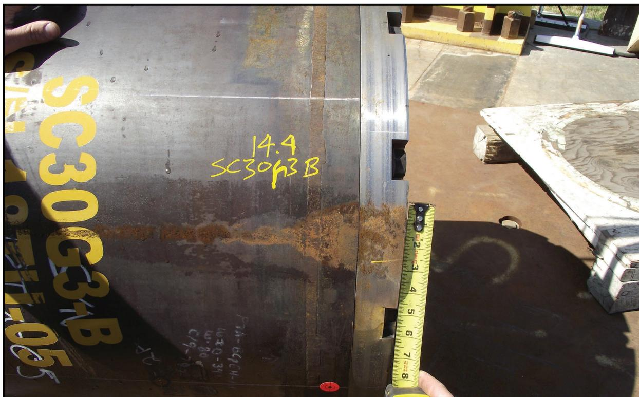
Figure 6-63 – SC-30G3 18TU-05 Side Drop Lid-End Damage
