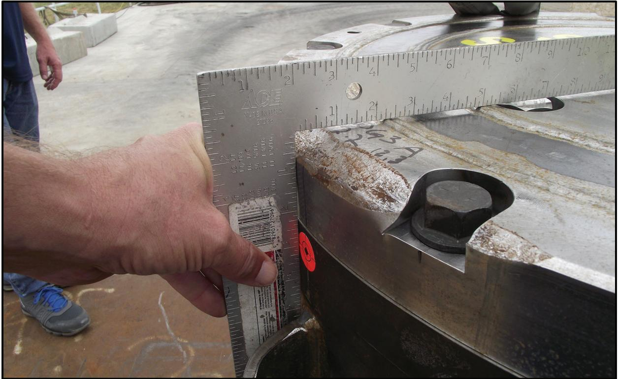
Figure 6-56 – SC-30G3 18TU-03 Center-of-Gravity Over Top Corner Drop Damage 2
