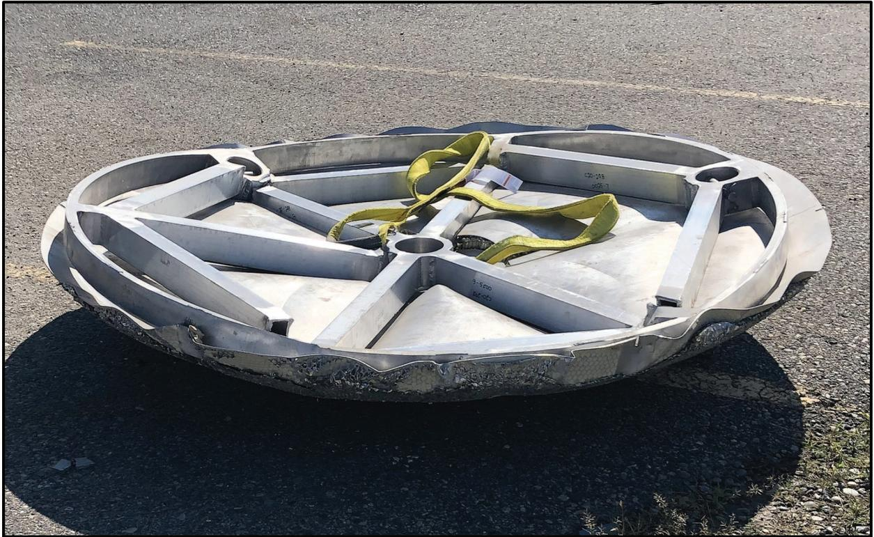
**Figure 6-11** – Deformed Heavy-Duty Pallet and Lower Spacer
