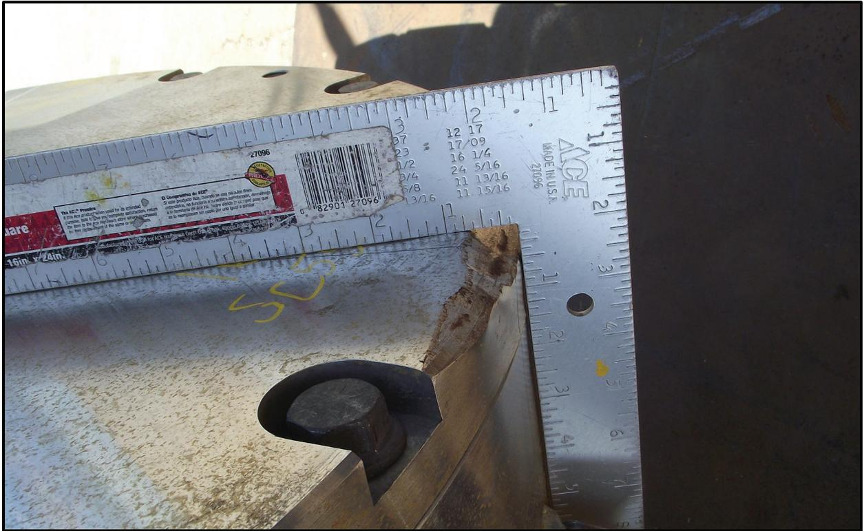
Figure 6-24 – SC-55G1 18TU-06 Center-of-Gravity Over Top Corner Drop Damage 2
