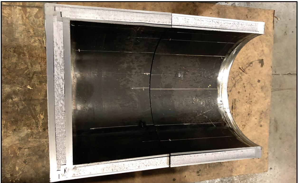
**Figure 7-17** – SC-30G2 18TU-02 Destructive Disassembly Overview
