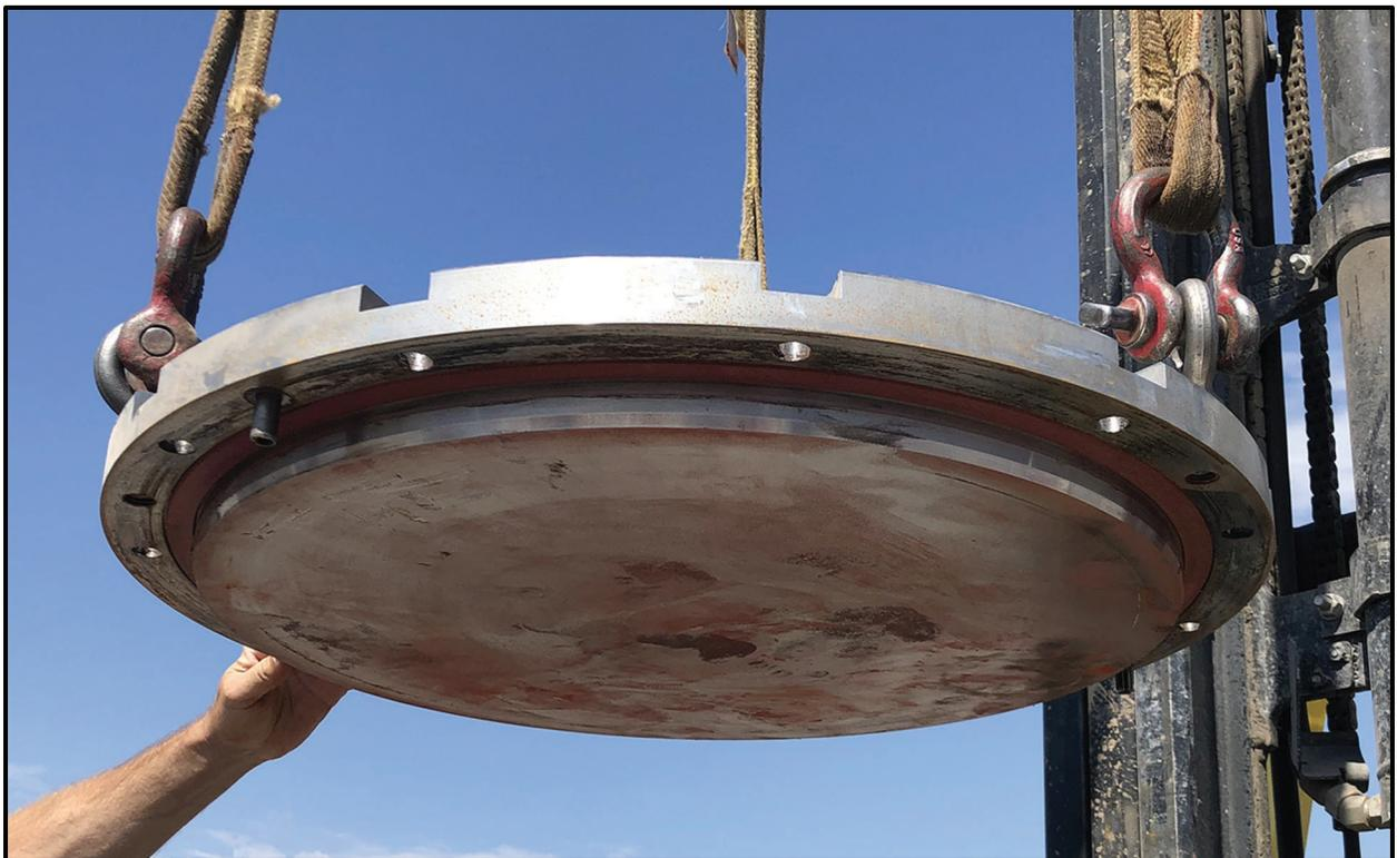
**Figure 6-22** – Fluorescein Dye under the SC-55G1 Lid
