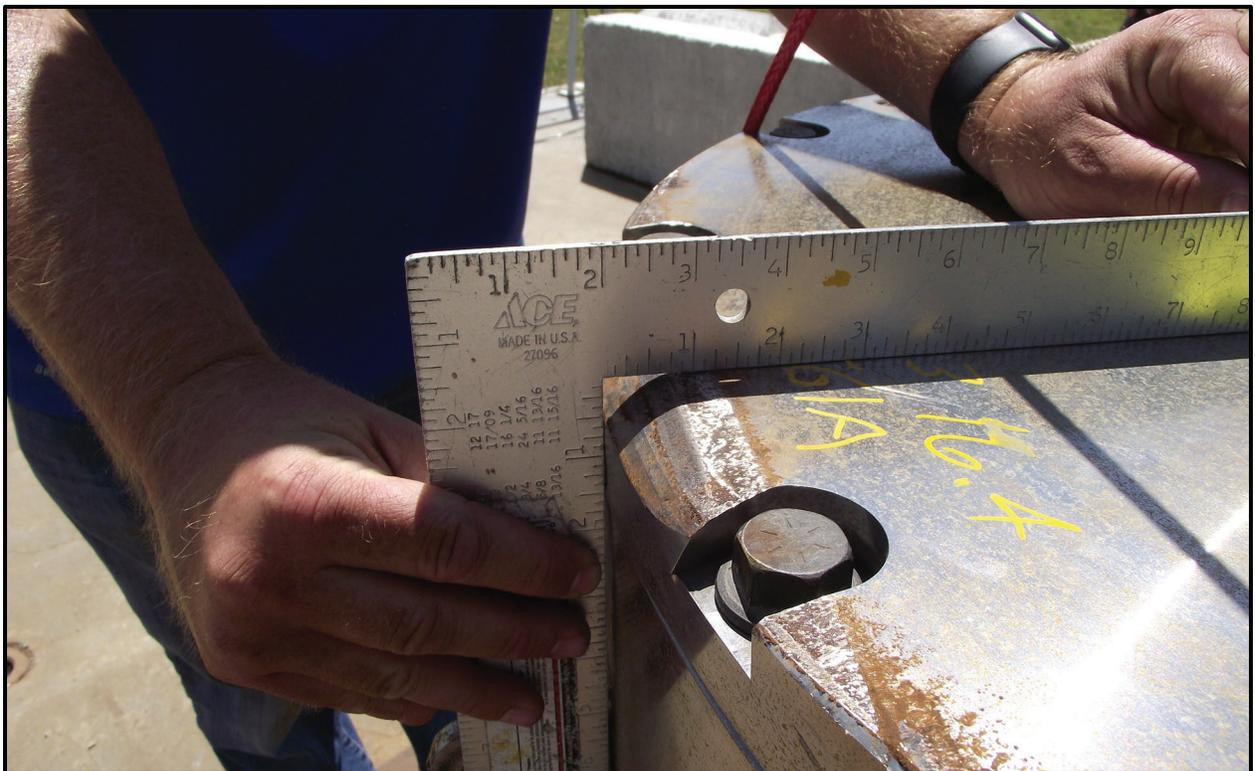
Figure 6-27 – SC-55G1 18TU-06 Top-Down Near-Vertical Drop Damage 2
