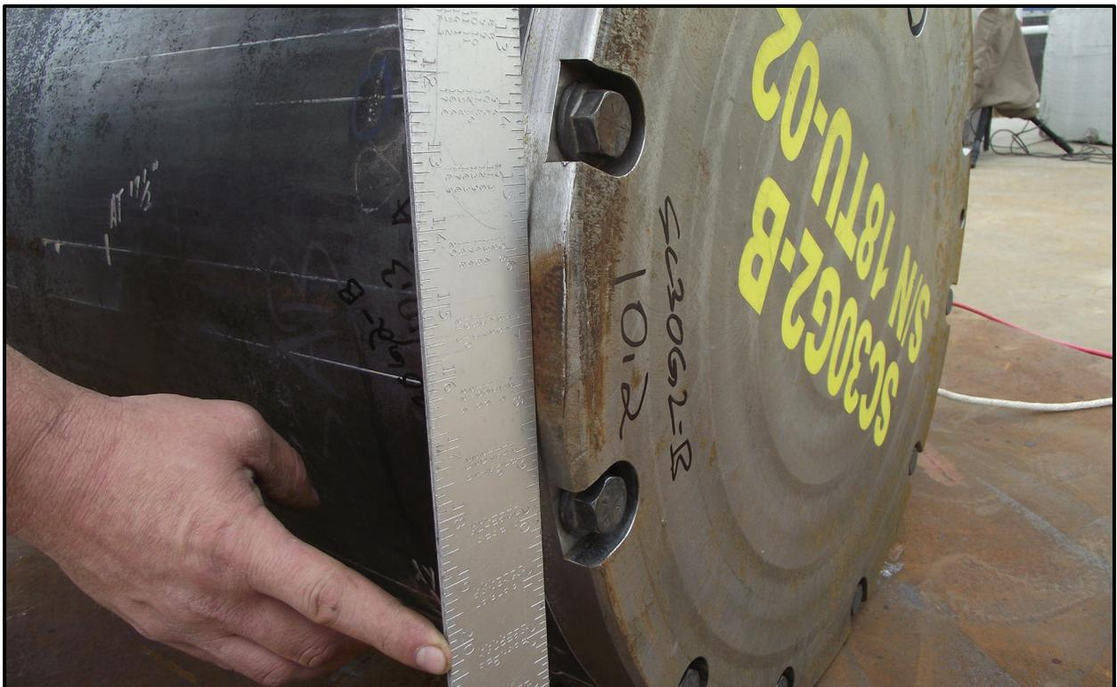
**Figure 7-8** – SC-30G2 18TU-02 Horizontal Side Drop Lid-End Damage
