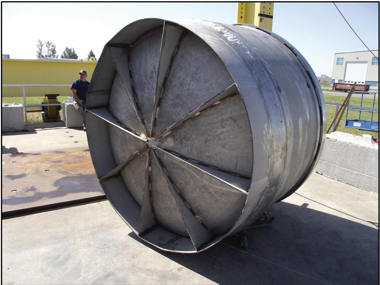
**Figure 4-11** – HalfPACT ICV Bottom Reinforcement Configuration
