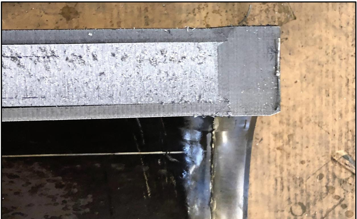
**Figure 7-21** – SC-30G2 18TU-02 Destructive Disassembly Cut AT/AU at Upper Flange
