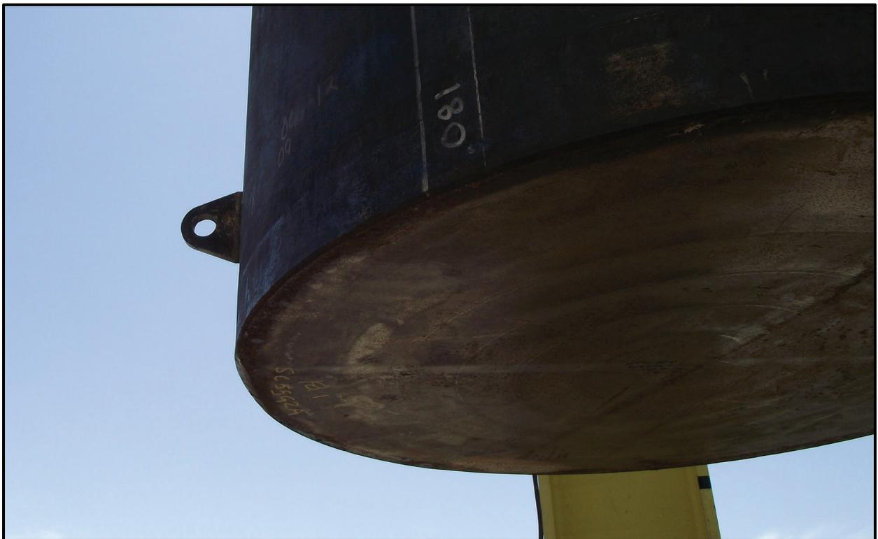
**Figure 7-26** – SC-55G2 18TU-09 Vertical End Drop Damage
