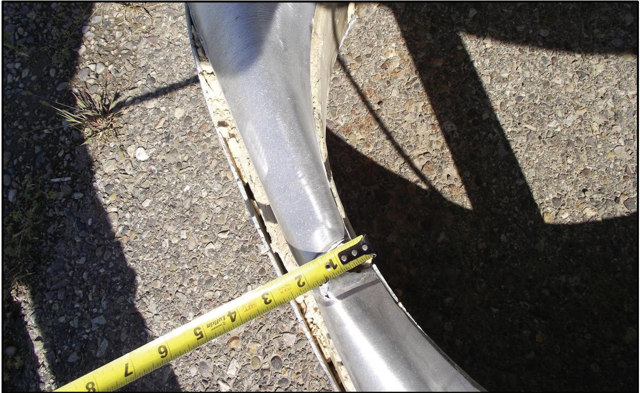
**Figure 6-15 – SC-55G1 Radial Dunnage Lower-End Residual Thickness**
