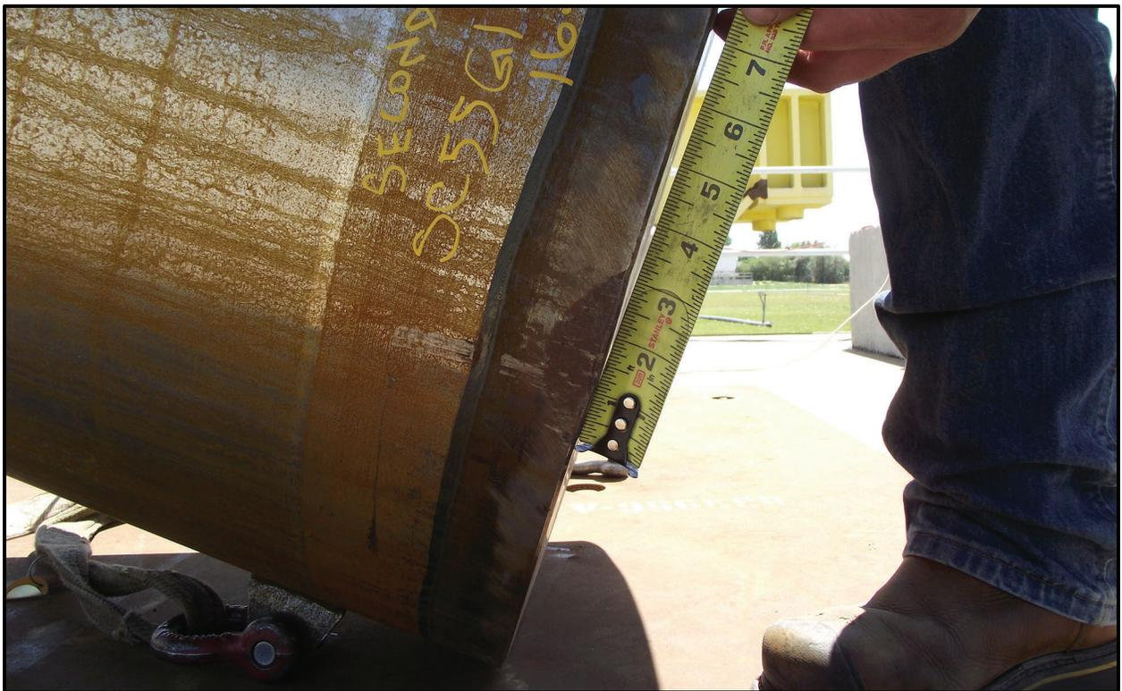
Figure 6-25 – SC-55G1 18TU-06 CG Over Top Corner Drop Secondary Damage
