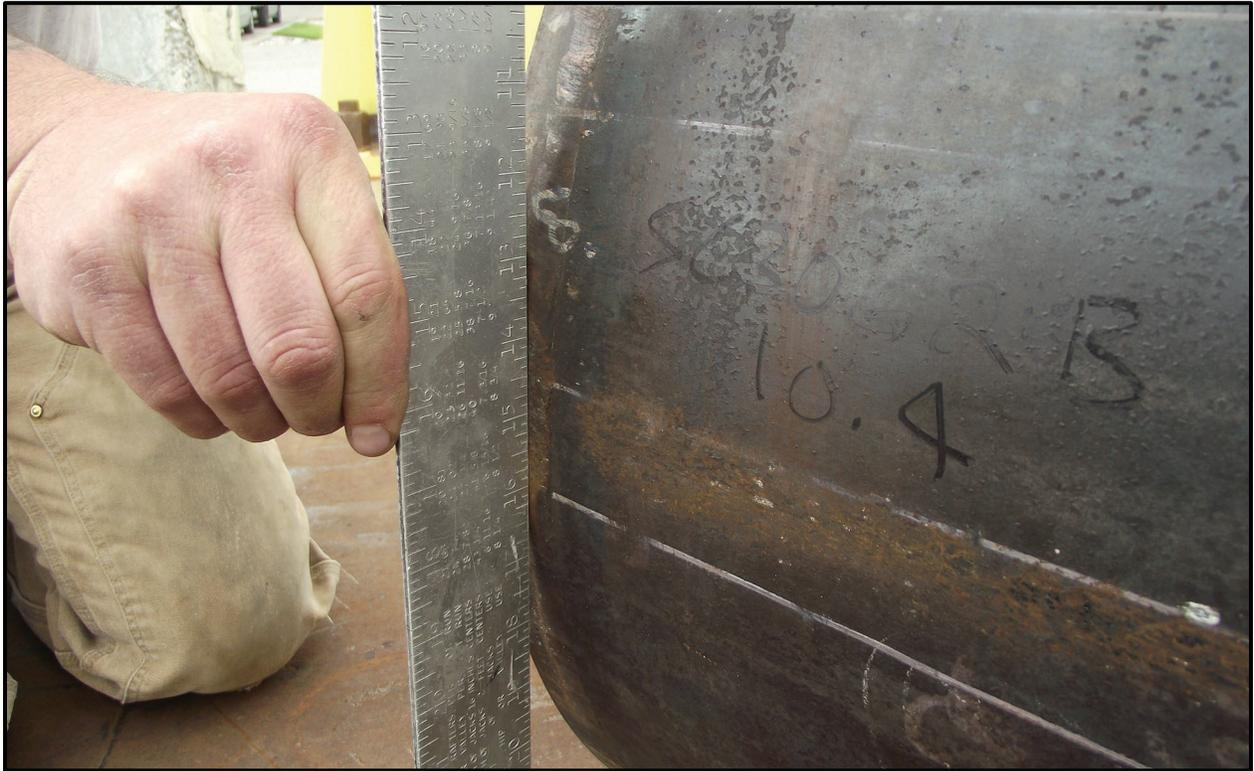
**Figure 7-7** – SC-30G2 18TU-02 Horizontal Side Drop Base-End Damage
