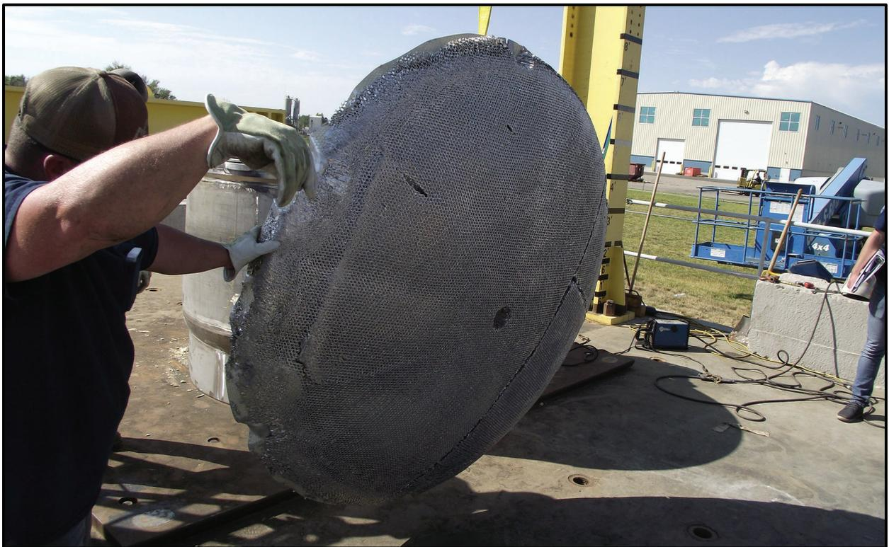
**Figure 6-12** – Deformed Lower Spacer (Bottom-View)
