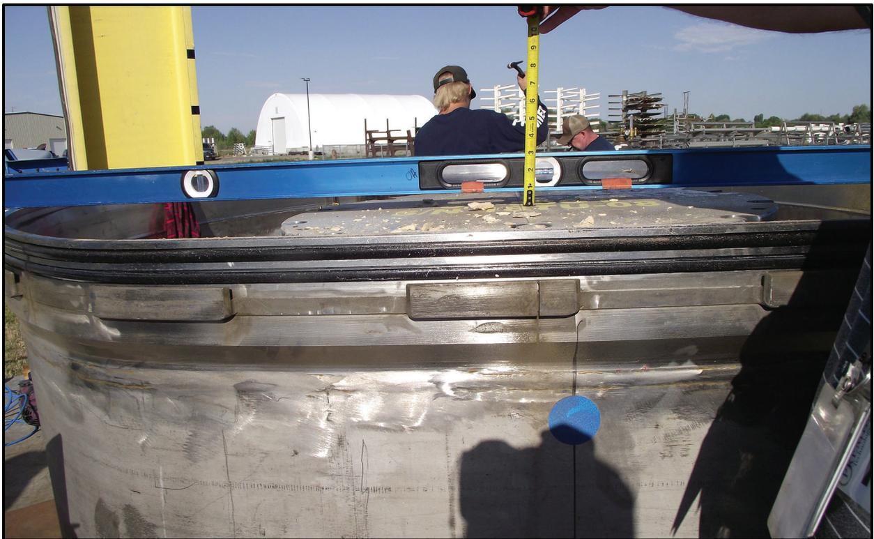
**Figure 6-10** – Post-End Drop Relative Position of SC-55G1s
