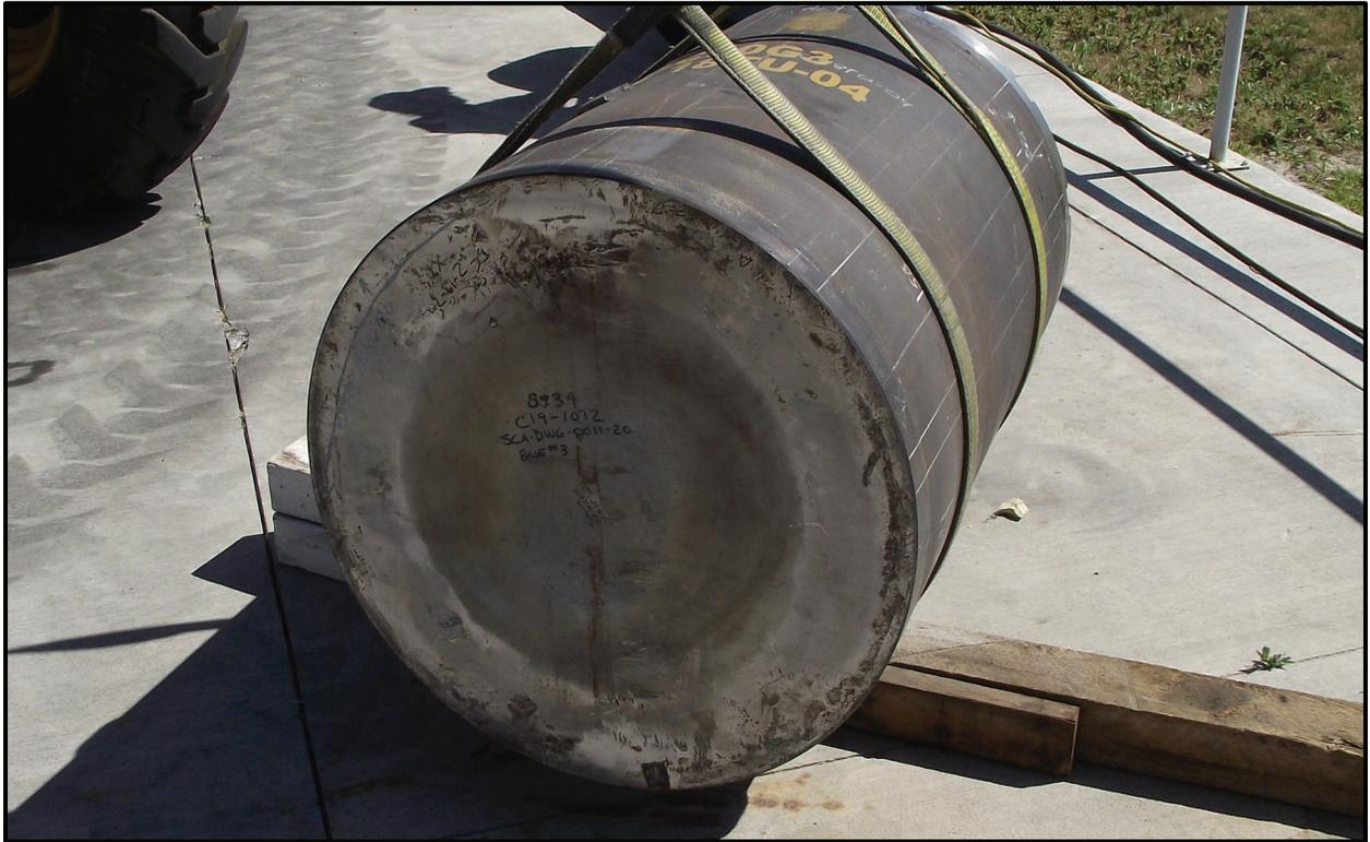
**Figure 7-1 – SC-30G3 18TU-04 HAC Type B 30-foot Vertical End Drop Damage**
