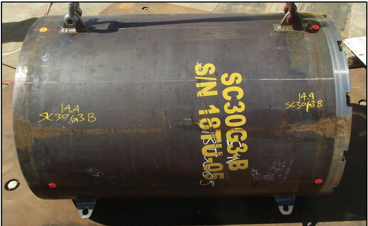
Figure 7-4 – SC-30G3 18TU-03 DOT-7A Type A 4-foot Horizontal Side Drop Damage
