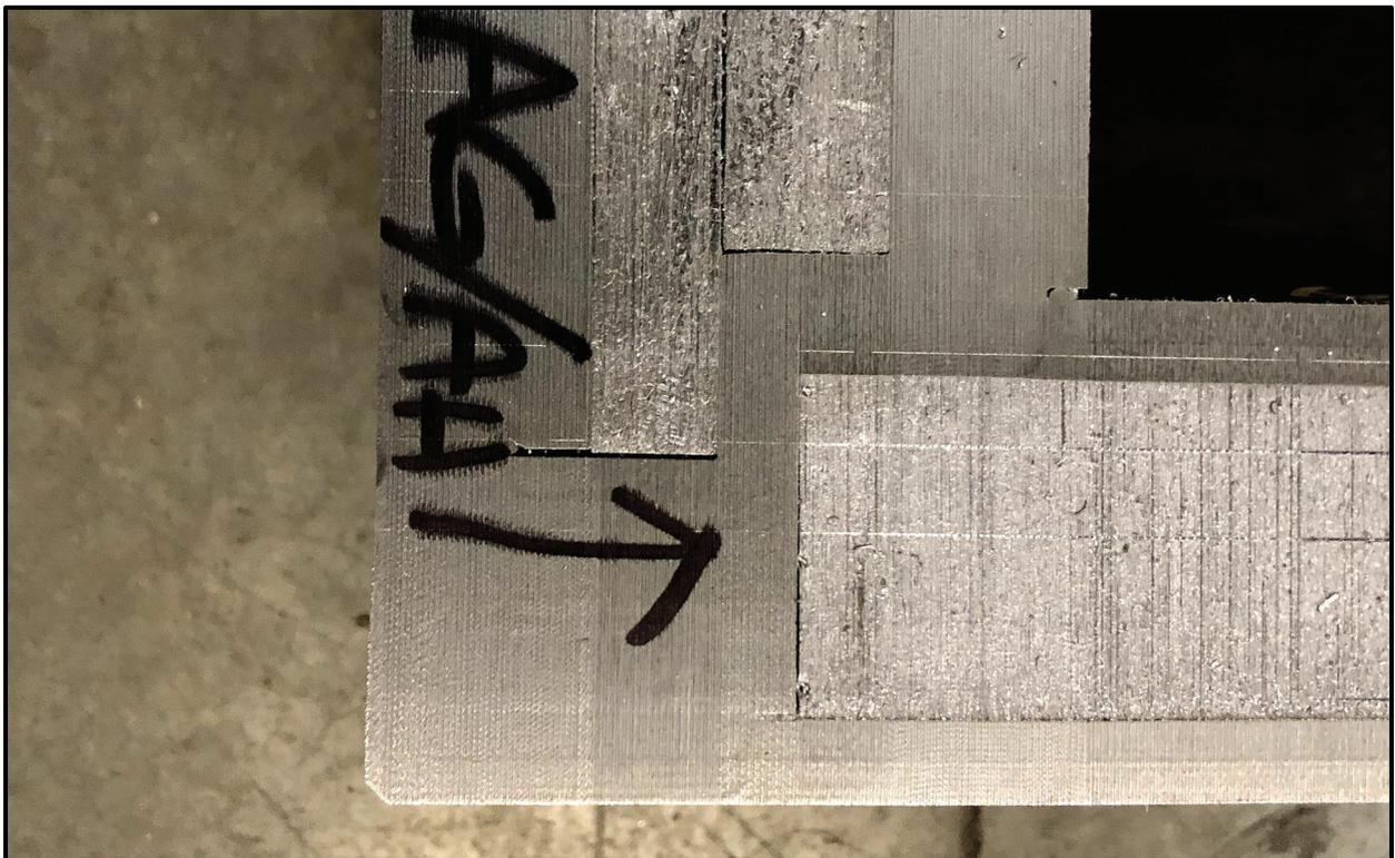
Figure 7-35 – SC-55G2 18TU-09 Destructive Disassembly Cut AG/AH at Lower Flange
