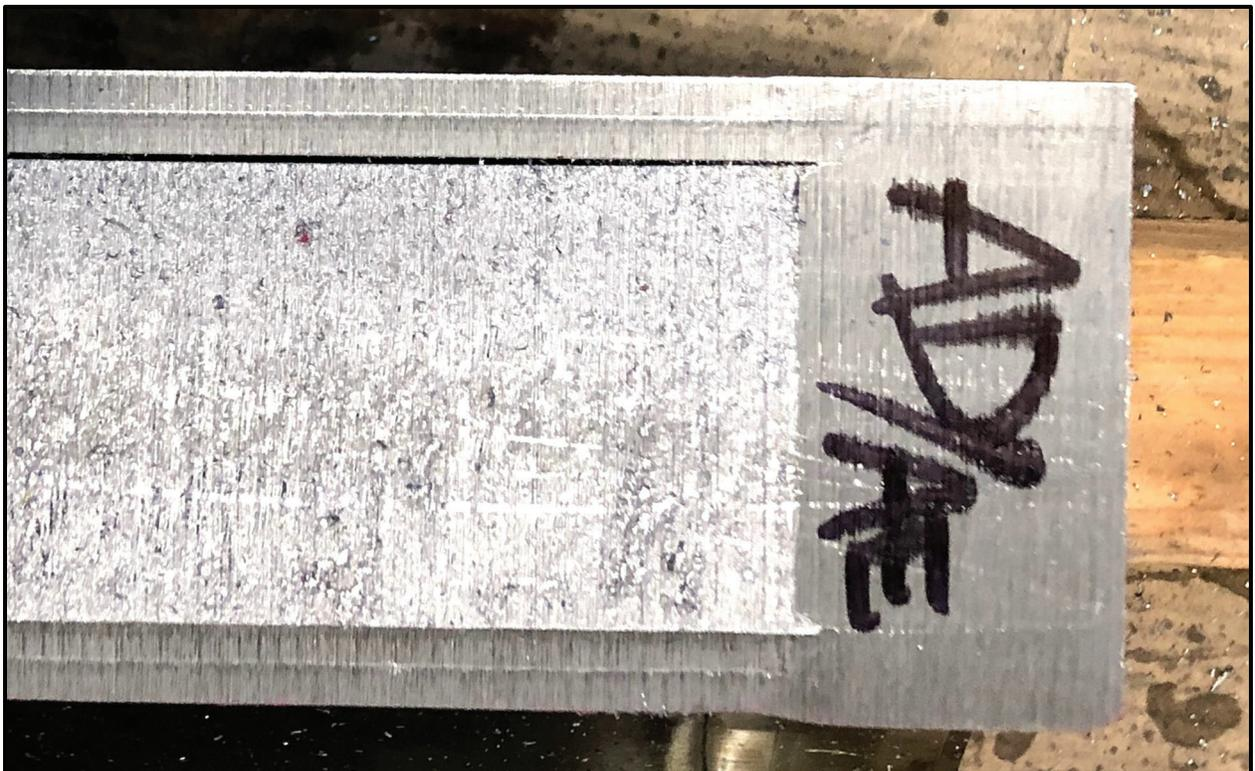
**Figure 6-54** – SC-30G3 18TU-04 Destructive Disassembly Cut AD/AE at Upper Flange
