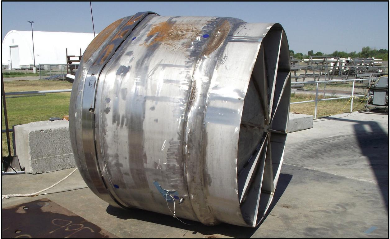
**Figure 6-33** – SC-30G3 Side Drop Radial Flattening of the ICV Shell
