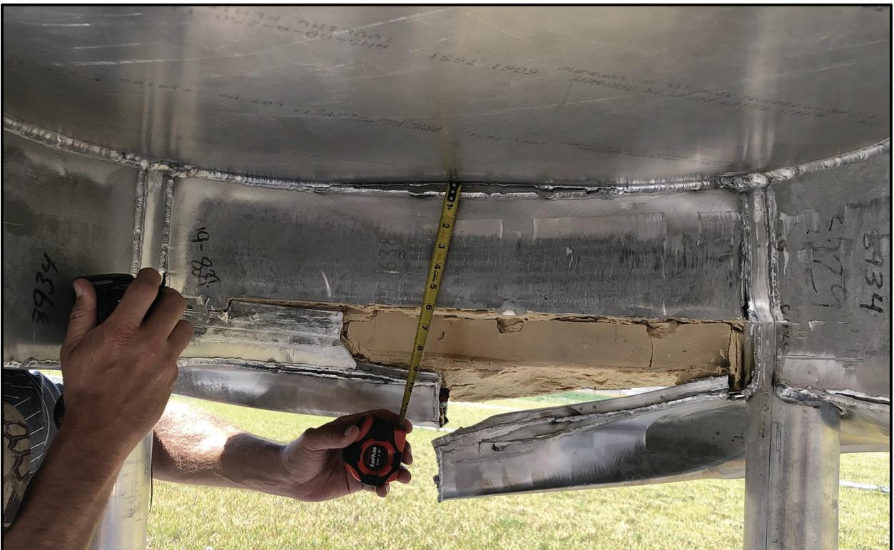
Figure 6-14 – SC-55G1 Radial Dunnage Upper-End Side Drop Damage
