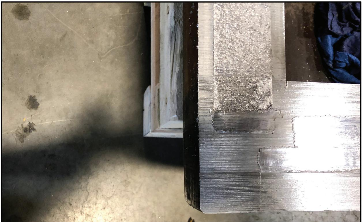
**Figure 7-41** – SC-55G2 18TU-10 Destructive Disassembly Cut E/F at Lower Flange
