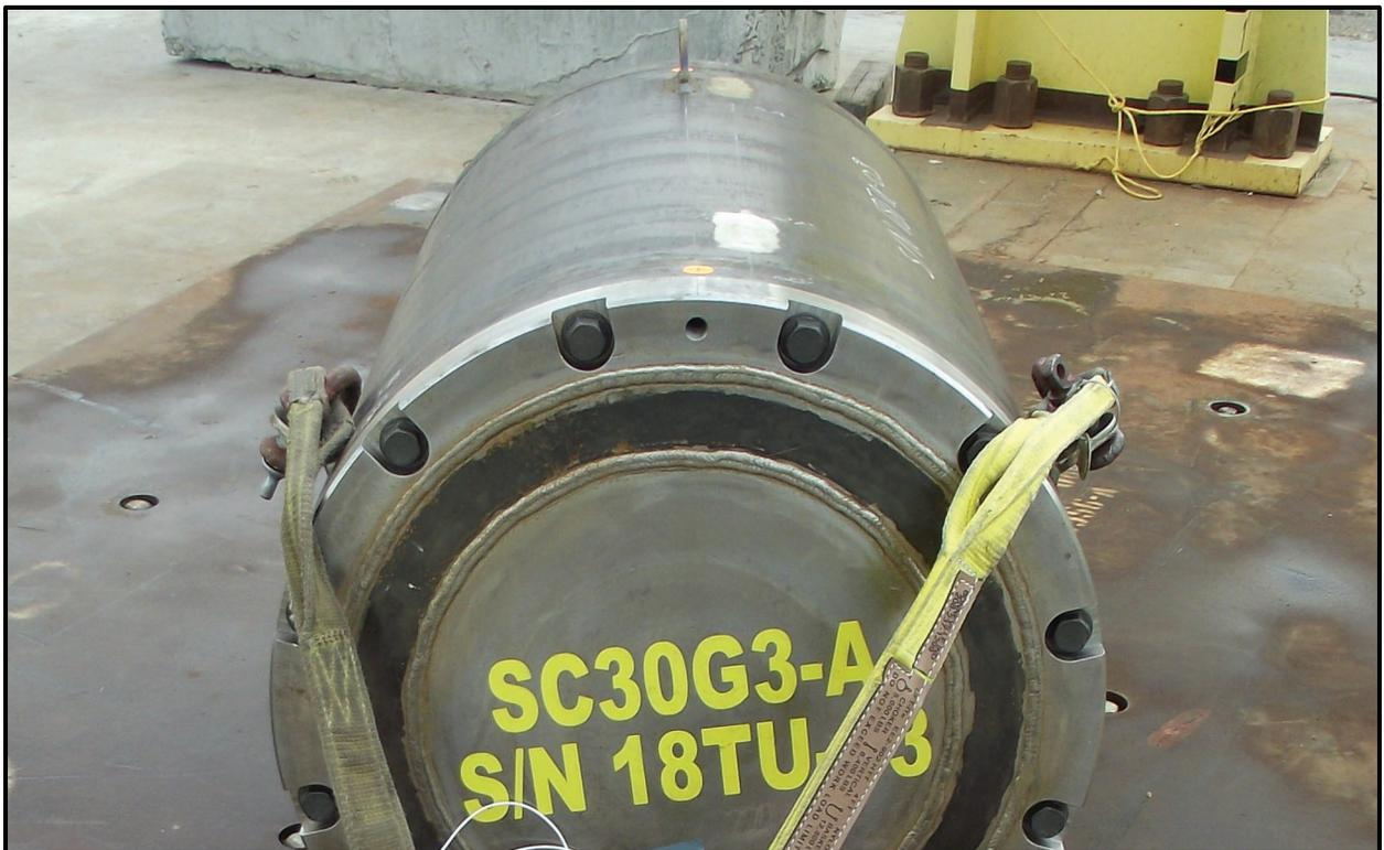
**Figure 6-59** – SC-30G3 18TU-03 Vertical Bottom End Drop Damage 3
