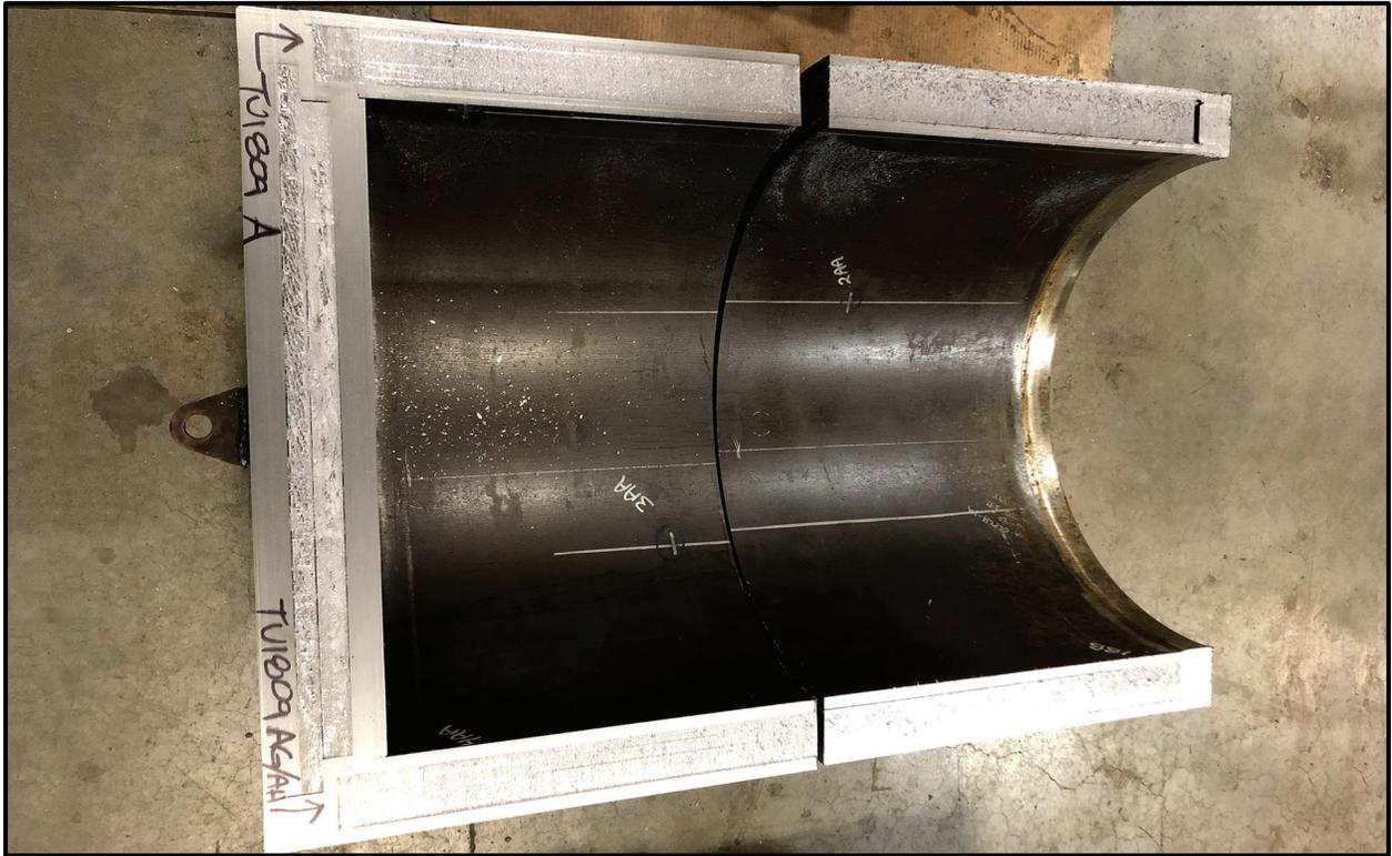
Figure 7-32 – SC-55G2 18TU-09 Destructive Disassembly Overview
