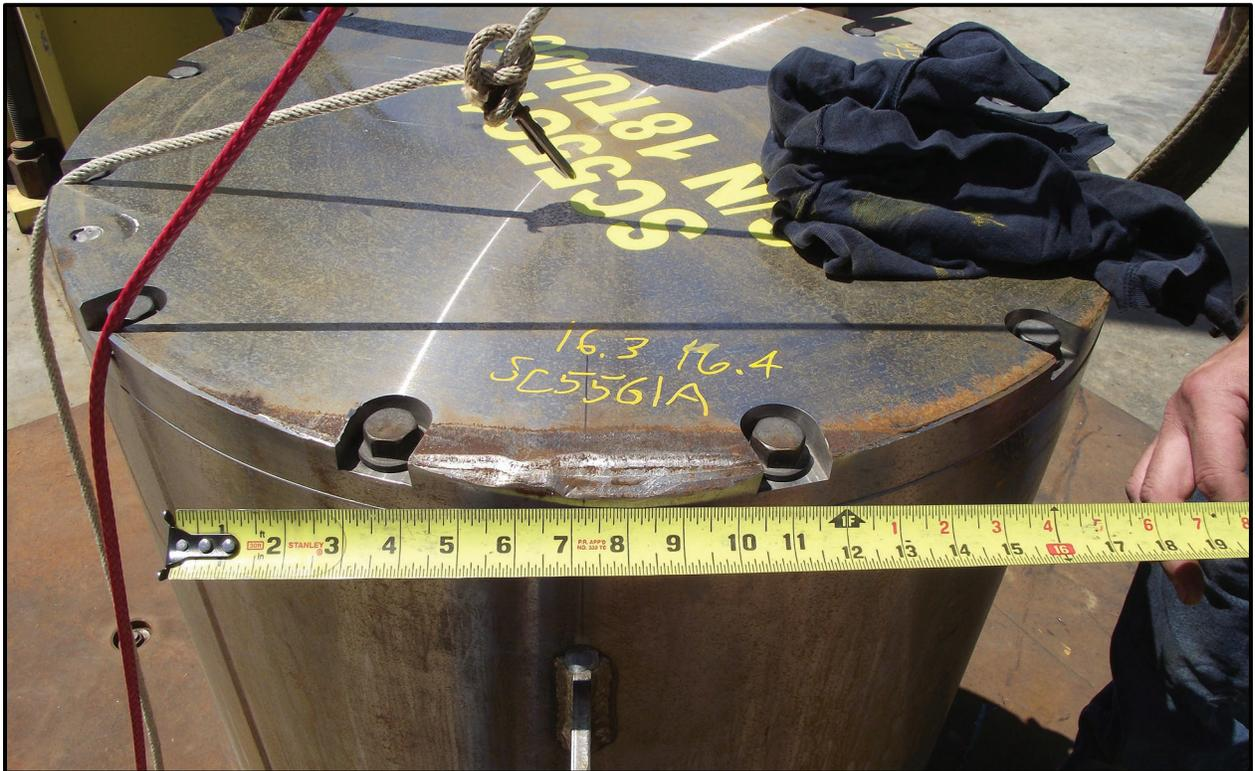
Figure 6-26 – SC-55G1 18TU-06 Top-Down Near-Vertical Drop Damage 1
