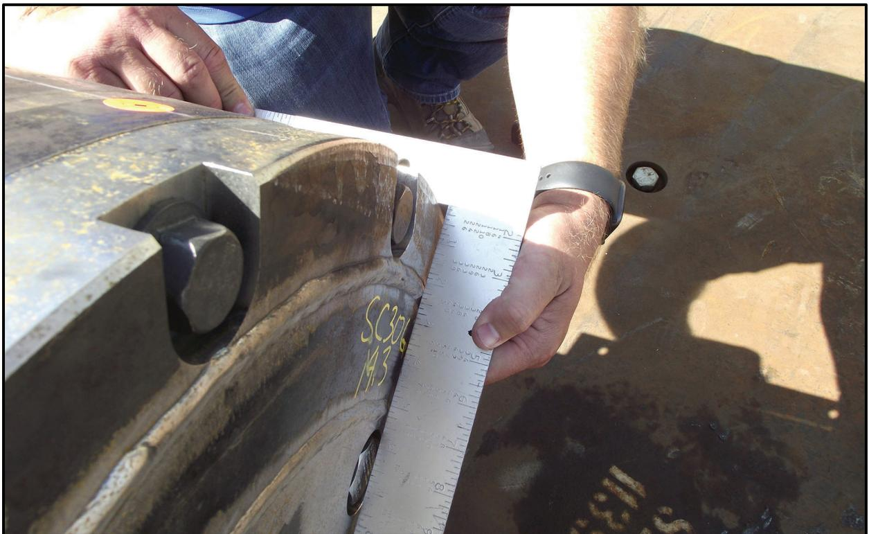
Figure 6-61 – SC-30G3 18TU-05 Top-Down Near-Vertical Drop Damage2
