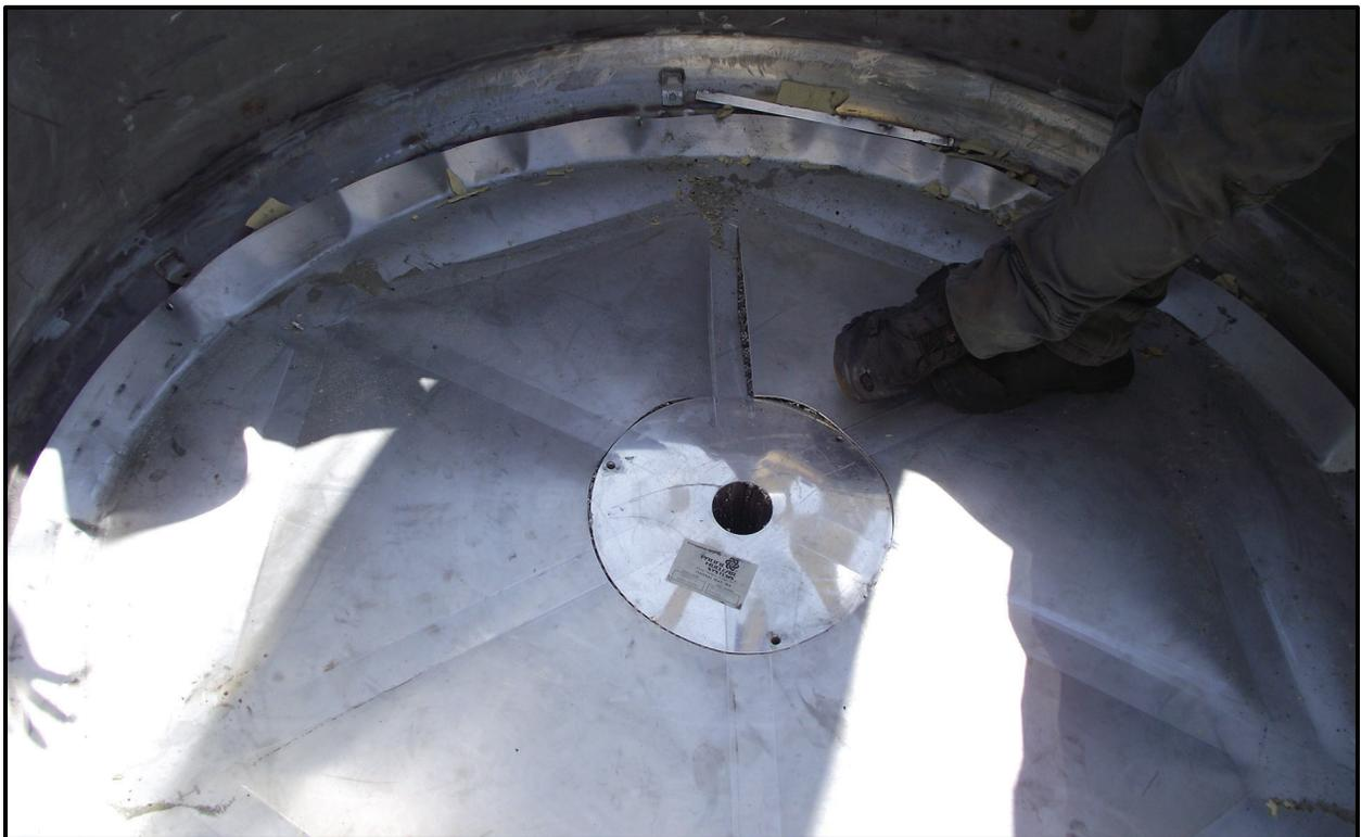
**Figure 6-36** – SC-30G3 Deformed Lower Spacer
