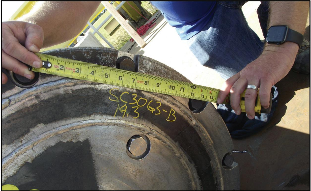
Figure 6-60 – SC-30G3 18TU-05 Top-Down Near-Vertical Drop Damage 1
