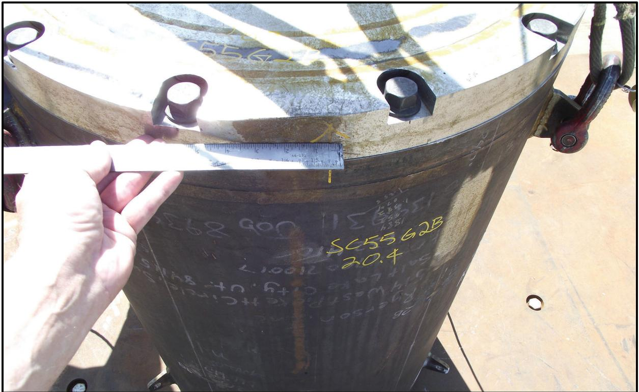
Figure 7-28 – SC-55G2 18TU-10 Horizontal Side Drop Lid-End Damage
