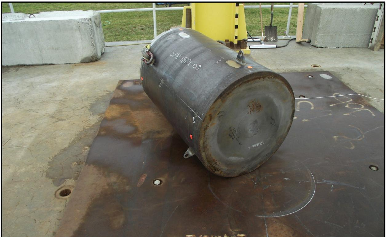
Figure 6-57 – SC-30G3 18TU-03 Vertical Bottom End Drop Damage 1
