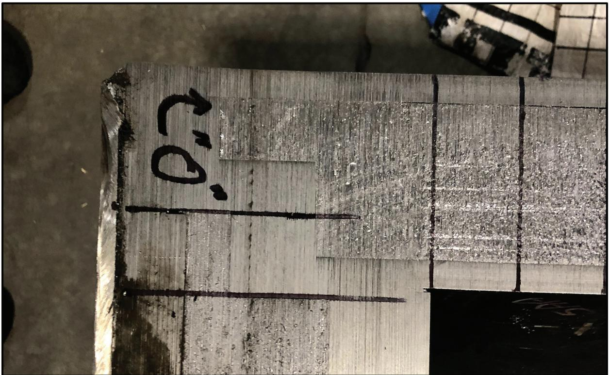
Figure 6-67 – SC-30G3 18TU-05 Destructive Disassembly Cut O at Lower Flange
