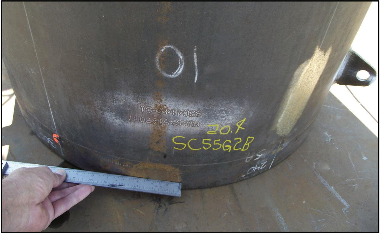
Figure 7-27 – SC-55G2 18TU-10 Horizontal Side Drop Base-End Damage
