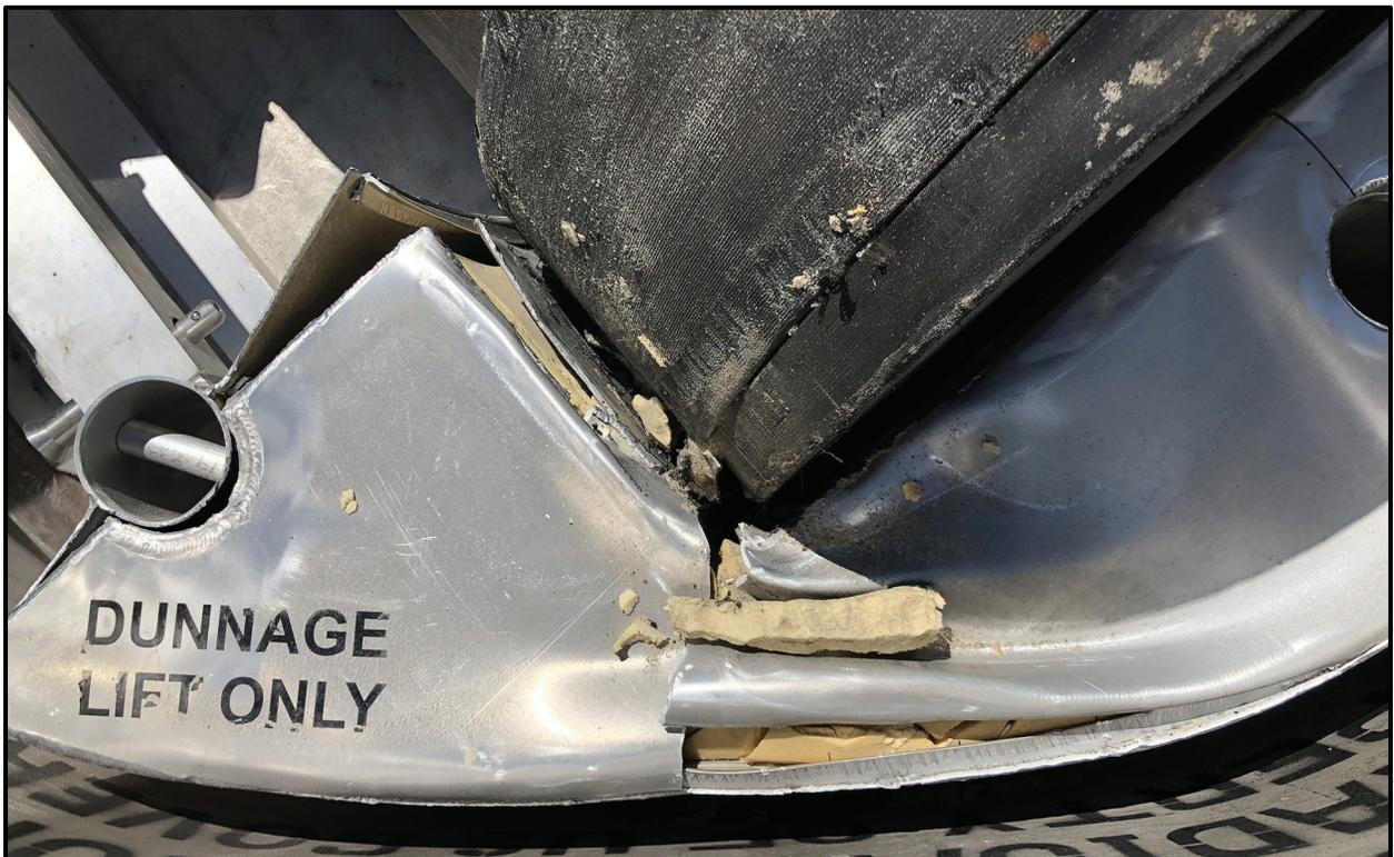
**Figure 6-38** – SC-30G3 Lateral Dunnage Side Drop Damage
