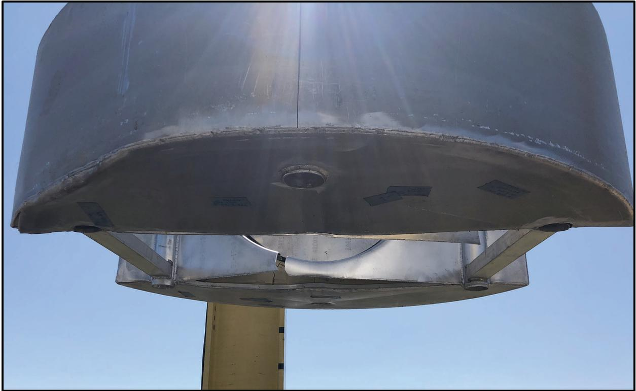
**Figure 6-37** – SC-30G3 Lateral Dunnage End Drop Damage
