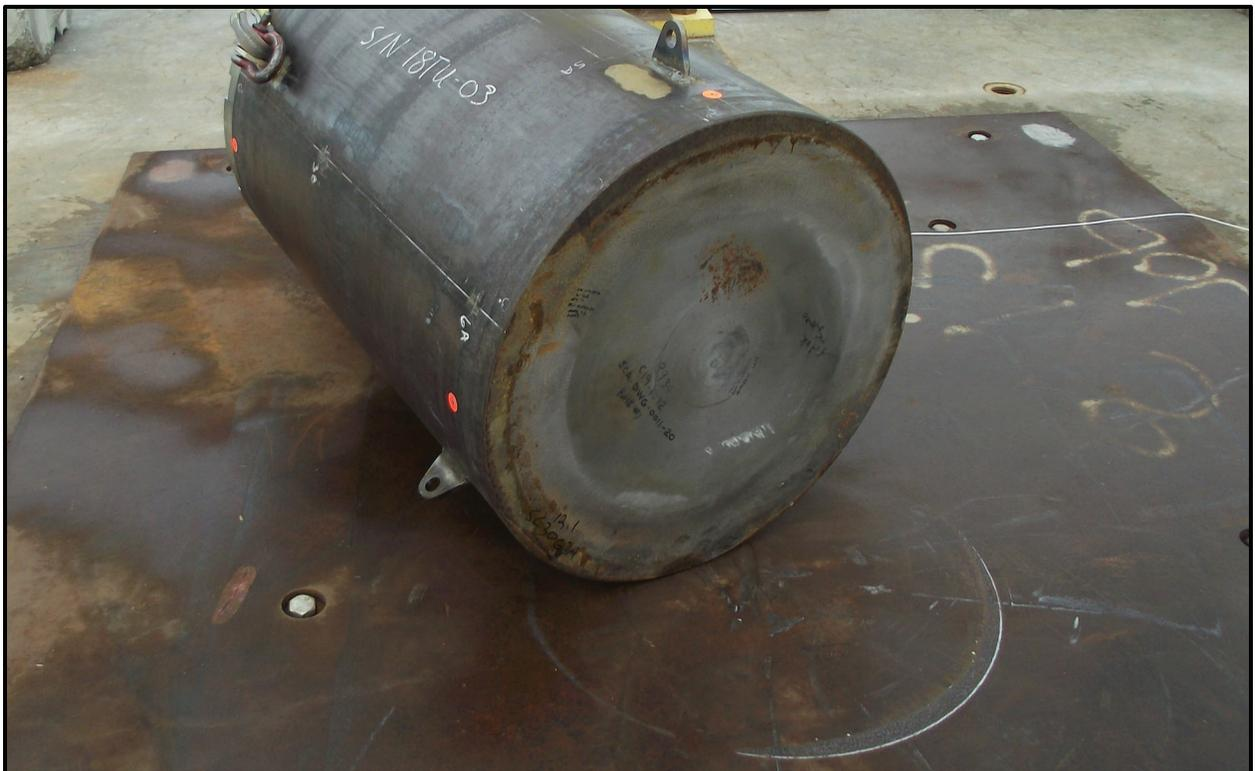
**Figure 7-2 – SC-30G3 18TU-03 DOT-7A Type A 4-foot Vertical End Drop Damage**
