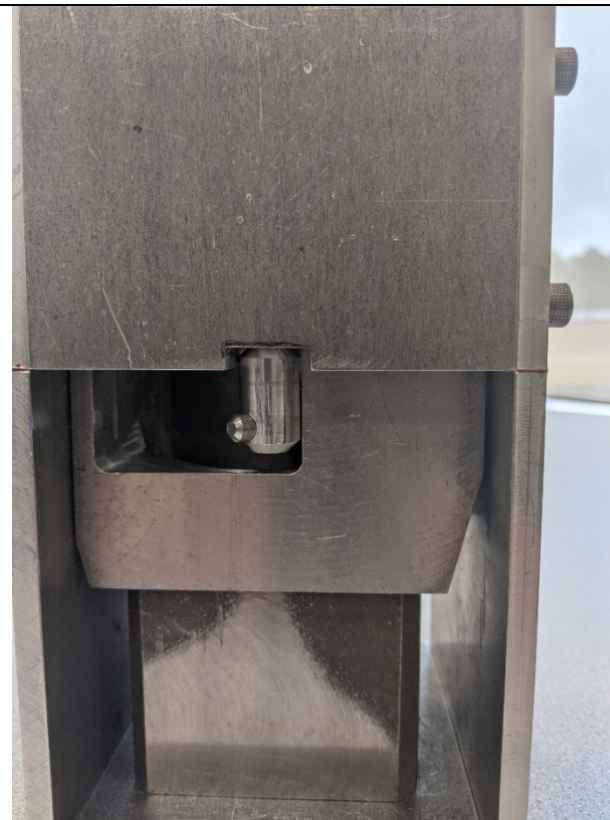
Figure 4. Fuel element head latched into a mockup of the upper grid plate
