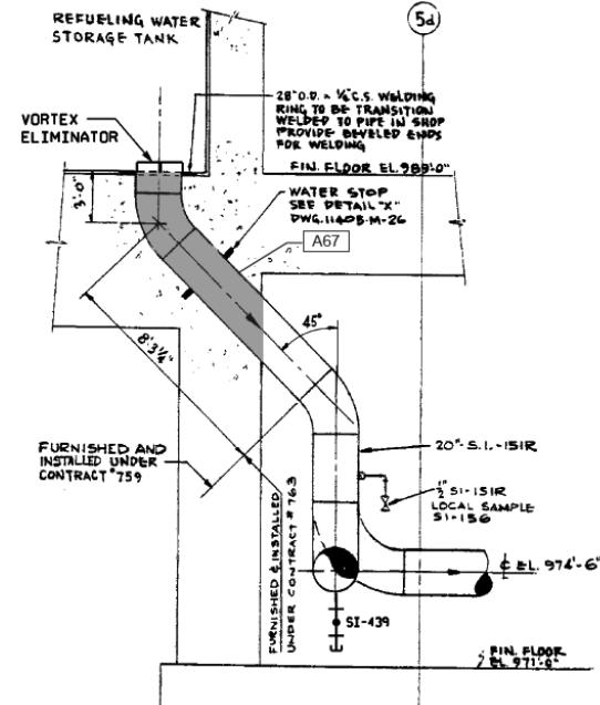
Figure 4 – Section View, 20" SI Piping (10603)
