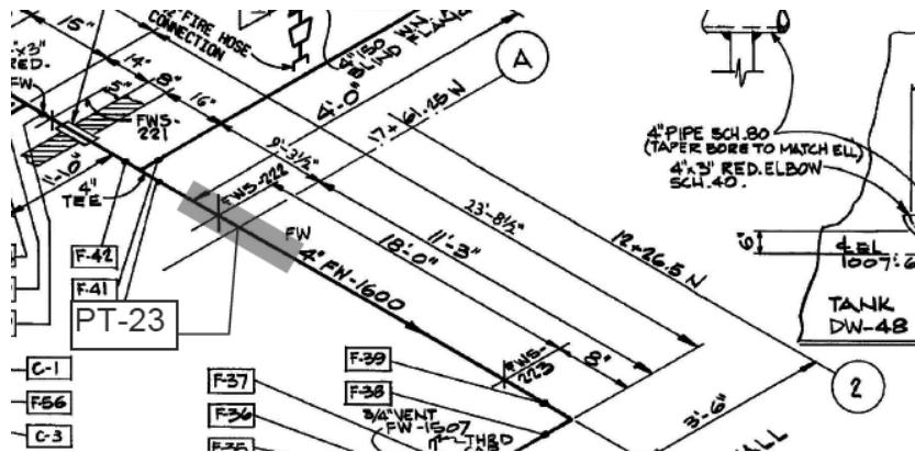
Figure 20 – Recirculation Piping of Feedwater Pump FW-54 (54058)
