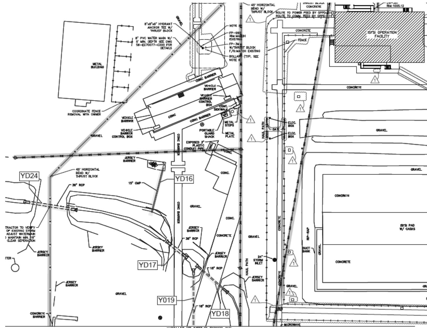
*Figure 7: Yard Drainage – Near ISFSI*
