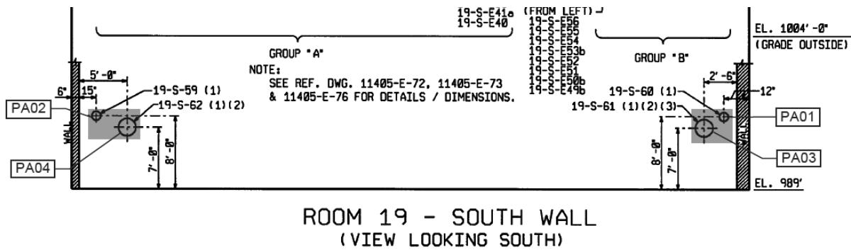
Figure 21 – Aux Bldg Room 19 South Wall Penetrations (60139)
