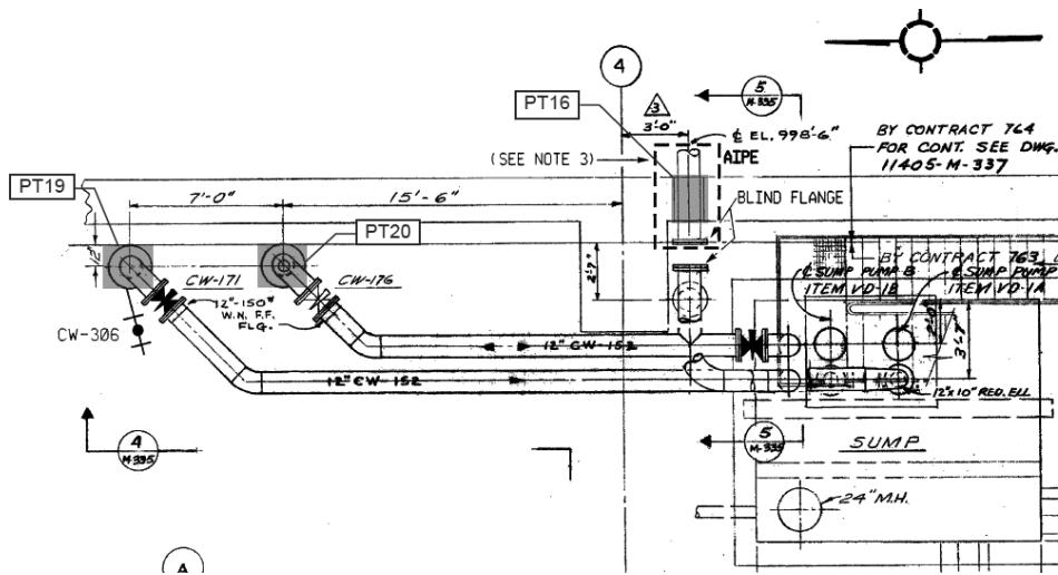
Figure 15 – Sump Pump Discharge Piping (10771)
