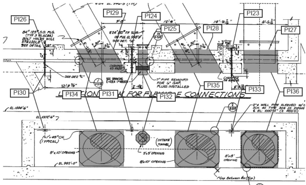
Figure 31 – Penetrations at Intake Tunnel (16539)
