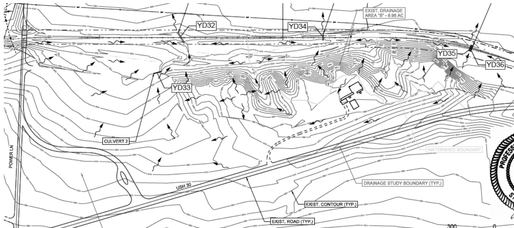
Figure 8: Yard Drainage – Near Waste Processing Tent
