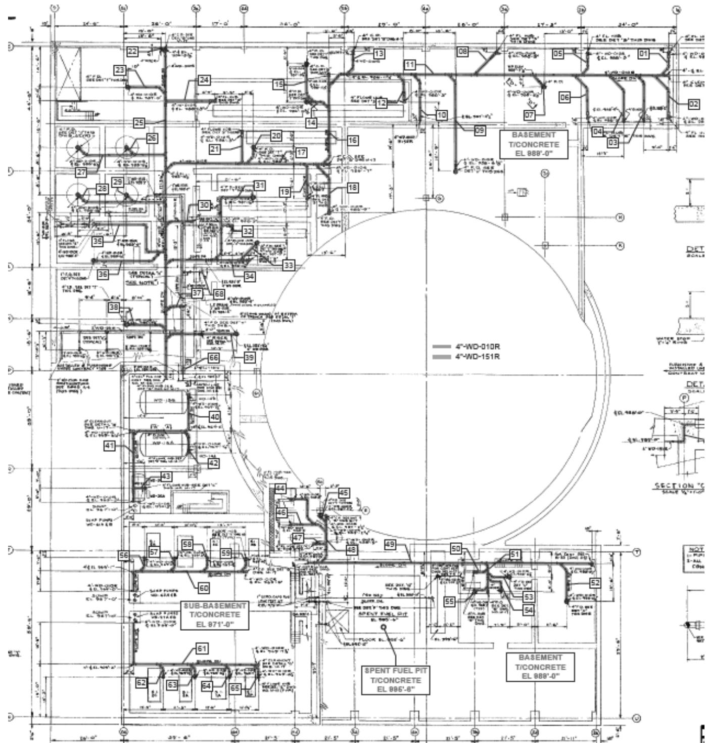
Figure 2 – Embedded Auxiliary Drain Piping to Remain (10592)
