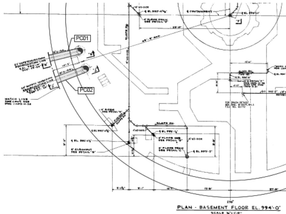
Figure 24 – Safety Injection from Containment to Aux Bldg (10585)
