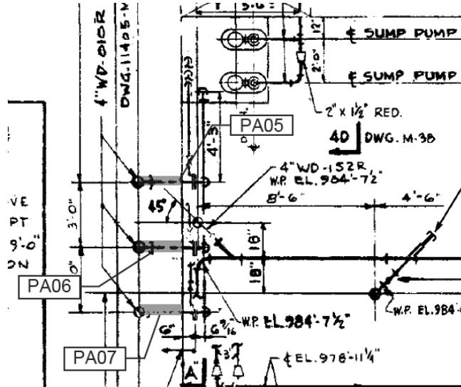
Figure 23 – Sub-basement North Wall Penetrations (10593)
