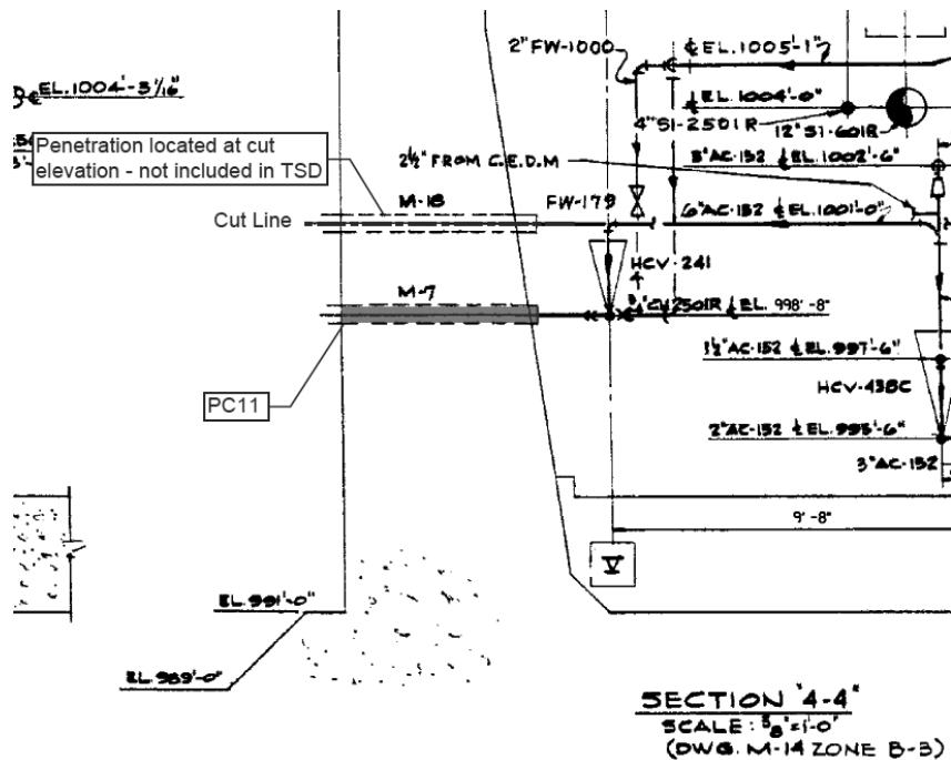
Figure 27 – Containment Wall Penetration Section 4-4 View (10588)
