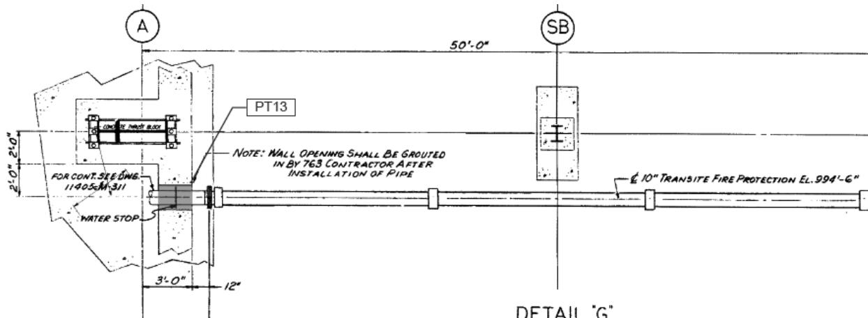
Figure 12 – Fire Protection Penetration at A-Line (10755)
