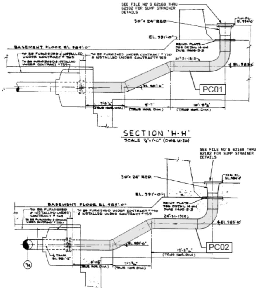
Figure 25 – Safety Injection Section Views (10585)
