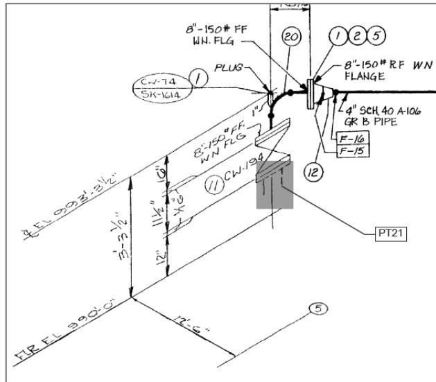
Figure 18 – Circ Water Floor Pen. (35665)
