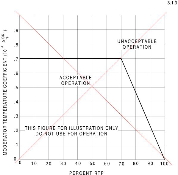
Figure 3.1.3 - 1 (page 1 of 1) Moderator Temperature Coefficient Vs. Rated Thermal Power
