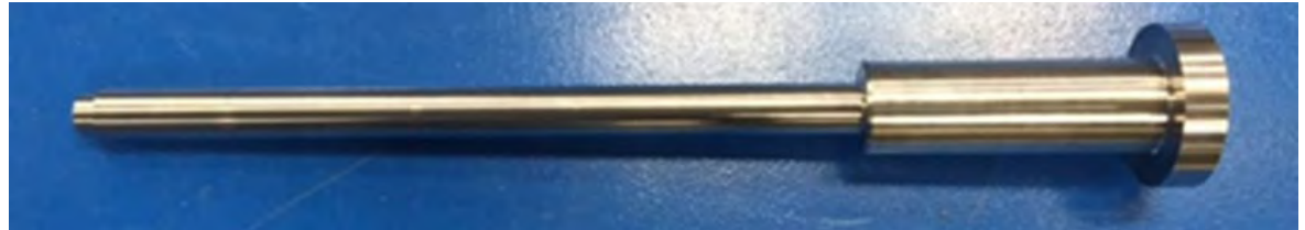
RVI Quickloc Upper Support Assembly Powder Metallurgy and Hot Isostatic Pressing (PM-HIP)
