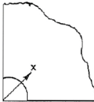
FUN 10 – QUARTER-CIRCULAR CRACK IN QUARTER-SPACE
