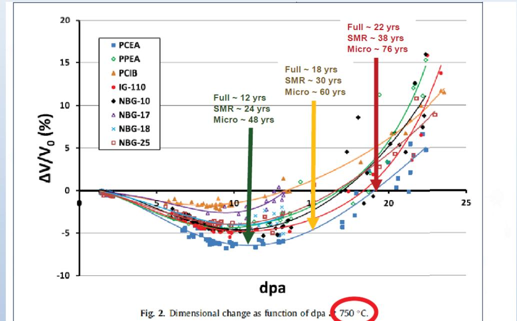
Irradiation significantly alters the graphite behavior - Behavior is completely different before and after “turnaround” dose is achieved.
