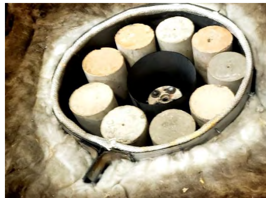
Concrete Heated to 400 to 800 F
