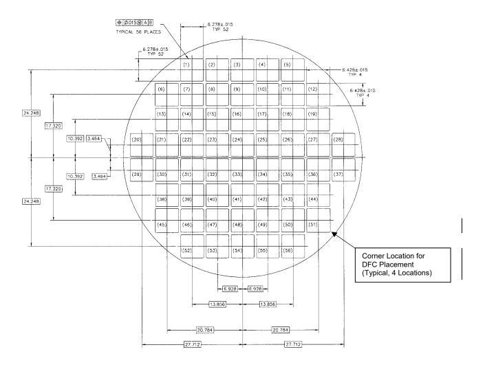
Note: Variations in the dimensions due to fabrication error are permitted provided the minimum flux trap thickness specified in this figure is maintained and no more than two affected (out-of-tolerance) disk openings are adjacent to each other.
