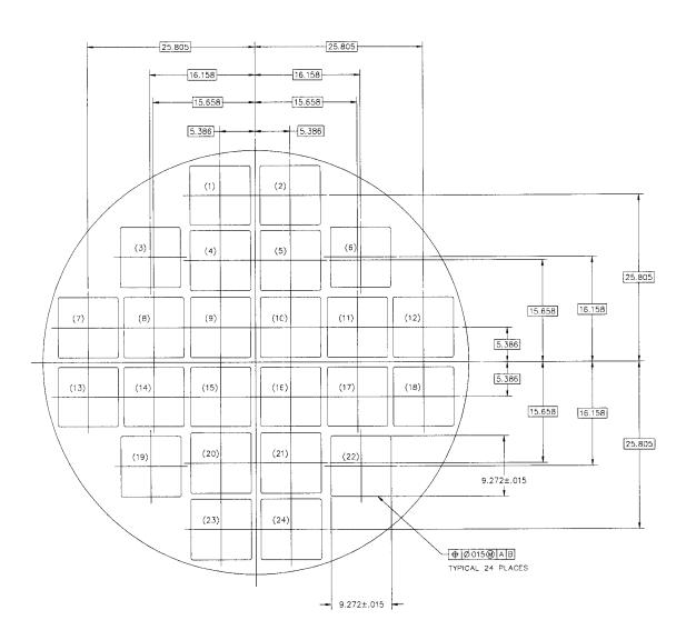
Figure B2-1 PWR Basket Fuel Loading Positions and Minimum Flux Trap Definition
