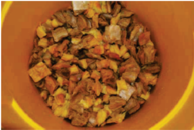
Figure 3.f.4-3: Fine Nukon Fiber Preparation for Head Loss Testing
