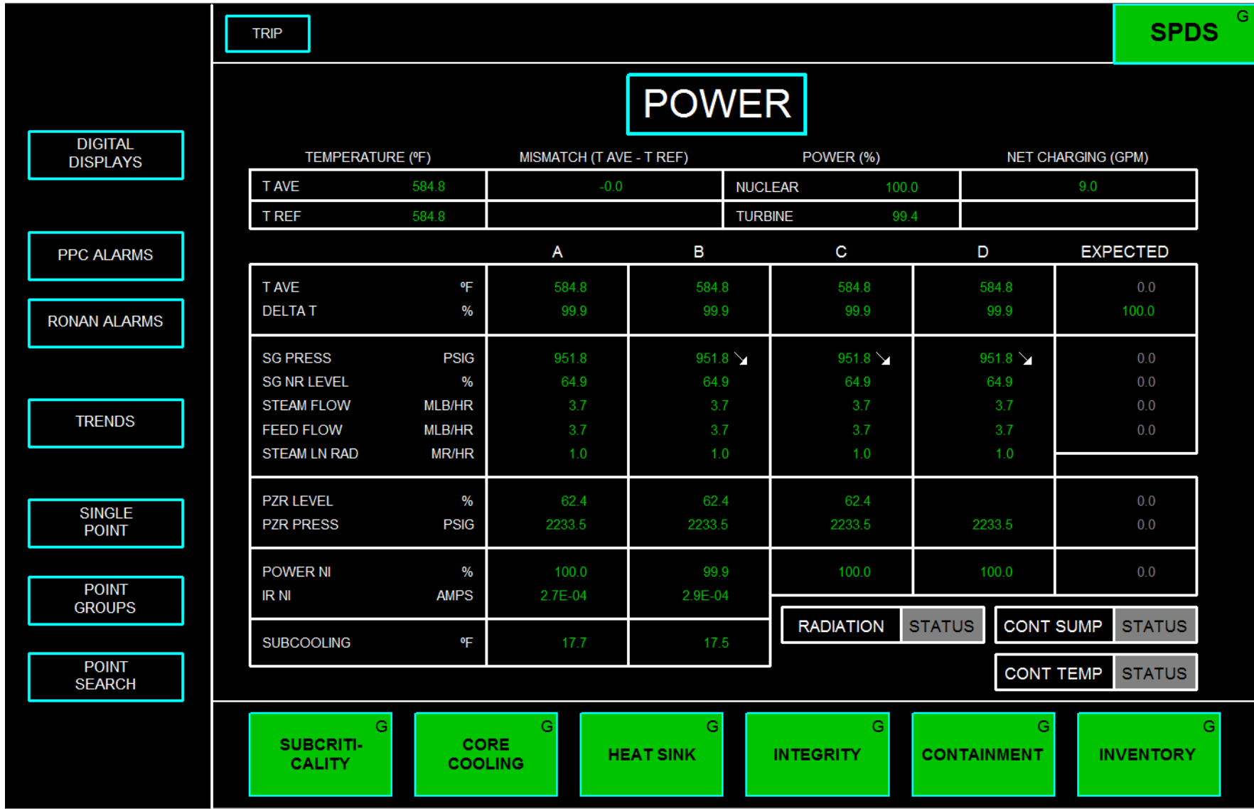
Figure 18-8 SPDS At Power Display
