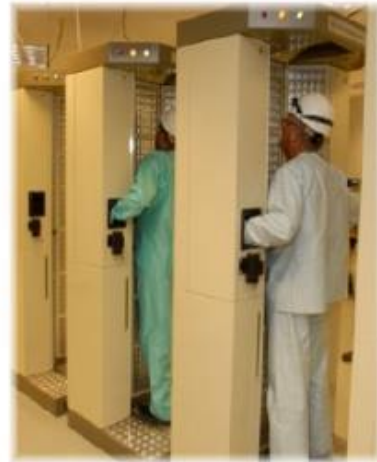
Personnel using one of several types of PCM's. Personnel contamination monitors are the best at detecting contamination. They have very large detectors and are very sensitive.
