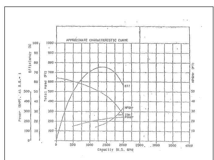
The Curve represents minimum expected performance for replacement parts, and lbr the originally supplied units at the rating point.
