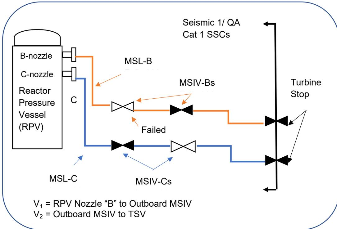
Figure 7: Conceptual MSIV Leakage Model
