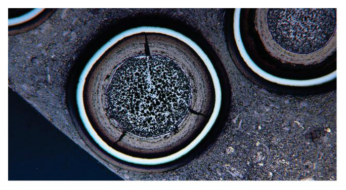
**TRISO** particles cannot melt in a reactor and can withstand extreme temperatures well beyond the threshold of current nuclear fuels.
