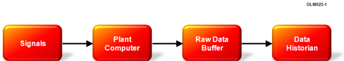
Figure 31: Illustration of sensor data flow
