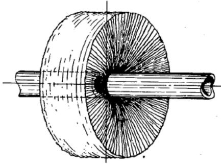
**Figure 2-1: Illustration of a laterally restrained DEGB jet**
