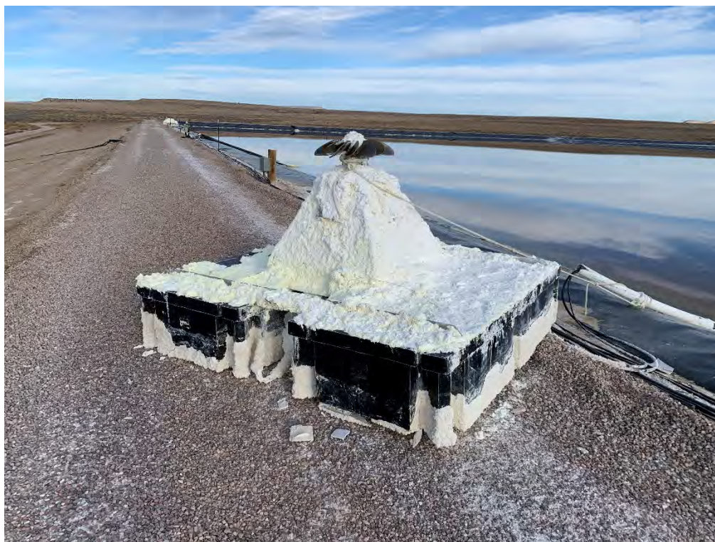
Photo 32: EP-3, evaporator unit pulled out of EP-3 with precipitate buildup
