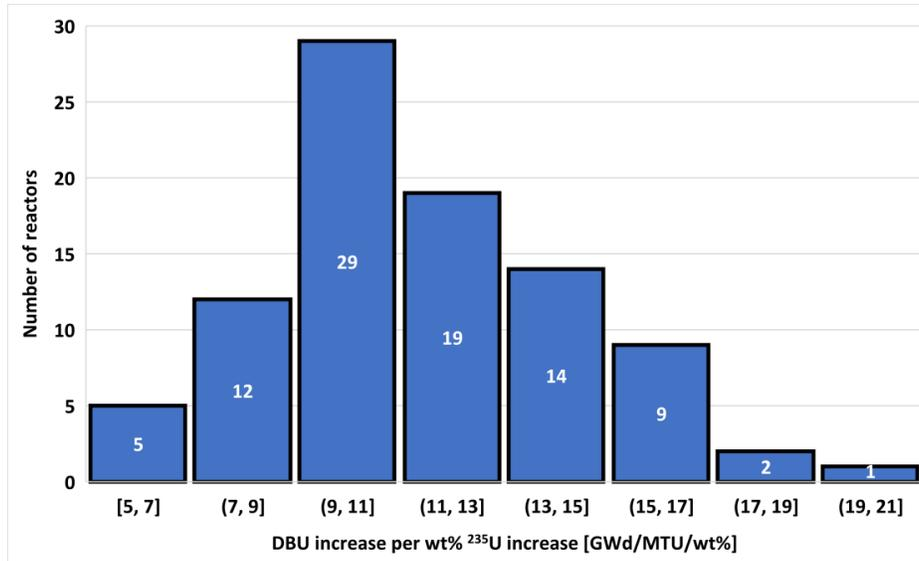
Figure 2. Operating US LWR DBU increase per wt % <sup>235</sup>U.
