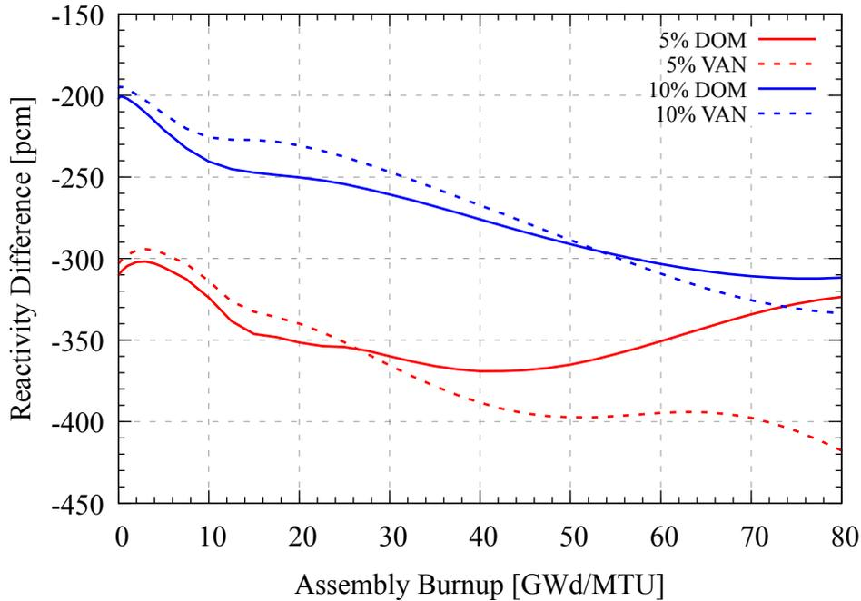
Figure 29. Reactivity difference for Cr-coated BWR ATF.
