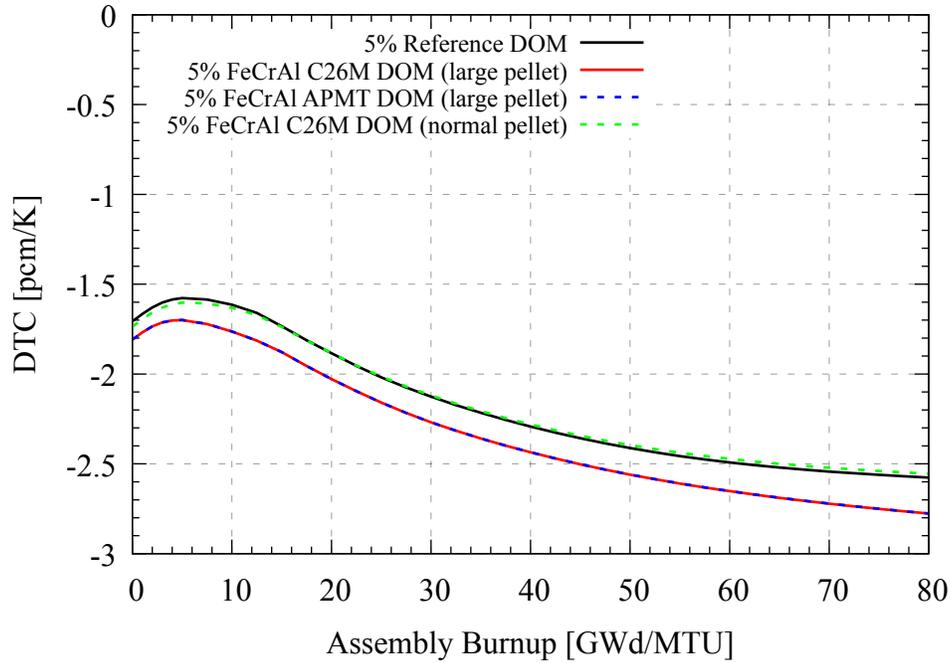
**Figure 37. DTC for 5 wt % limit BWR FeCrAl.**
