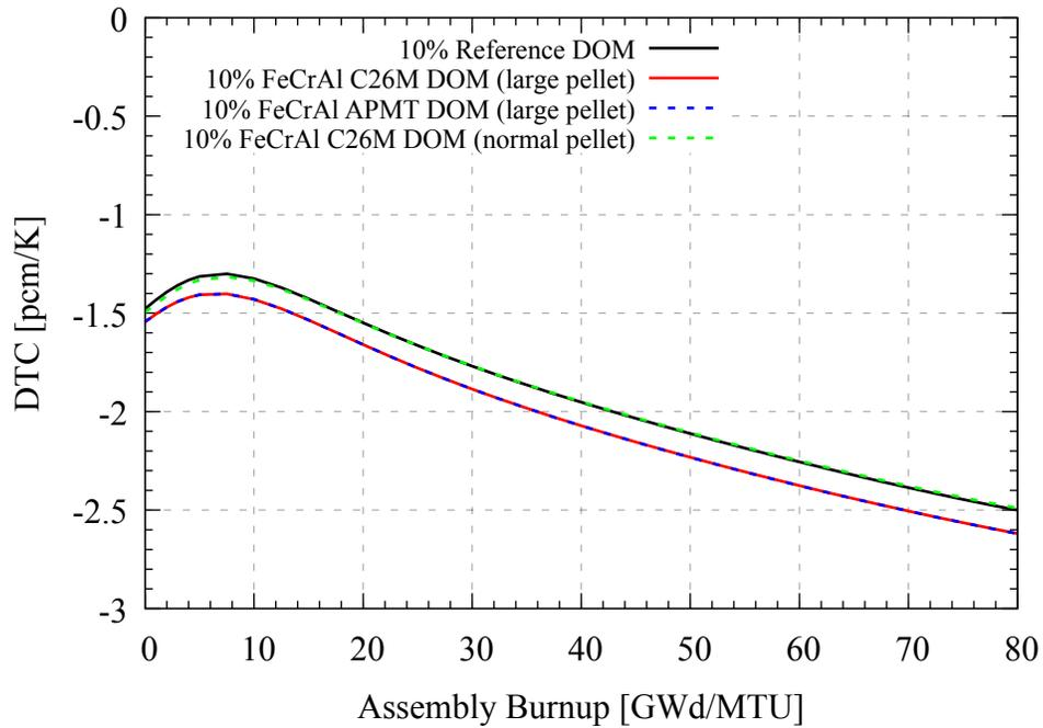
**Figure 38. DTC for 10 wt % limit BWR FeCrAl.**
