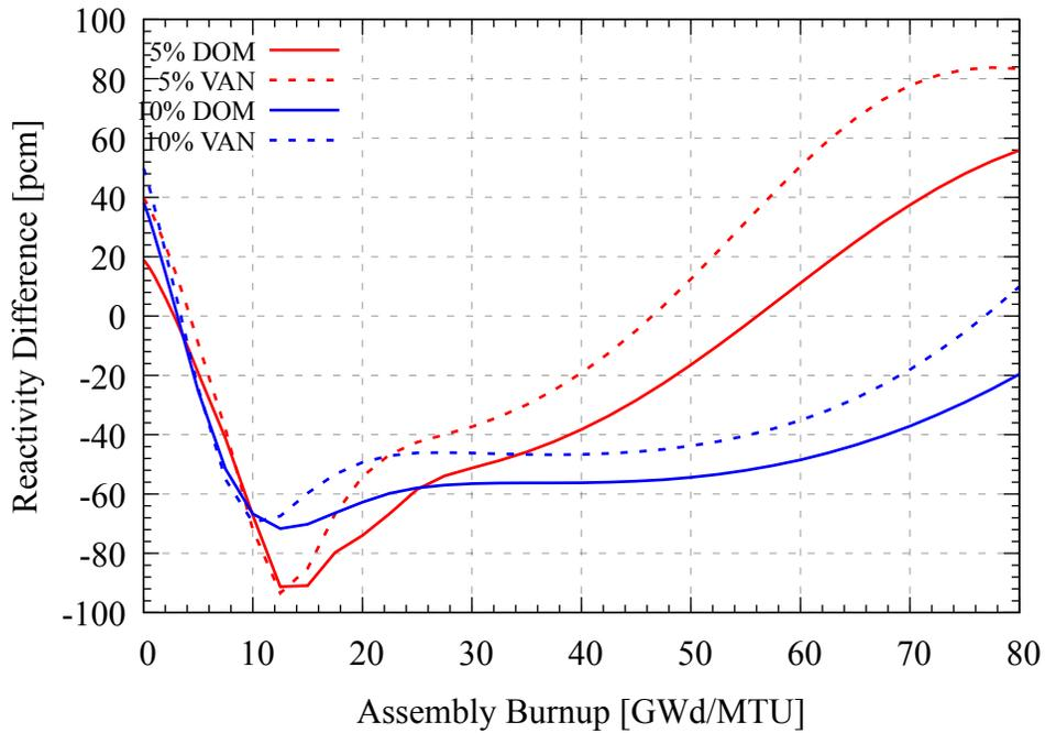
Figure 28. Reactivity difference for doped BWR ATF.
