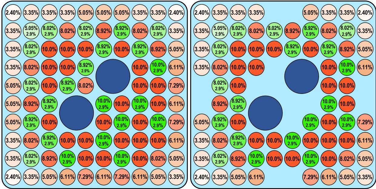
Figure 6. Layout of the 10% maximum enrichment fuel assembly for dominant (left) and vanished (right) regions. The multiplication factor for the reference  $\text{UO}_2$  fuel/Zircaloy-2 cladding simulations at up to 80 GWd/MTU is shown in Figure 7.
