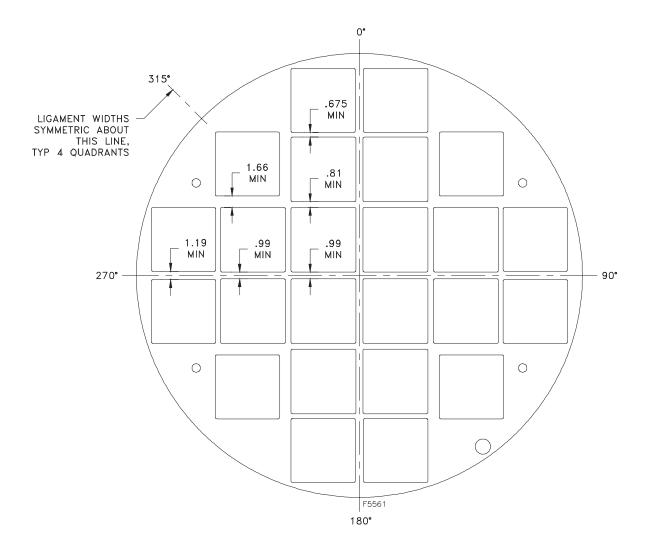
Figure 4-1 Minimum Spacer Disc Ligament Widths
