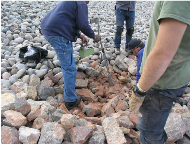
TP5 – Gamma scan of excavation
