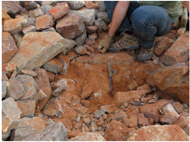
TP5 – Estimated Bottom of Angular Rip Rap
