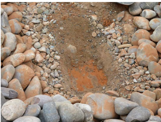
TP3 – Top of Radon Barrier
