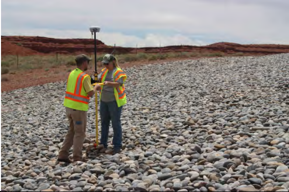
Photo 20. Surveyors gathering data on existing depressions on the northeast side slope of the Mexican Hat Disposal Cell
