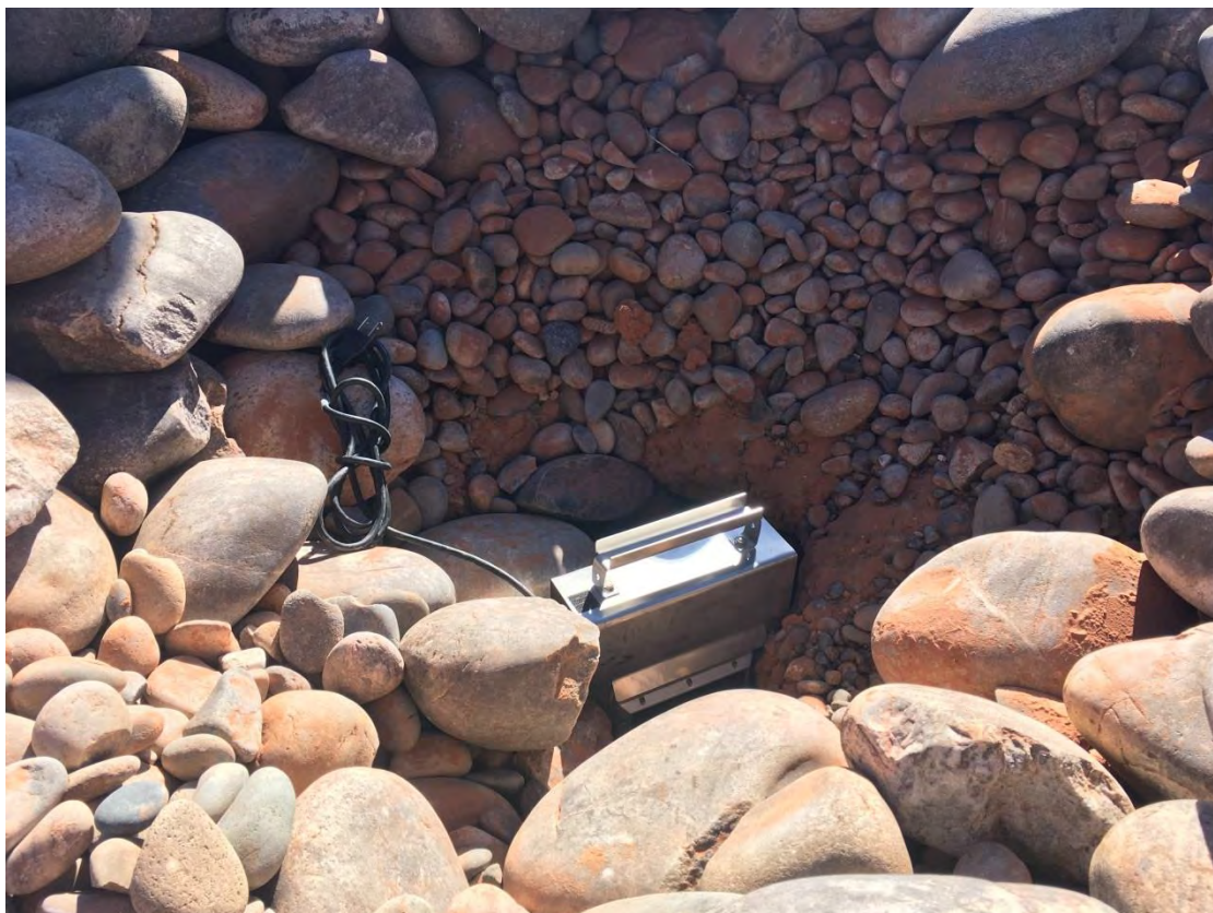
Radiological survey location RSL-4b (re-exposed void) using alphaNUCLEAR Model 597-PX3 radon monitor
