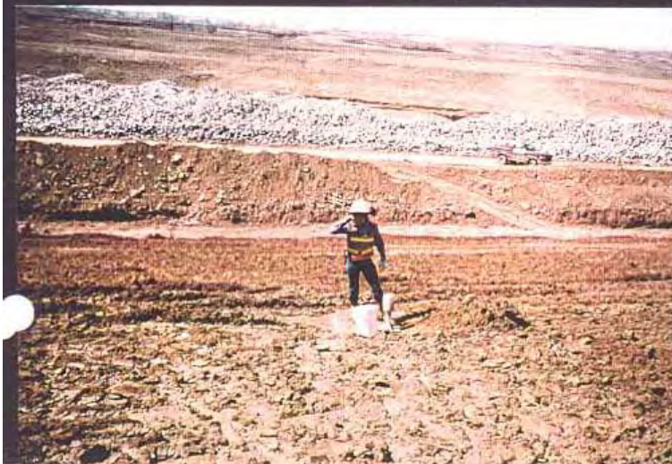
Cell, north 5:1 slope area: QC person, sandcone density test with type C erosion protection material stockpile in background.
