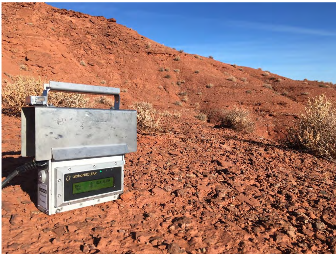
Ongoing collection of radon data at radiological survey location RSL-2 (upwind) using alphaNUCLEAR Model 597-PX3 radon monitor
