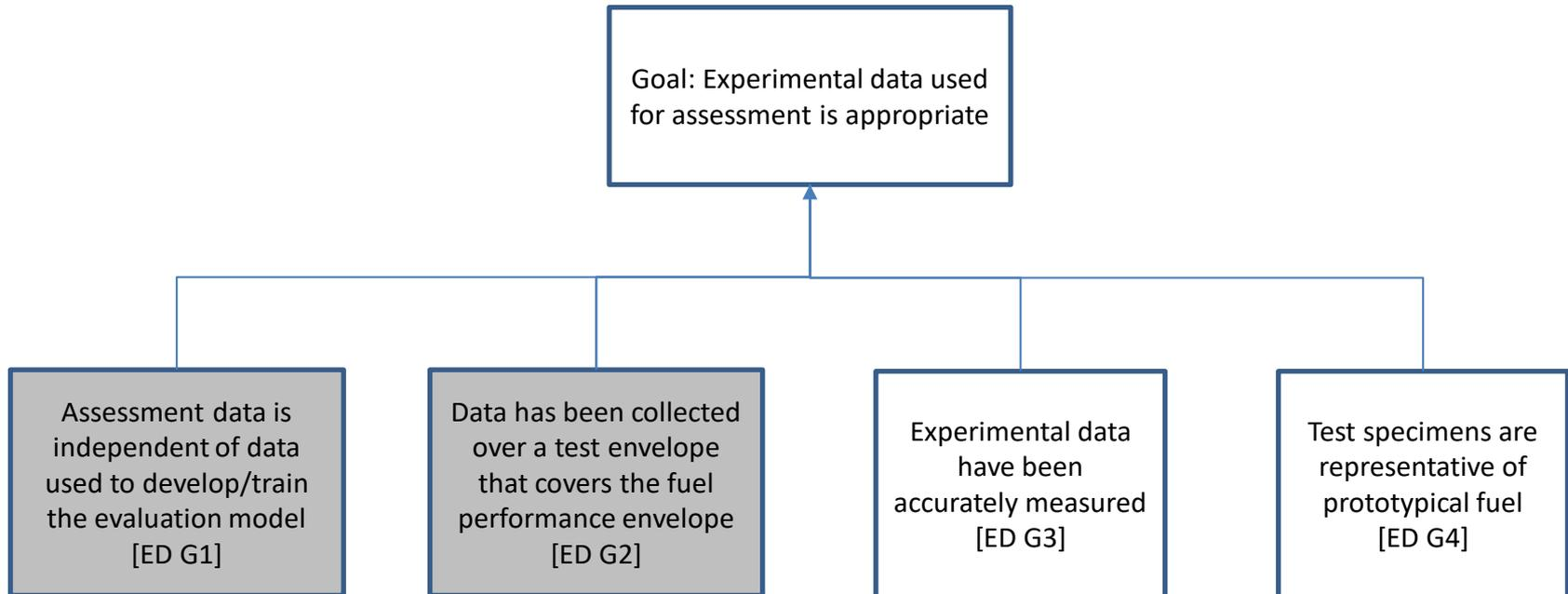
Note: The types of test that should be considered in the test envelope include (1) **steady-state integral testing** of the fuel system in a prototypical environment, (2) **high power and undercooling tests** to address AOO conditions and to assess design margin, (3) **power ramp testing** to assess fuel performance during anticipated power changes, and (4) **design basis accident tests** to establish margin to fuel breach and contribution to source term under accident conditions
