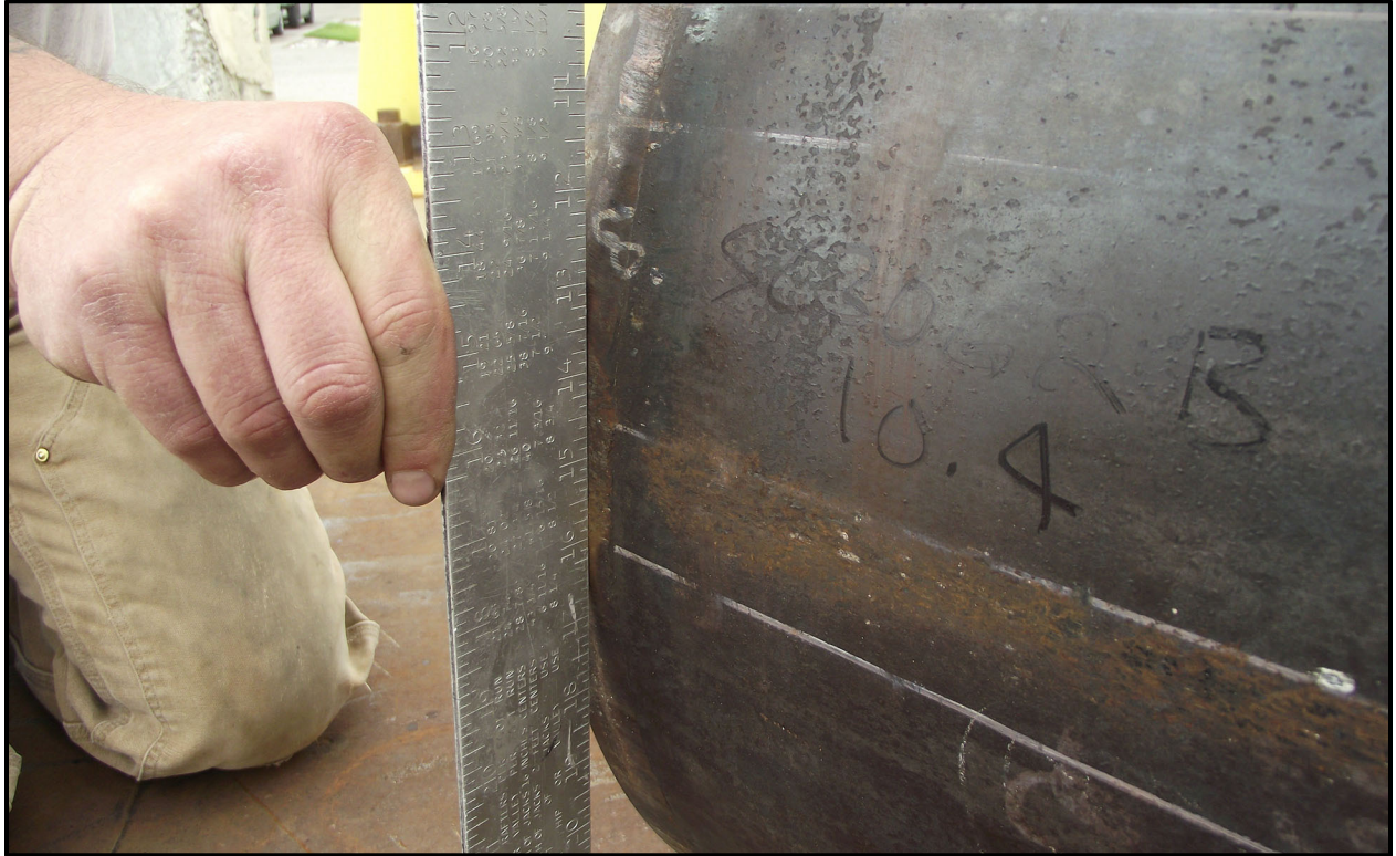
Figure 7-3 – SC-30G2 18TU-02 Horizontal Side Drop Base-End Damage
