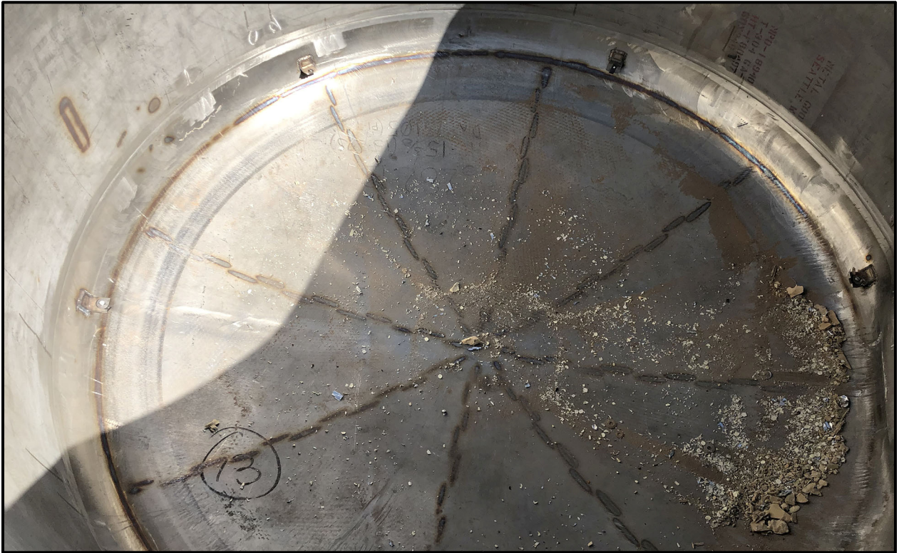
Figure 6-19 – SC-55G1 ICV with No Visible End Drop Interaction from SC-55G1s
