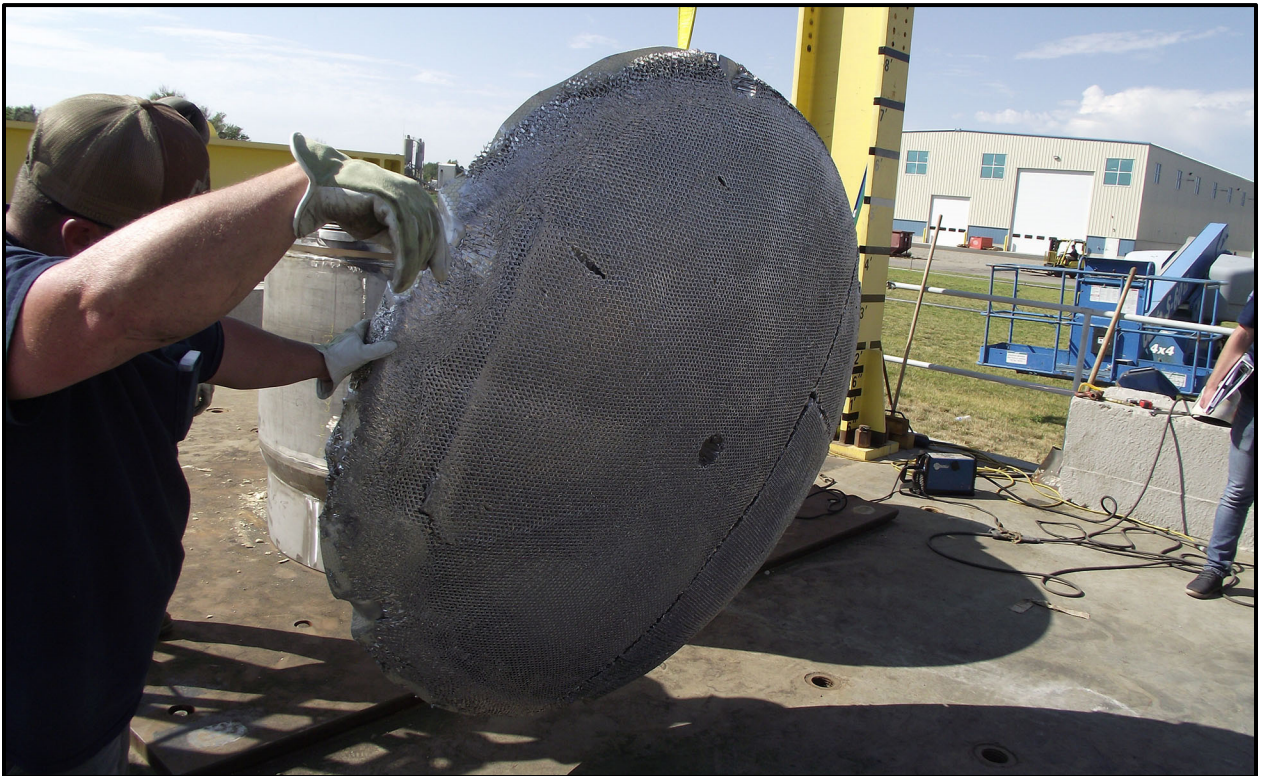
Figure 6-12 – Deformed Lower Spacer (Bottom-View)
