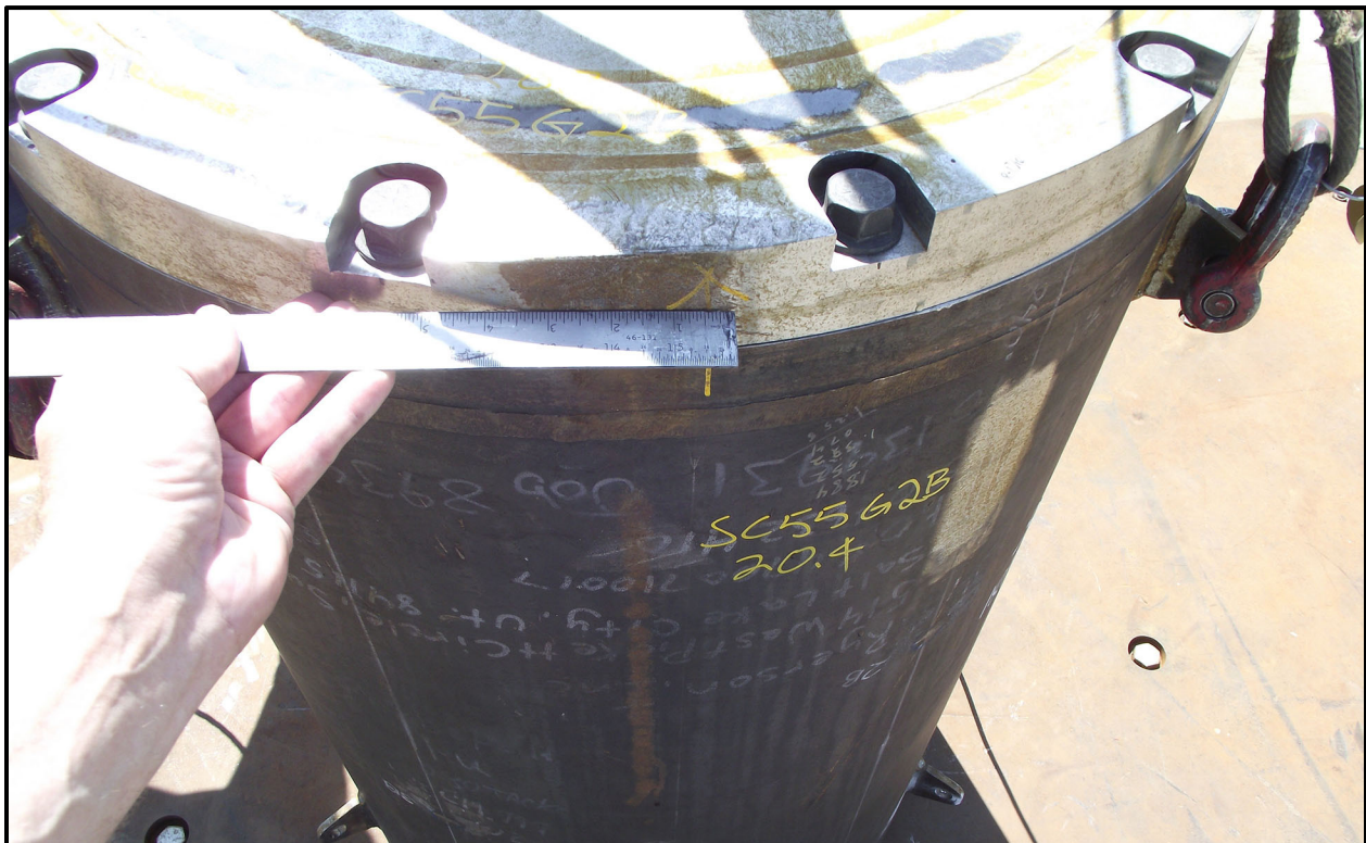
Figure 7-24 – SC-55G2 18TU-10 Horizontal Side Drop Lid-End Damage
