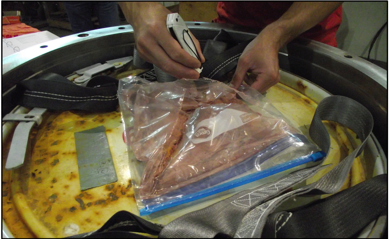
Figure 6-1 – Installing and Cutting the Fluorescein Dye Bags
