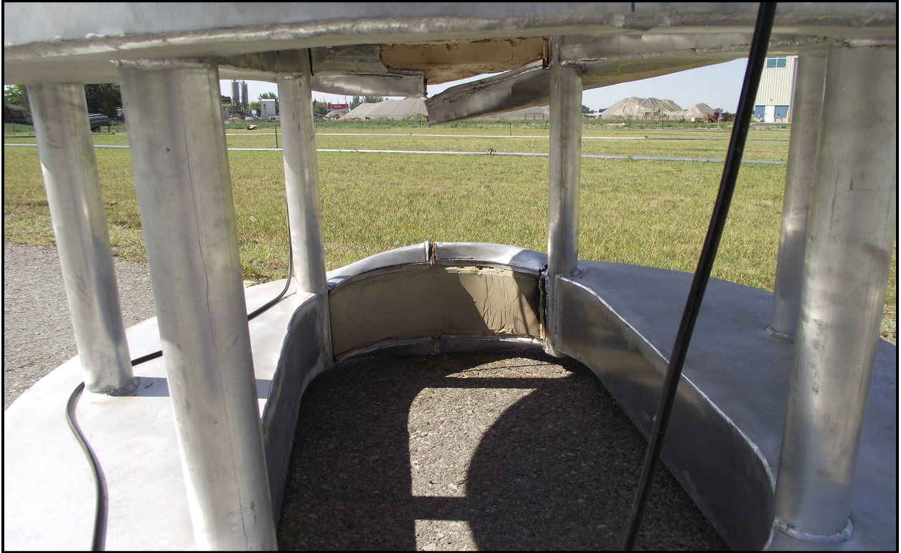
Figure 6-13 – SC-55G1 Radial Dunnage Side Drop Damage
