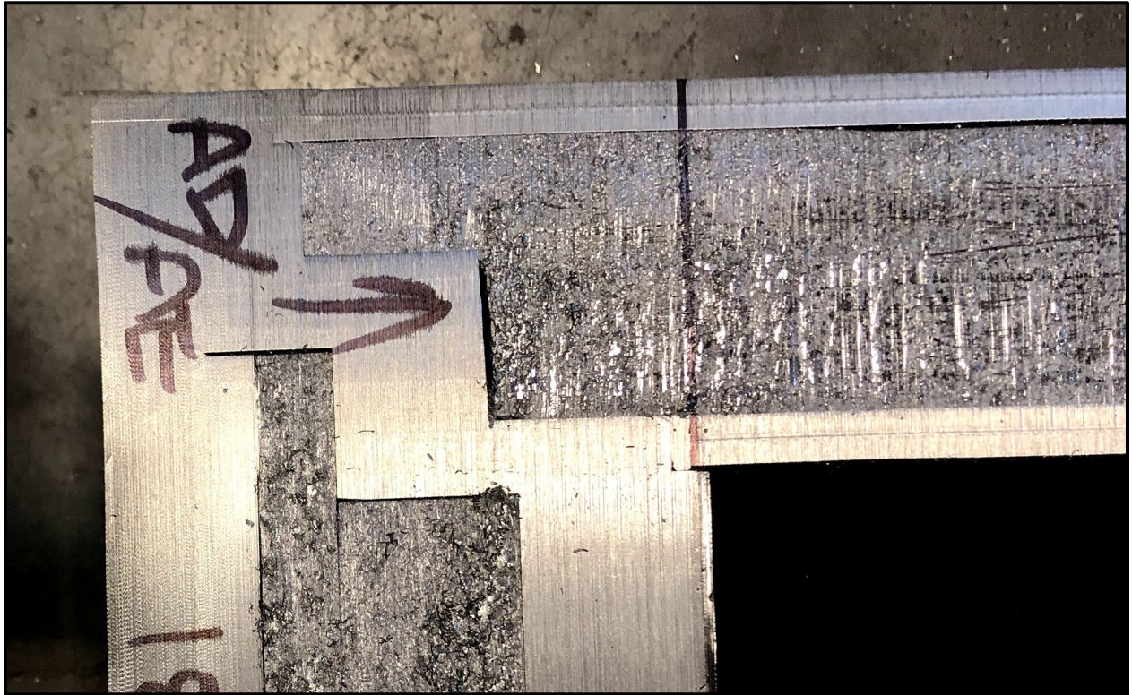
Figure 6-48 – SC-30G3 18TU-04 Destructive Disassembly Cut AD/AE at Lower Flange
