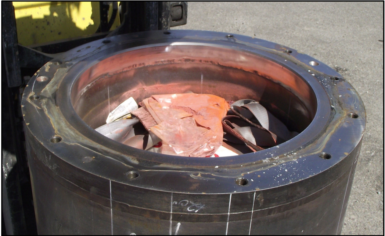
Figure 6-38 – Fluorescein Dye inside the SC-30G3 Body
