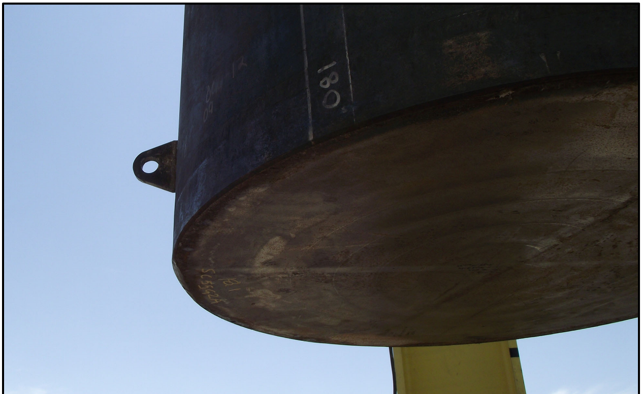
Figure 7-22 – SC-55G2 18TU-09 Vertical End Drop Damage
