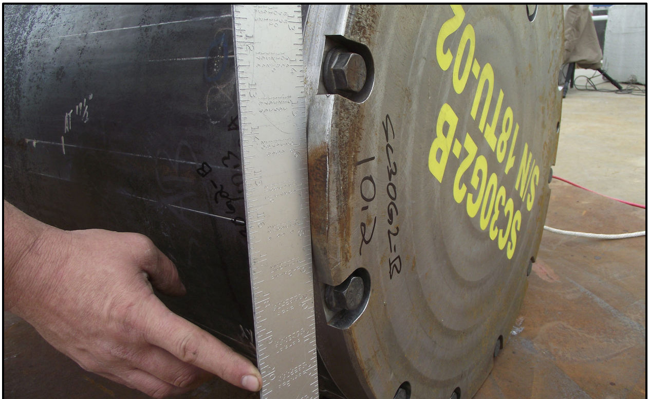
Figure 7-4 – SC-30G2 18TU-02 Horizontal Side Drop Lid-End Damage
