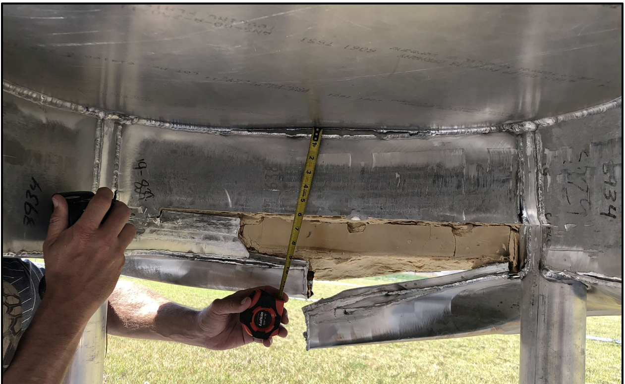
Figure 6-14 – SC-55G1 Radial Dunnage Upper-End Side Drop Damage
