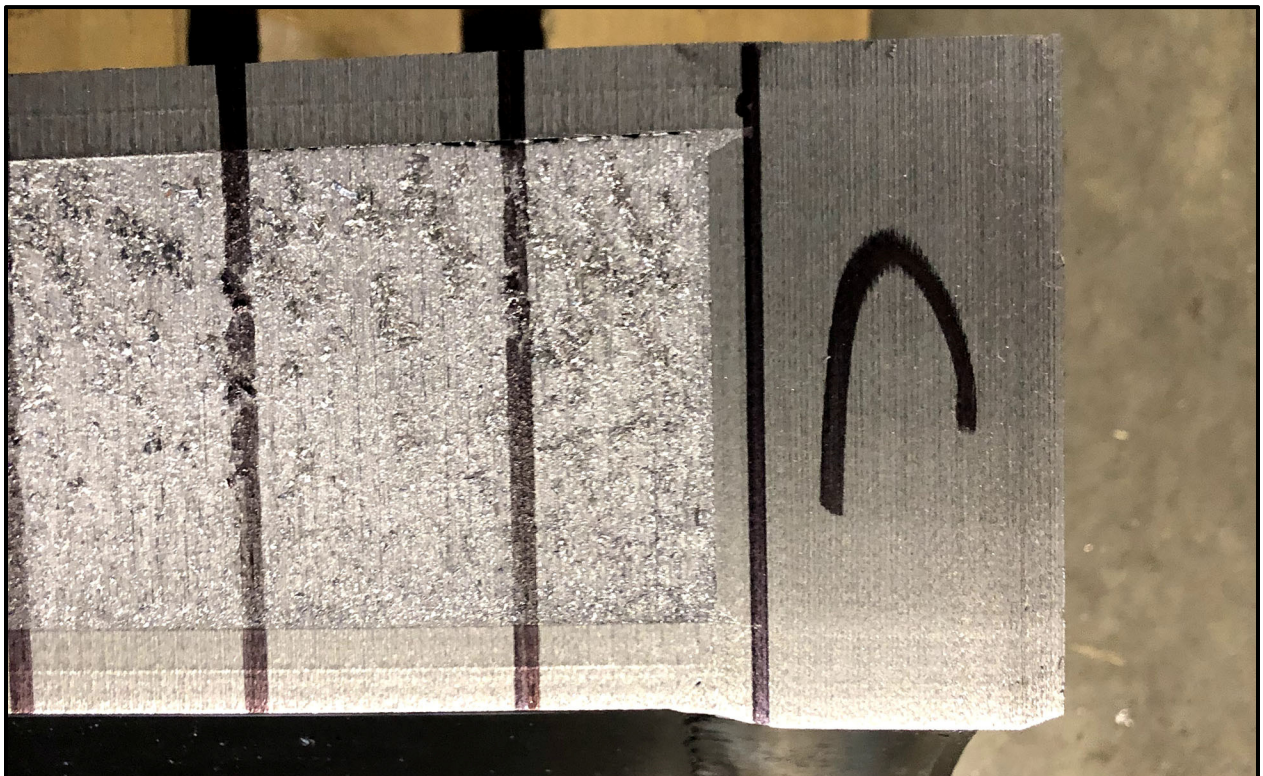
Figure 6-45 – SC-30G3 18TU-04 Destructive Disassembly Cut C at Upper Flange
