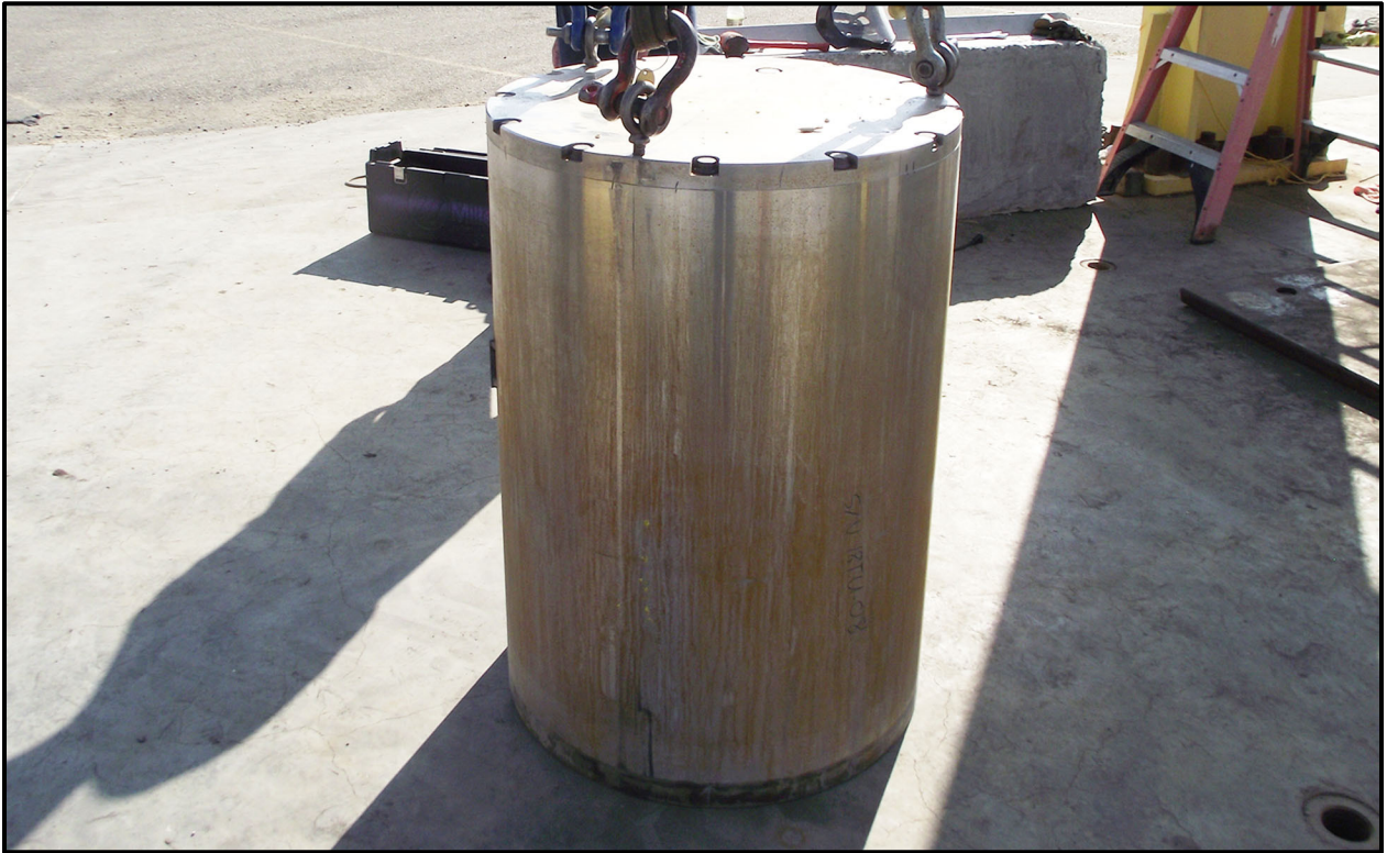
Figure 6-17 – SC-55G1 18TU-08 Superficial Sidewall Damage (Lower in Side Drop)
