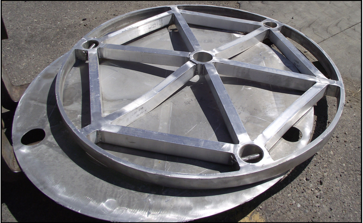
Figure 6-30 – SC-30G3 Deformed Heavy-Duty Pallet
