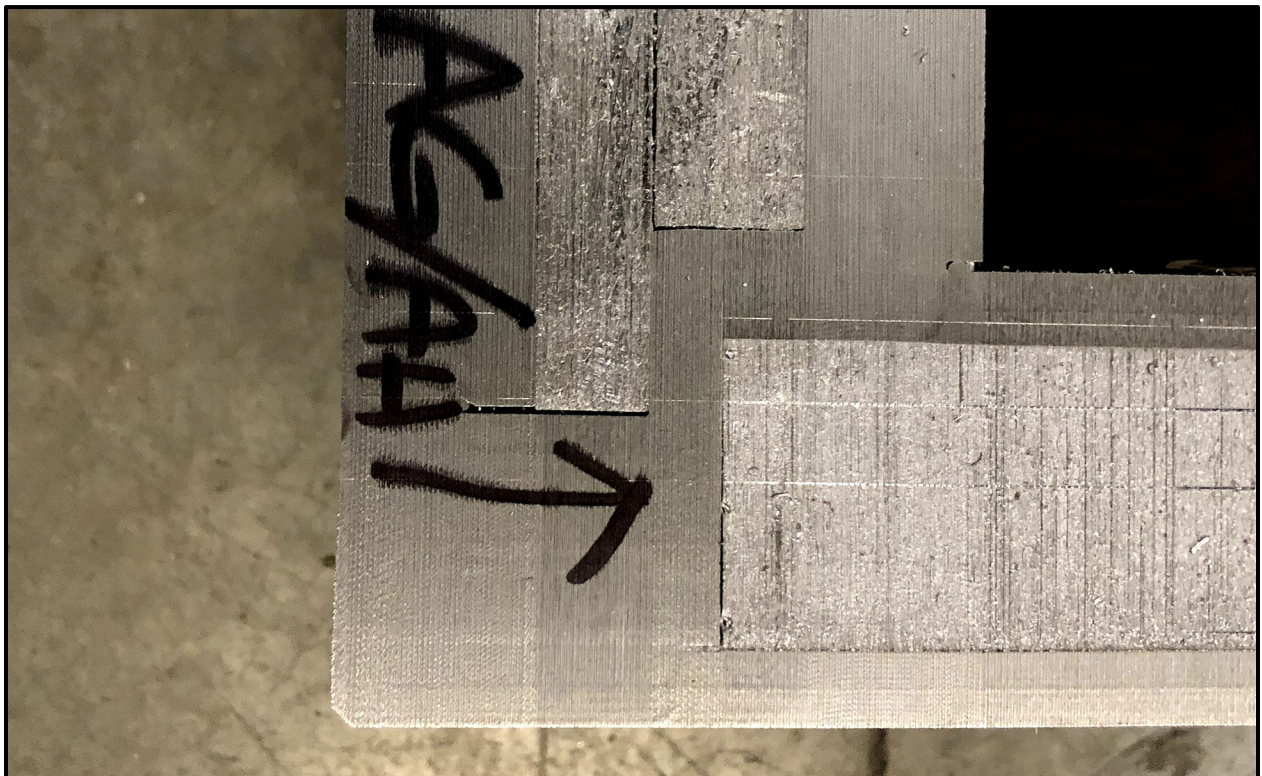
Figure 7-31 – SC-55G2 18TU-09 Destructive Disassembly Cut AG/AH at Lower Flange
