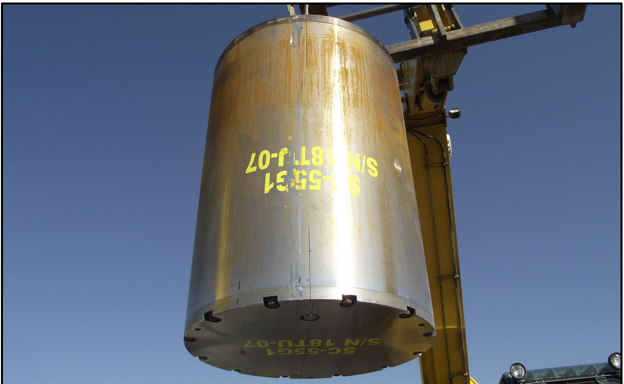
Figure 6-18 – SC-55G1 18TU-07 Superficial Sidewall Damage (Upper in Side Drop)
