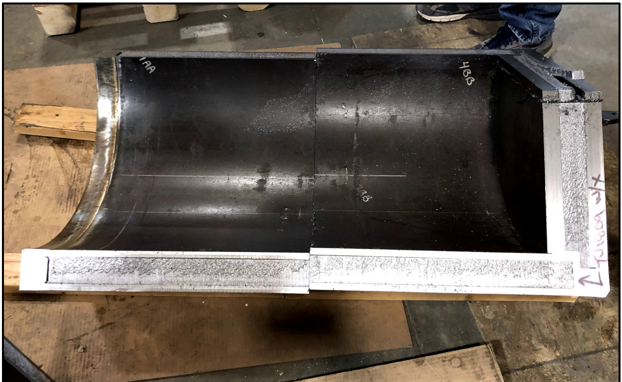
Figure 7-33 – SC-55G2 18TU-09 Destructive Disassembly Cut W/X
