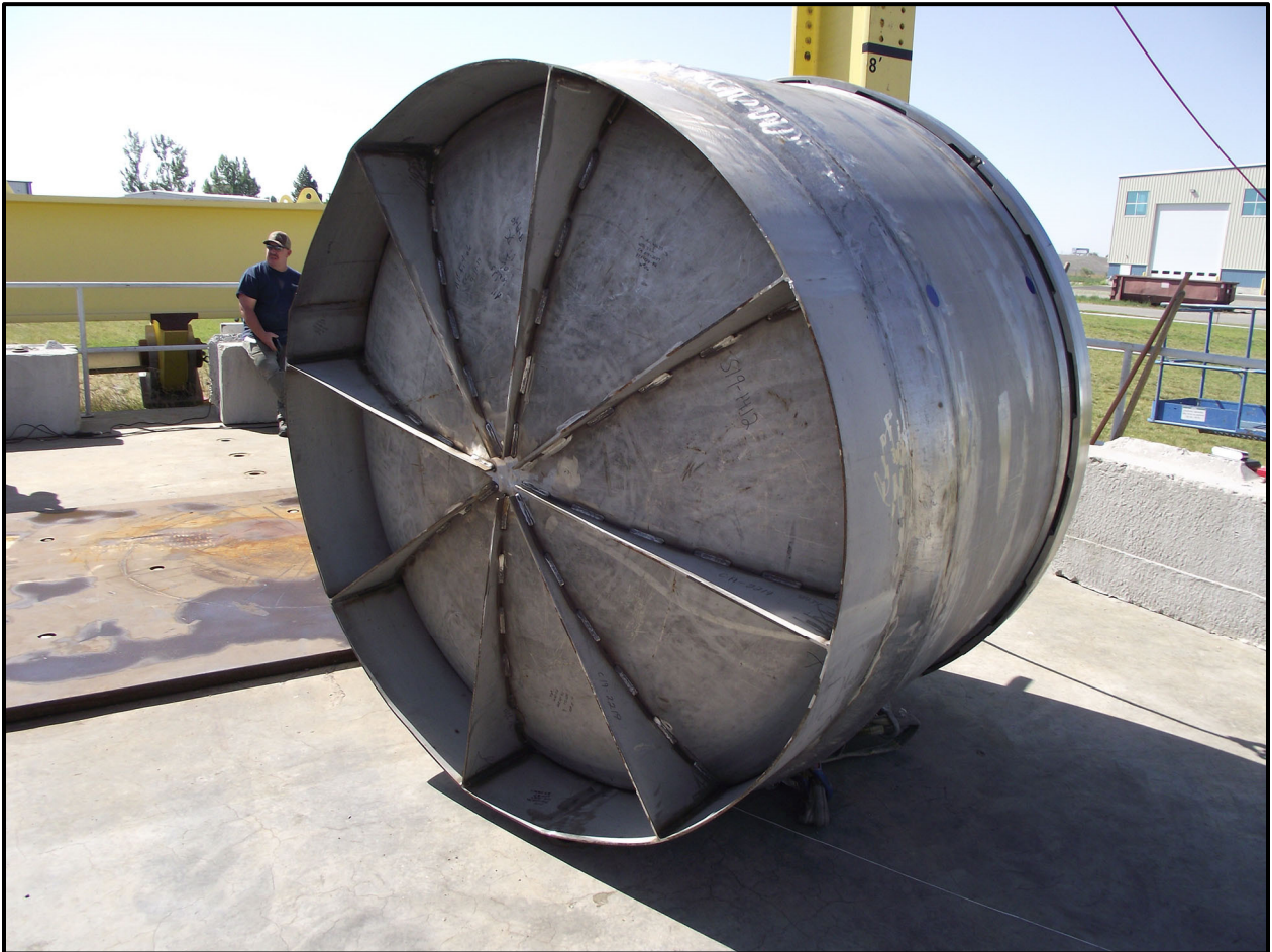
Figure 4-11 – HalfPACT ICV Bottom Reinforcement Configuration
