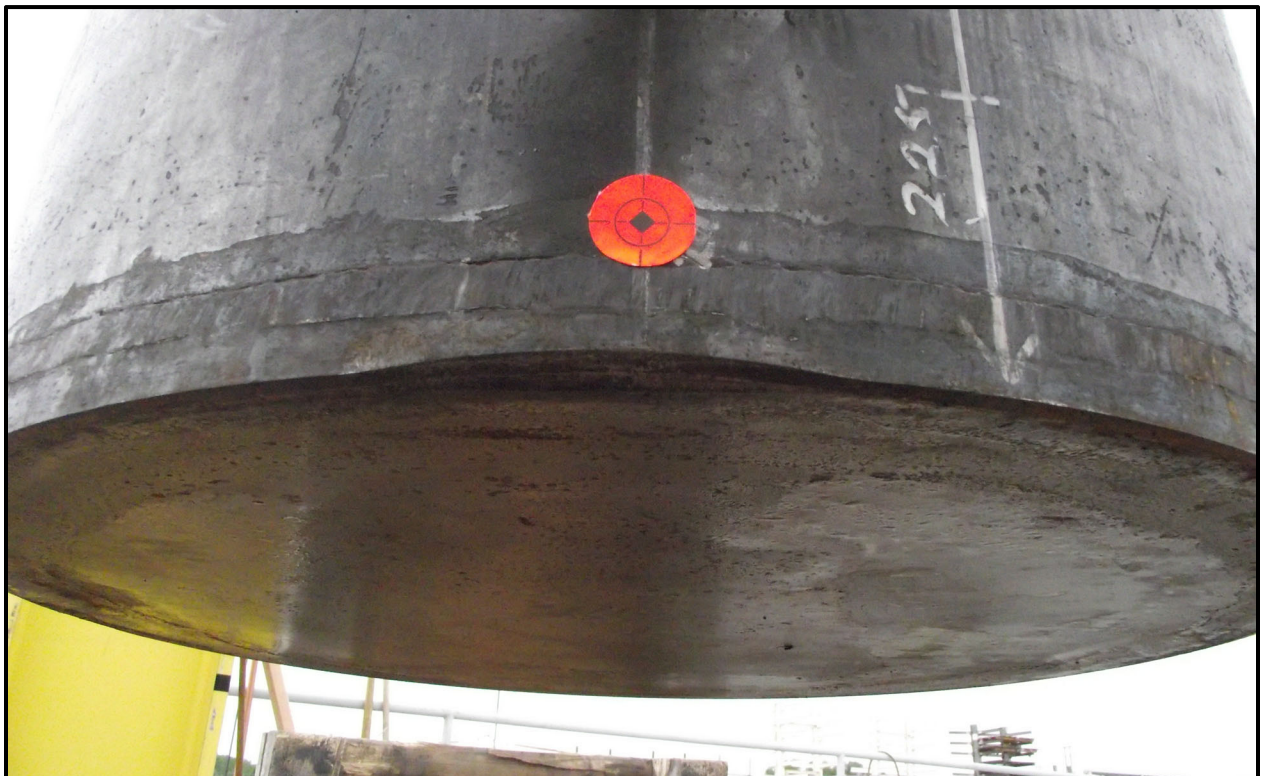
Figure 7-2 – SC-30G2 18TU-01 Vertical End Drop Damage
