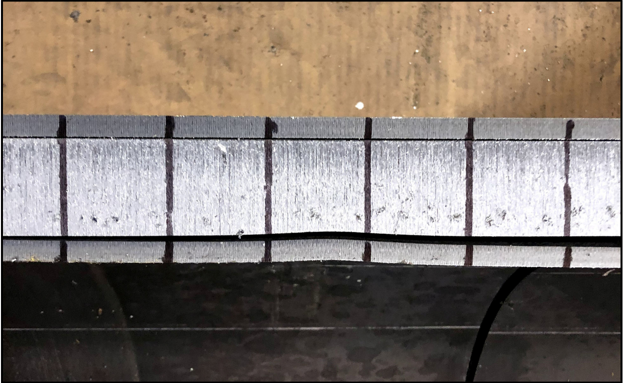
Figure 7-18 – SC-30G2 18TU-02 Destructive Disassembly Cut AT/AU at Axial Elevation 10.5
