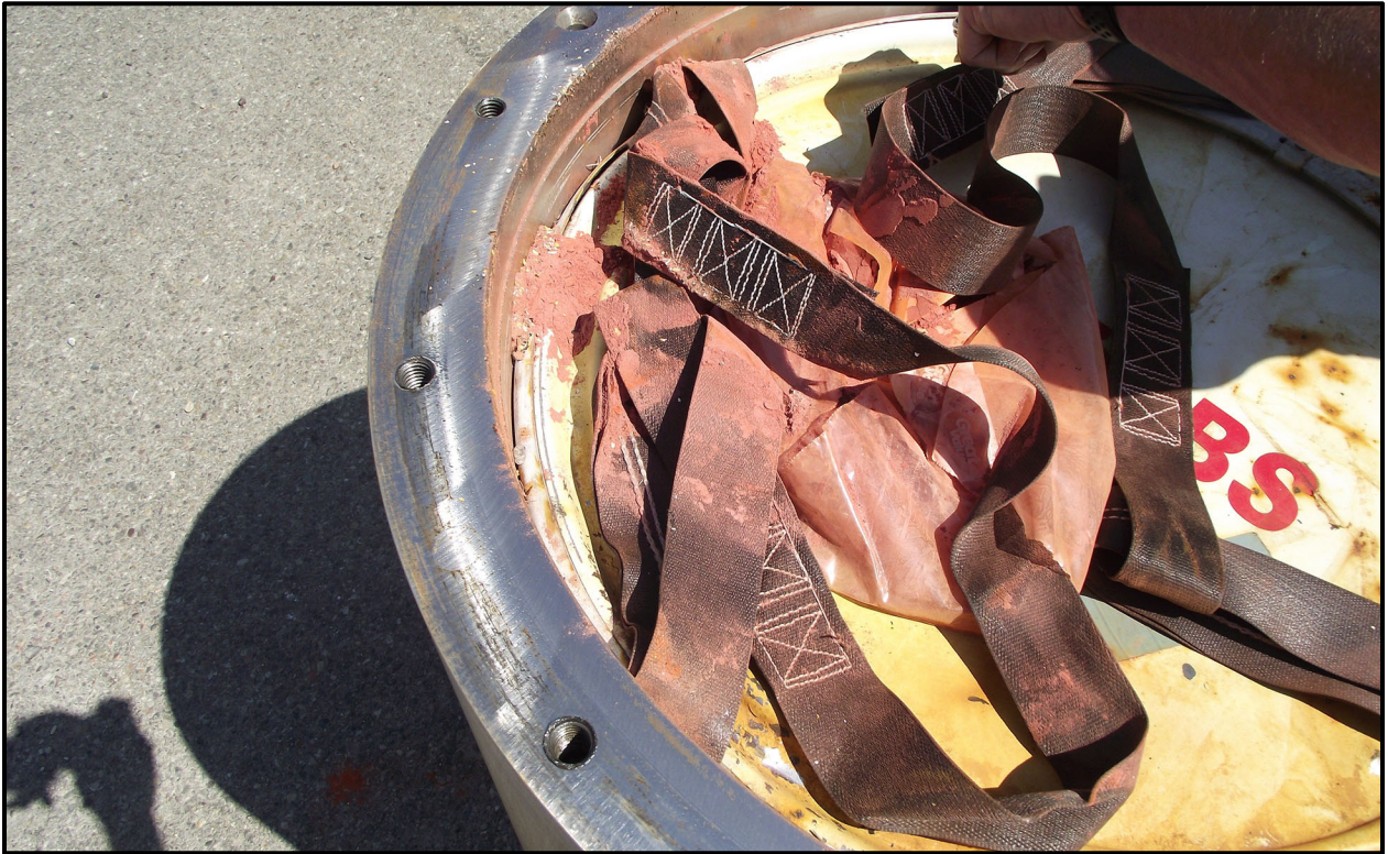
Figure 6-21 – Fluorescein Dye inside the SC-55G1 Body
