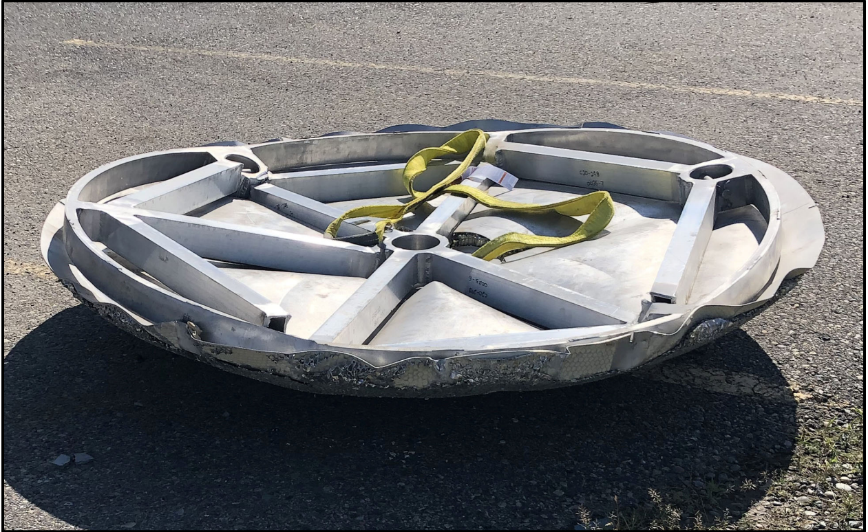
Figure 6-11 – Deformed Heavy-Duty Pallet and Lower Spacer
