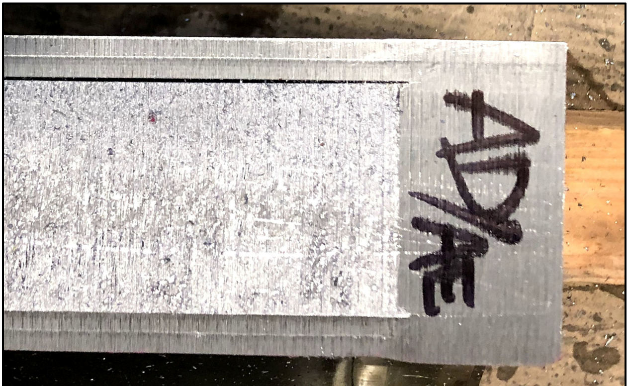
Figure 6-49 – SC-30G3 18TU-04 Destructive Disassembly Cut AD/AE at Upper Flange
