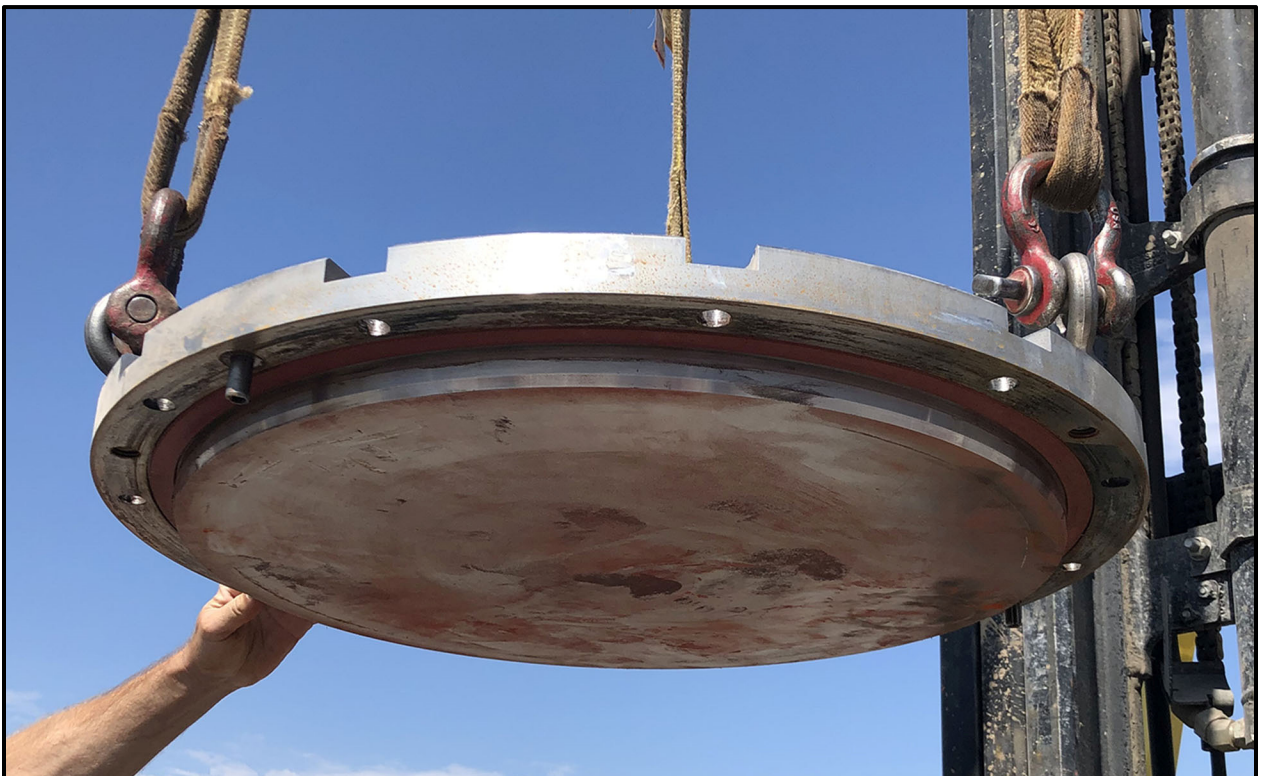
Figure 6-22 – Fluorescein Dye under the SC-55G1 Lid
