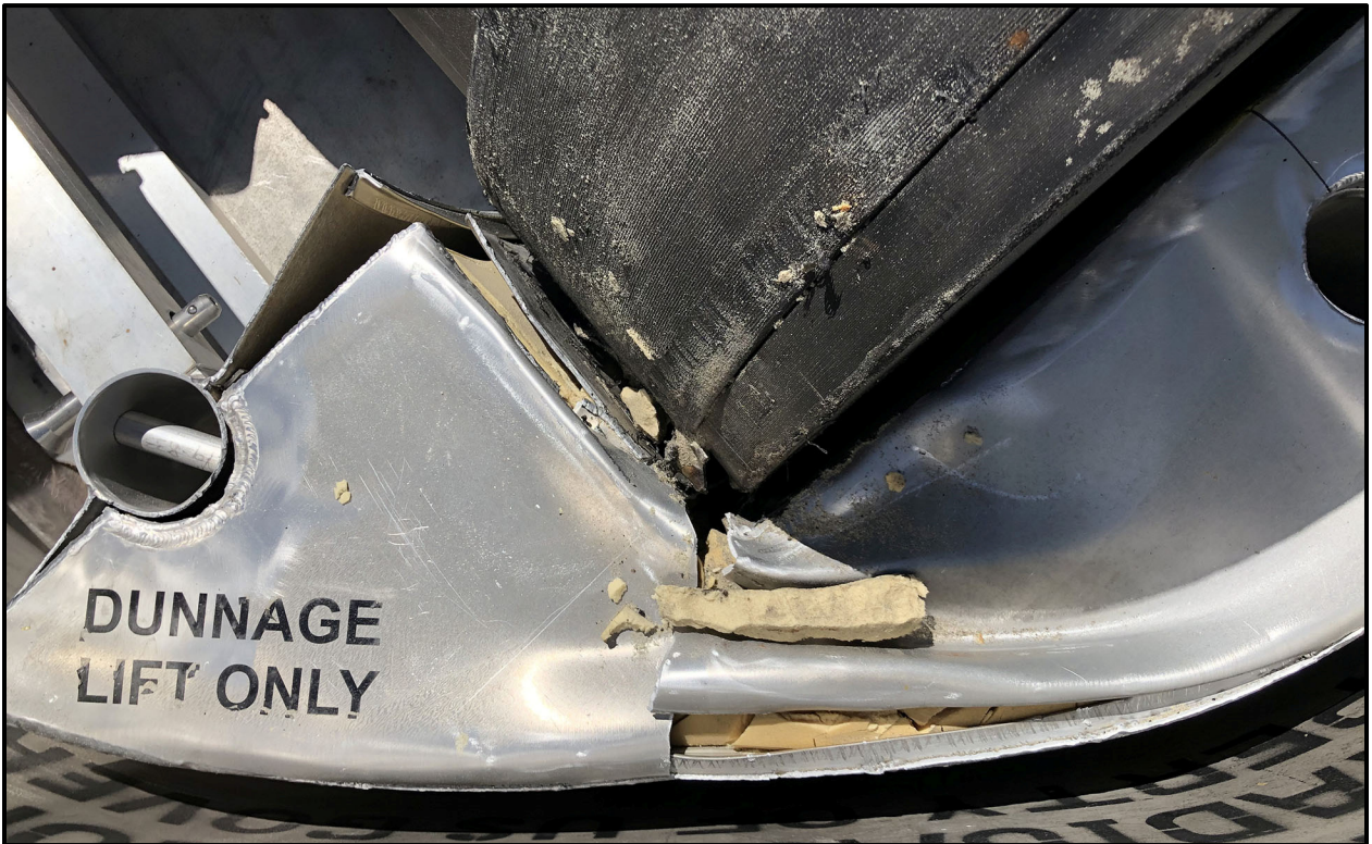
Figure 6-33 – SC-30G3 Lateral Dunnage Side Drop Damage
