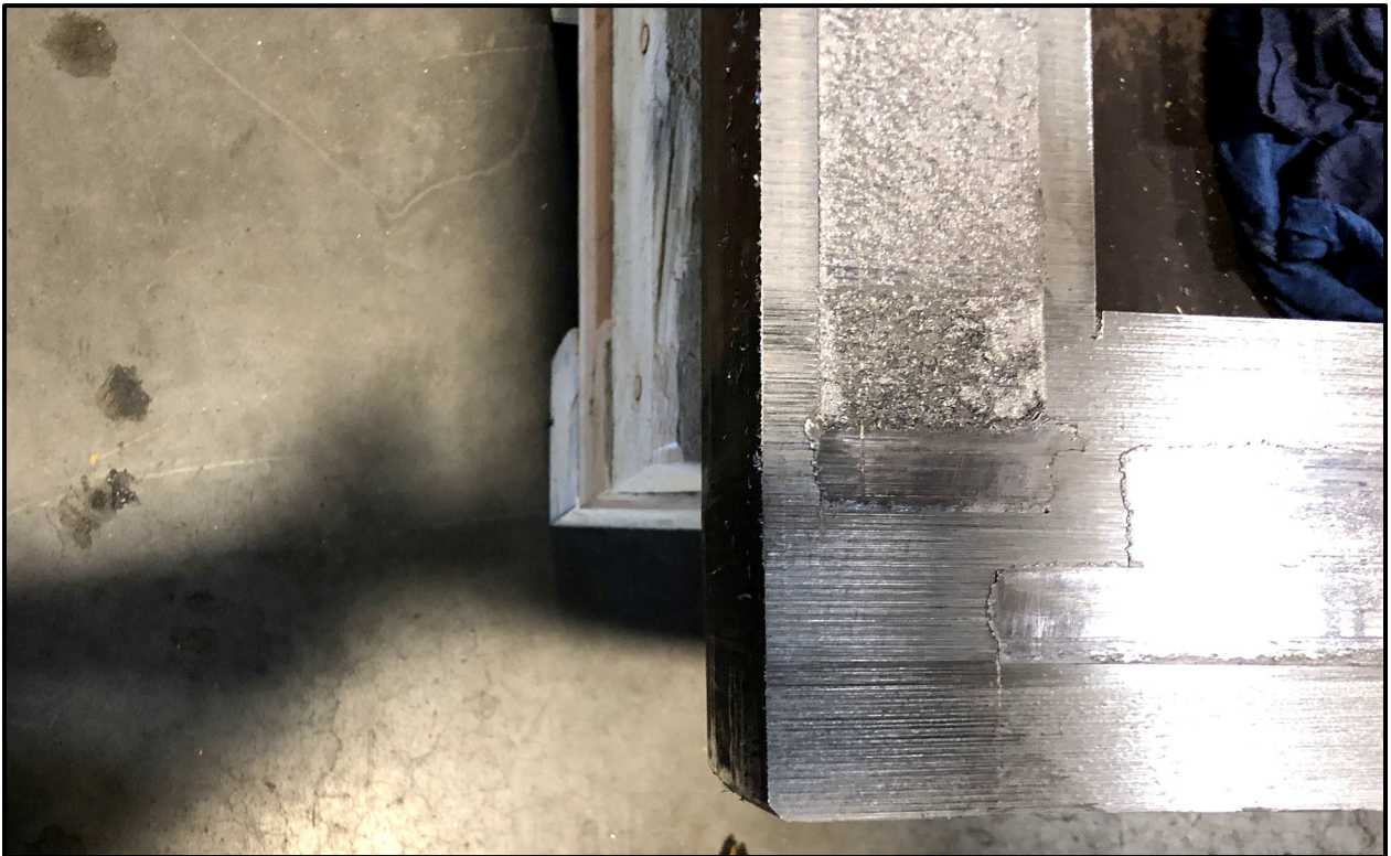
Figure 7-37 – SC-55G2 18TU-10 Destructive Disassembly Cut E/F at Lower Flange
