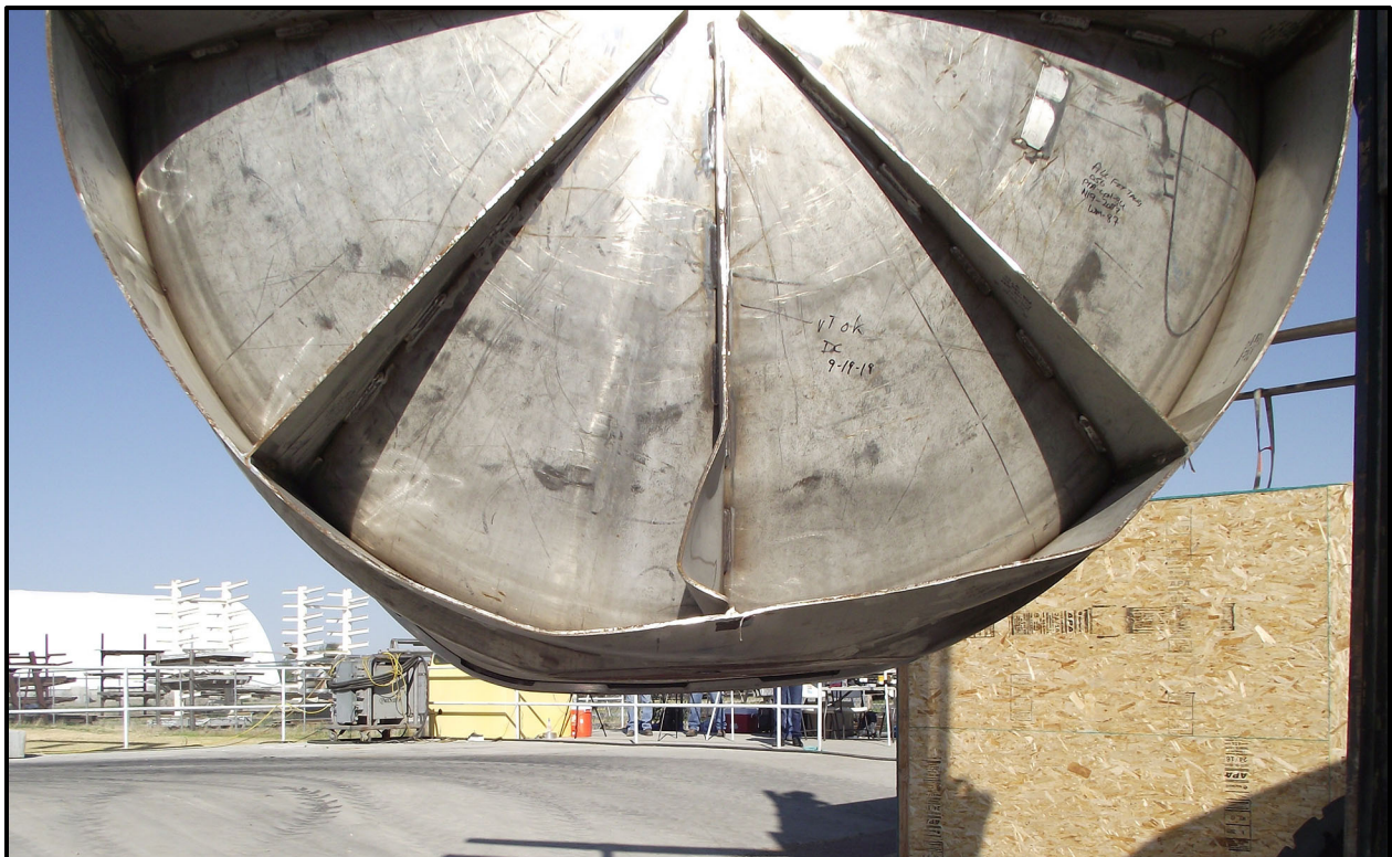
Figure 6-8 – SC-55G1 Side Drop Radial Flattening of the ICV Shell
