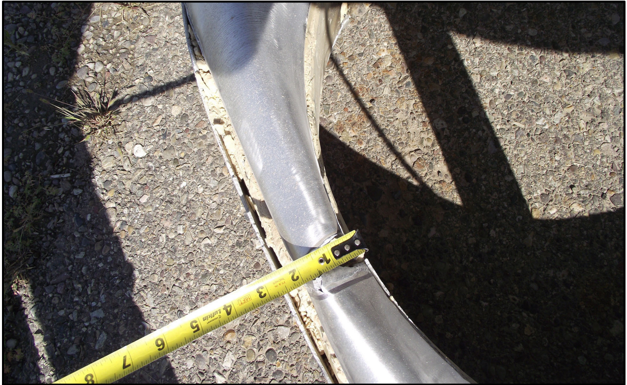
Figure 6-15 – SC-55G1 Radial Dunnage Lower-End Residual Thickness
