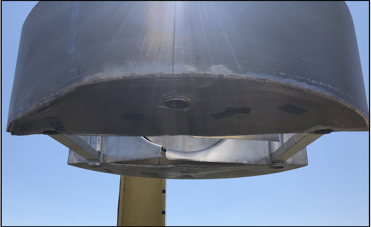
Figure 6-32 – SC-30G3 Lateral Dunnage End Drop Damage
