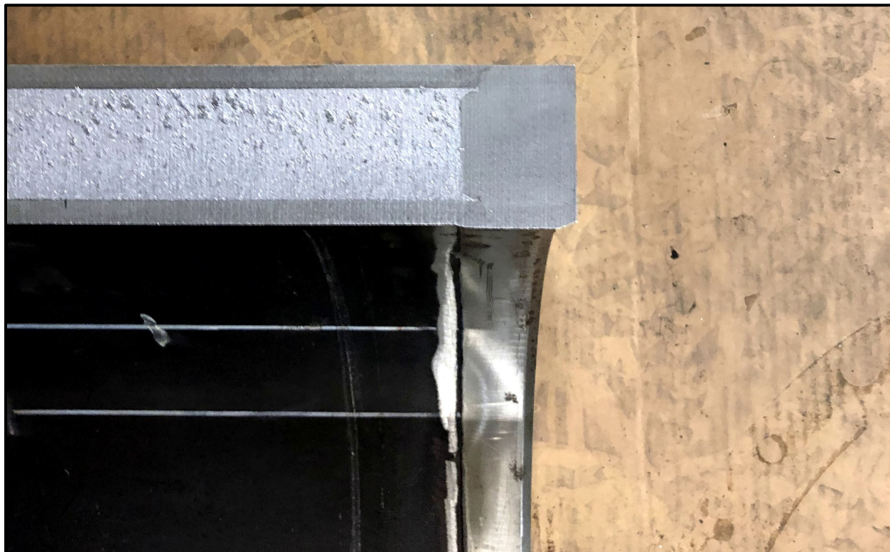
Figure 7-12 – SC-30G2 18TU-01 Destructive Disassembly Cut AA at Upper Flange
