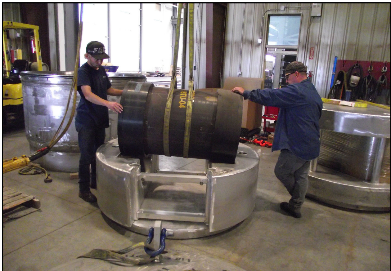
Figure 6-23 – SC-30G3 with End Caps Loaded into Lateral Dunnage
