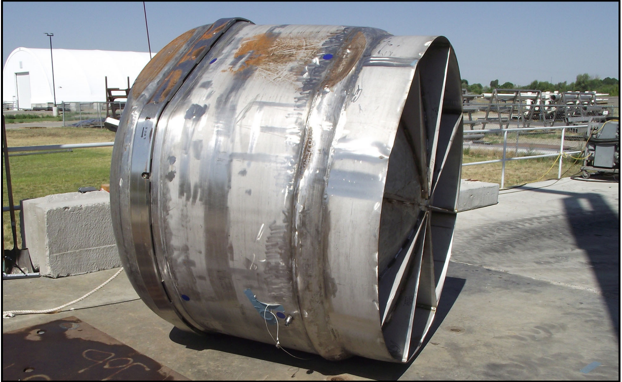
Figure 6-28 – Pre-End Drop Relative Position of the SC-30G3 Lateral Dunnage
