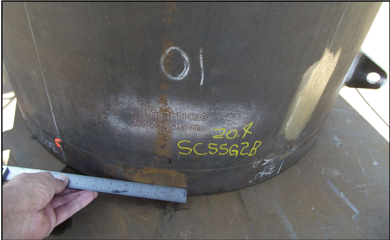
Figure 7-23 – SC-55G2 18TU-10 Horizontal Side Drop Base-End Damage
