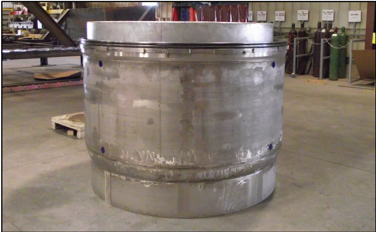
Figure 6-27 – SC-30G3 Side Drop Radial Flattening of the ICV Shell
