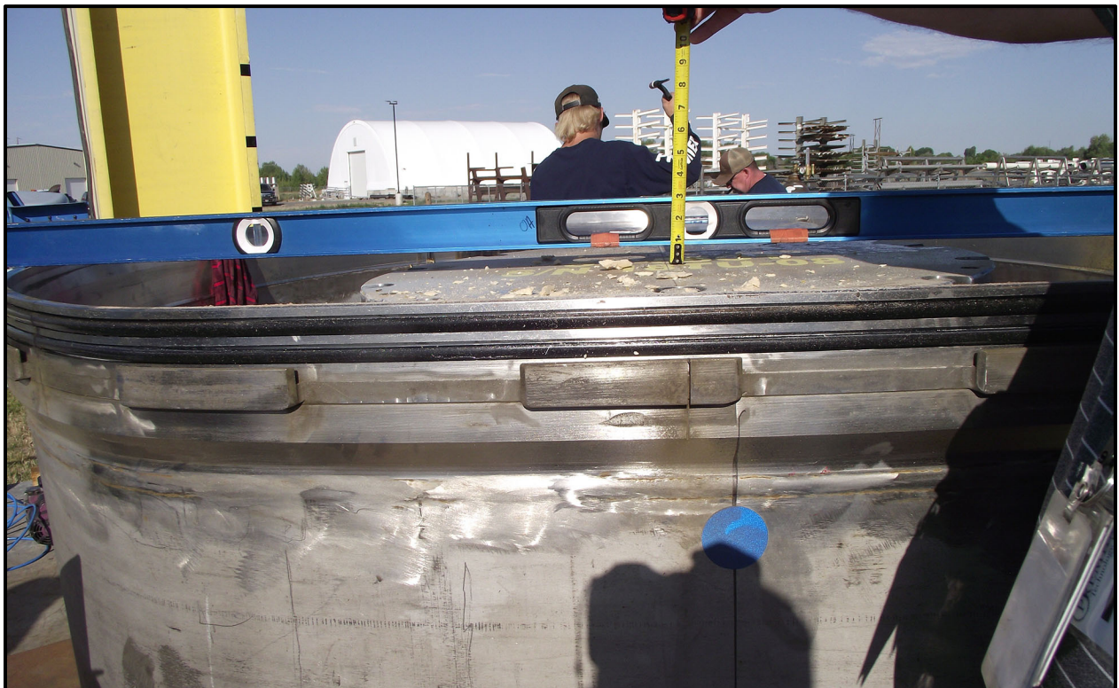
Figure 6-10 – Post-End Drop Relative Position of SC-55G1s
